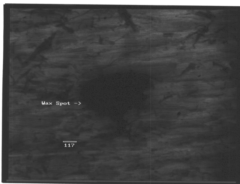
Figure 5 : Wax spots prior to drying at 219°F. (mag = 135x; calibration bar is in \mu\text{m} )
