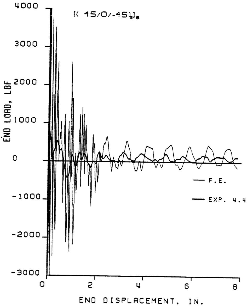
Figure 6.7 Dynamic Load vs. Displacement: Experimental and Finite Element Results for a  $[(45/0/-45)_5]_s$  Laminate
