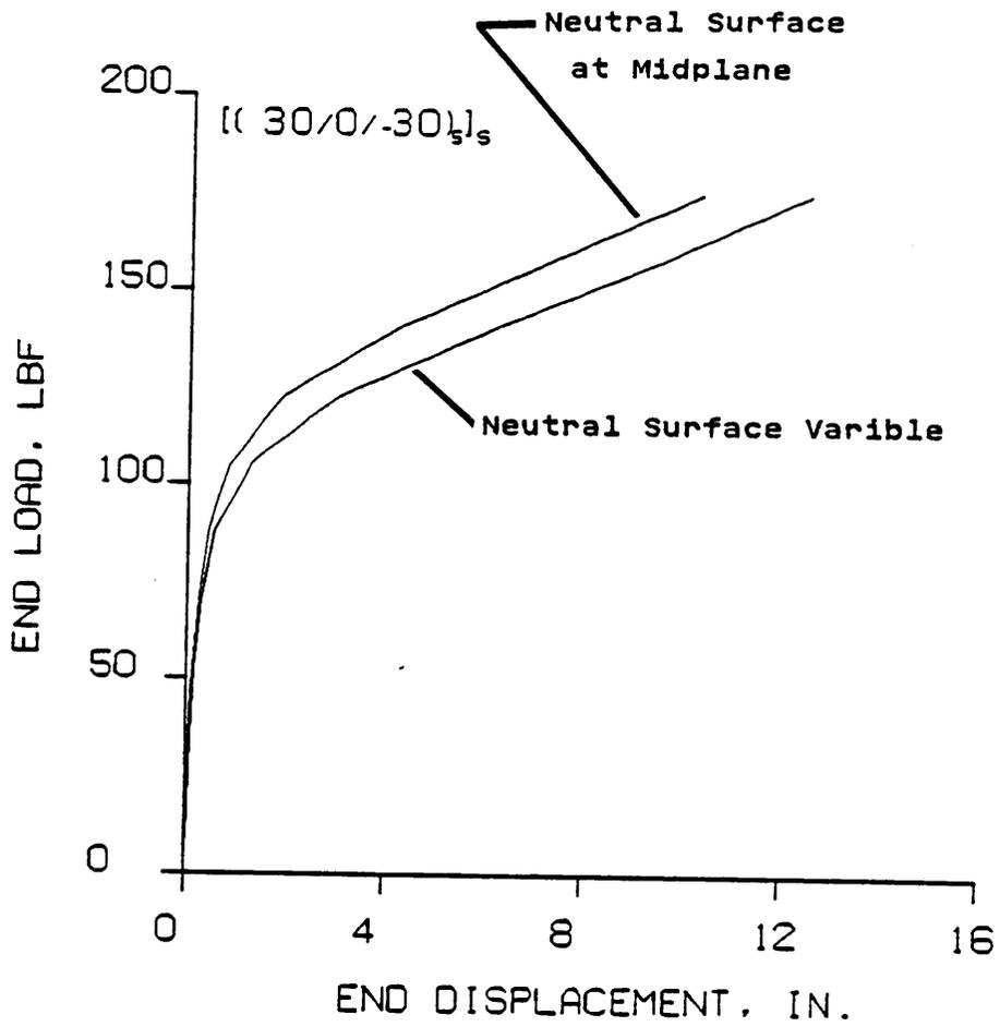
Figure H.1 Effect of Shift in Neutral Surface on the Load-Displacement Relation for the  $[(30/0/-30)_5]_s$  Laminate
