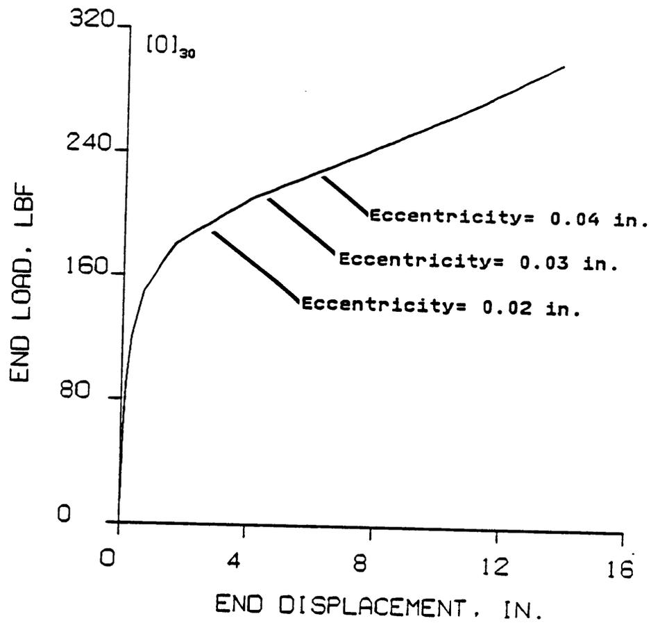
Figure B.1 Effect of Beam Eccentricity on Static Load-Displacement Relation
