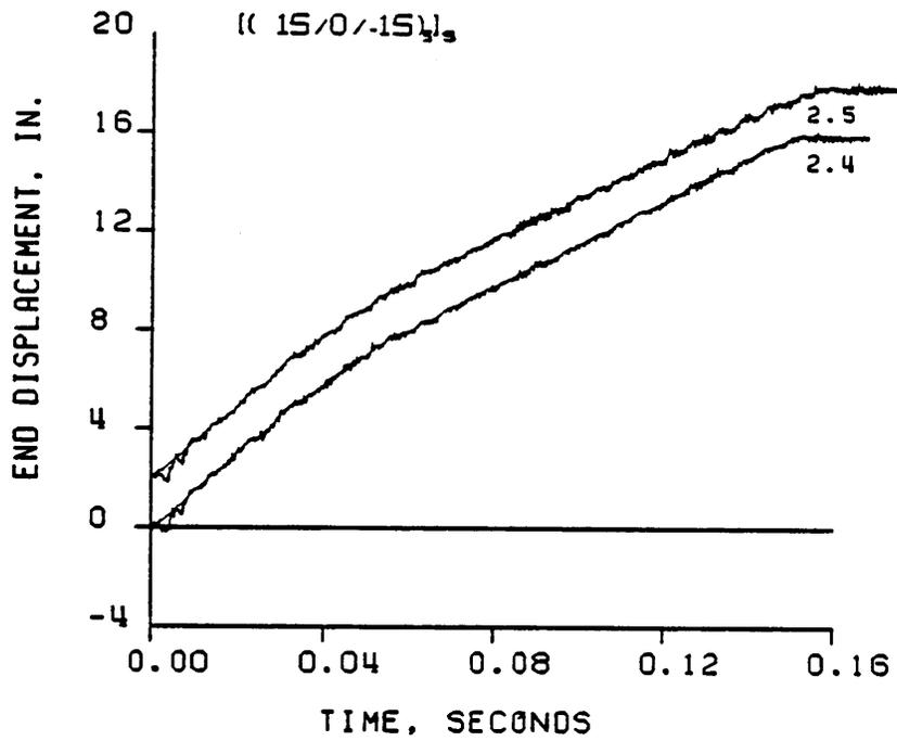
Figure 3.7 Dynamic Displacement vs. Time for the  $[(15/0/-15)_5]_s$  Laminates
