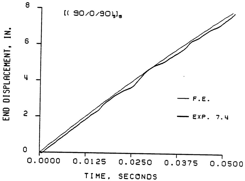
Figure 6.3 Dynamic Displacement vs. Time: Experimental and Finite Element Results for a [(90/0/90)<sub>5</sub>]<sub>s</sub> Laminate
