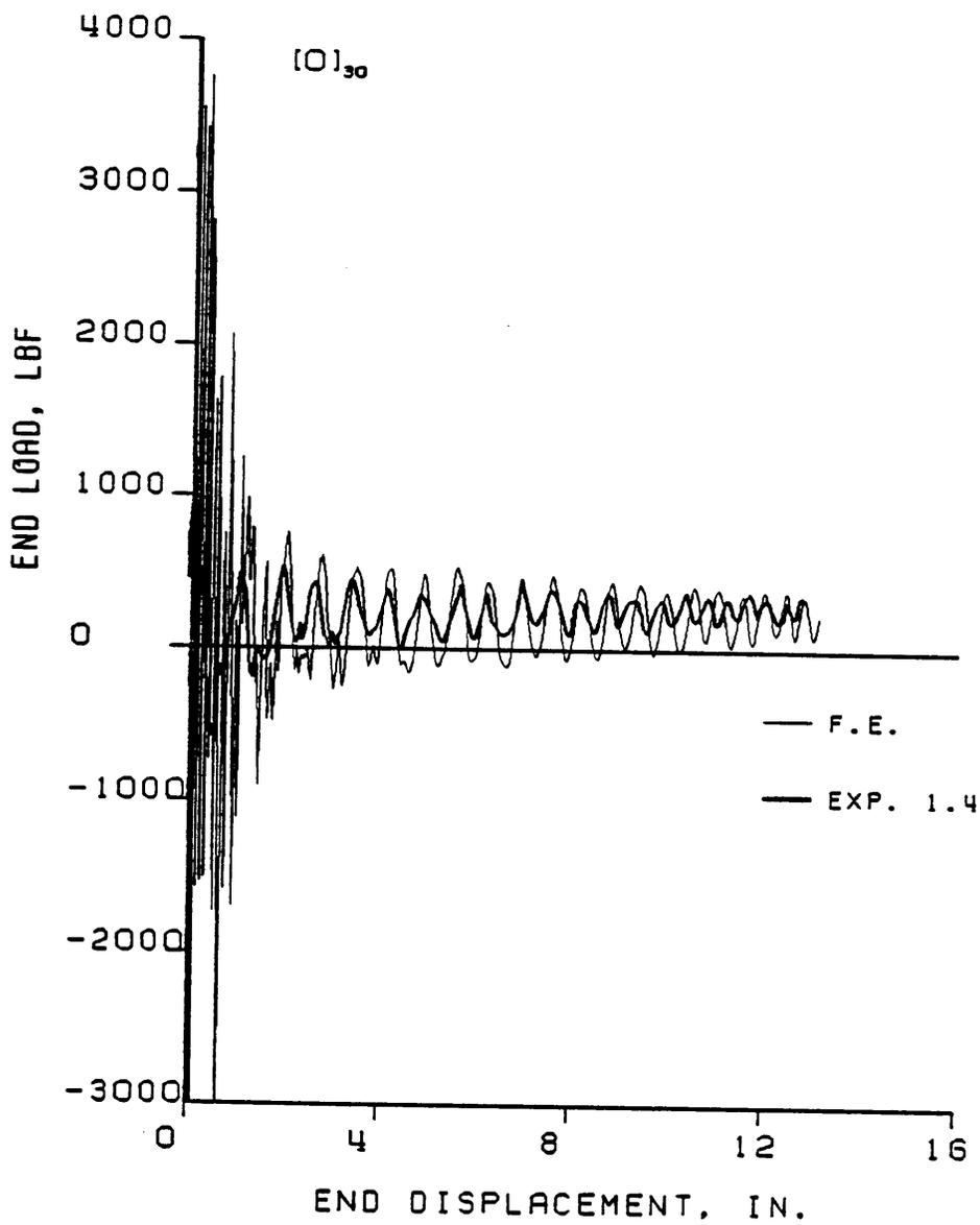
Figure 6.10 Dynamic Load vs. Displacement: Experimental and Finite Element Results for a  $[0]_{30}$  Laminate
