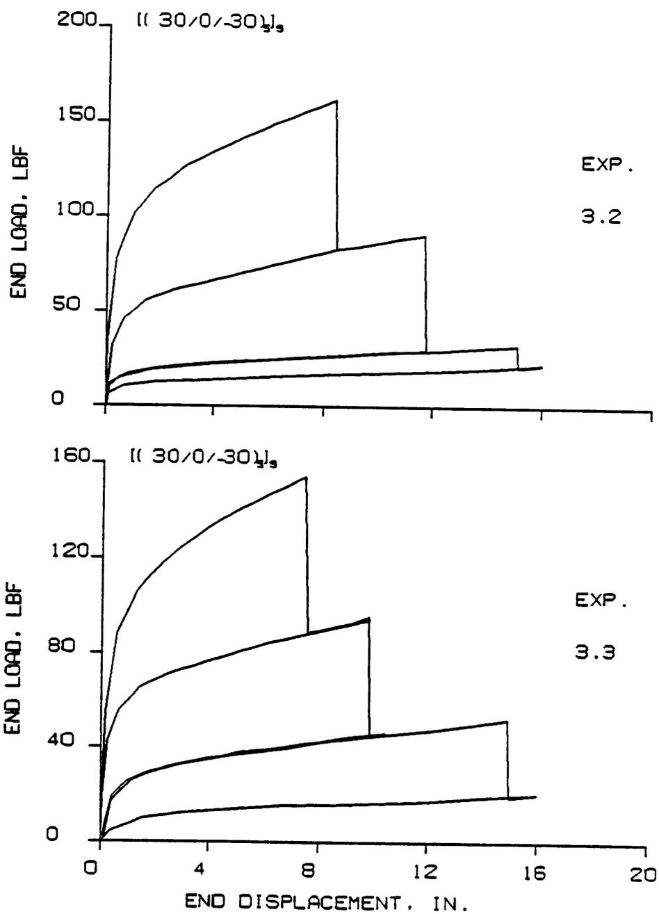
Figure D.4 Static Load-Displacement Relation for Specimens 3.2 and 3.3
