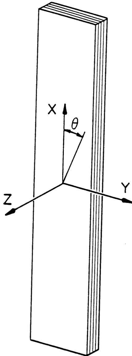
Figure 3.38 Beam Coordinate System
