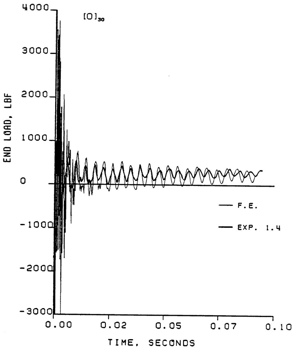
Figure 6.8 Dynamic Load vs. Time: Experimental and Finite Element Results for a  $[0]_{30}$  Laminate
