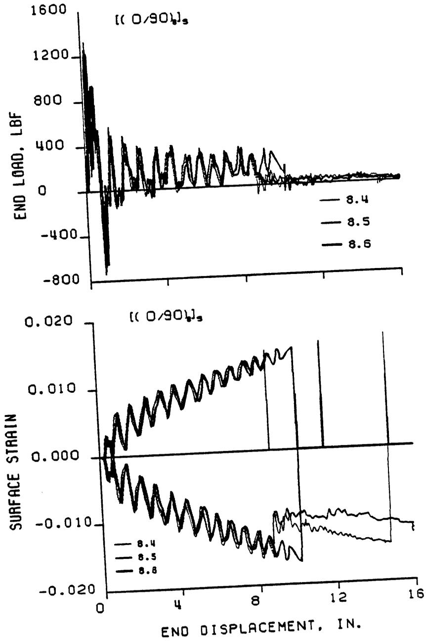
Figure 3.24 Dynamic Load and Strain vs. Displacement for the  $[(0/90)_8]_s$  Laminates
