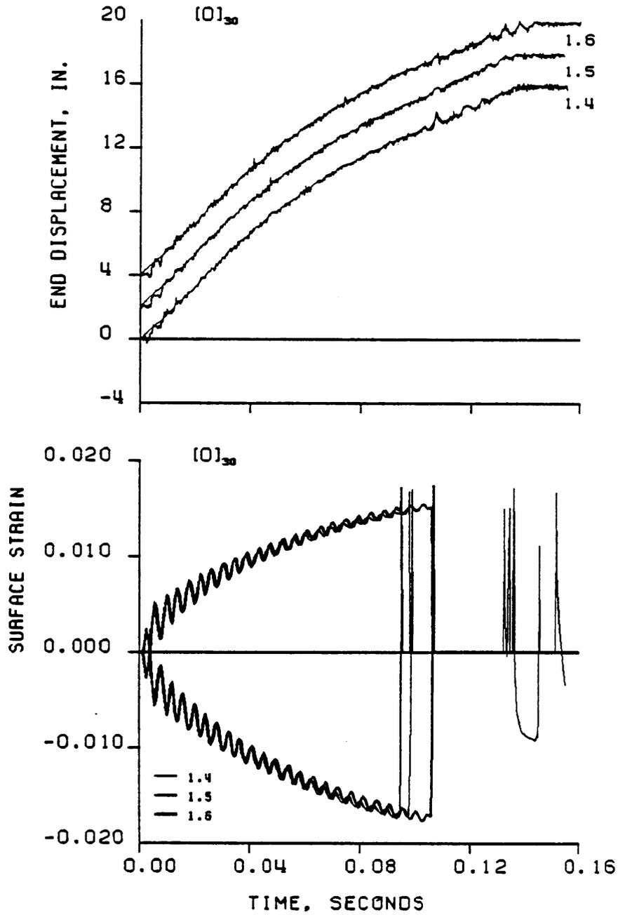
Figure 3.10 Dynamic Displacement and Strain vs. Time for the [0]<sub>30</sub> Laminates
