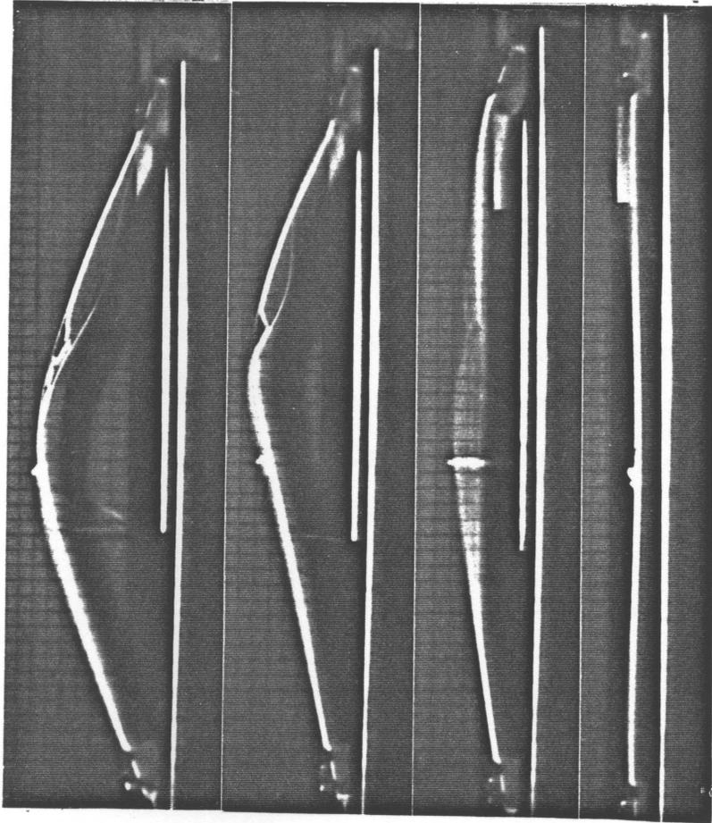
Figure 3.41 Dynamic Failure Mode of  $(0_g/90_g)_s$
