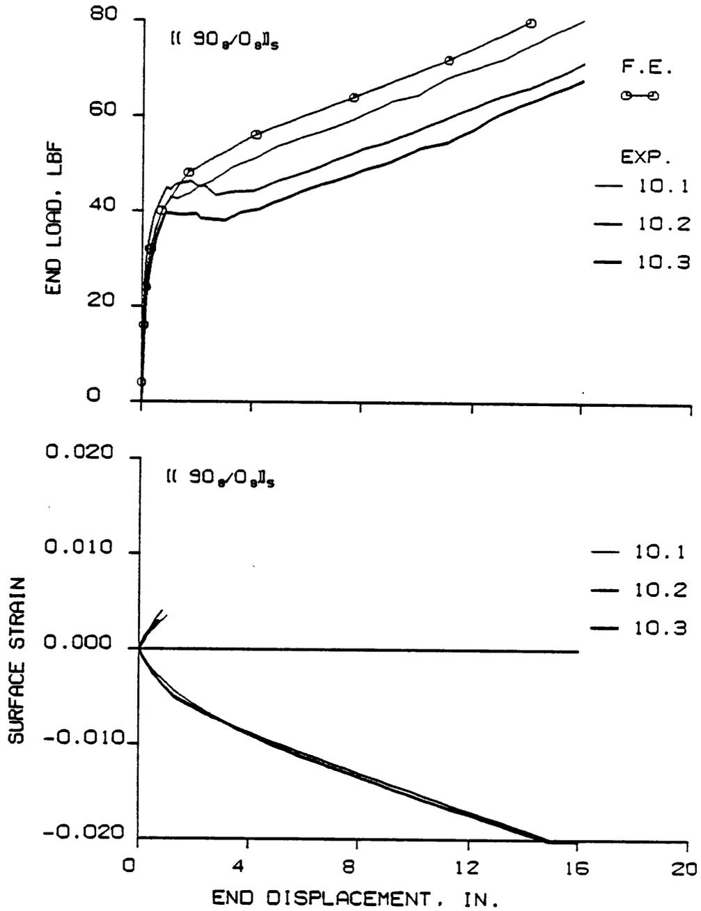
Figure 3.29 Static Load and Strain vs. Displacement for the  $(90_{\theta}/0_{\theta})_s$  Laminates
