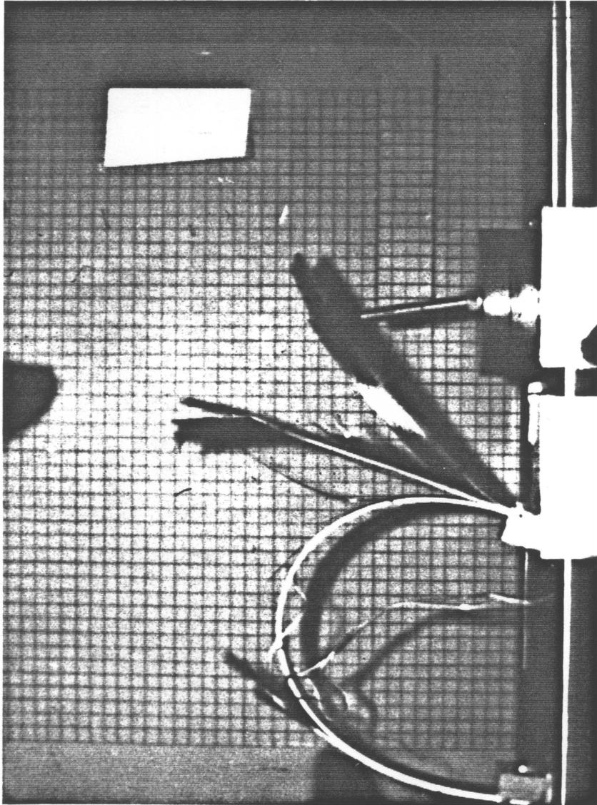
Figure 3.42 Failure Mode of  $[(0/45/0/-45)_3/90/0/1/2]_s$
