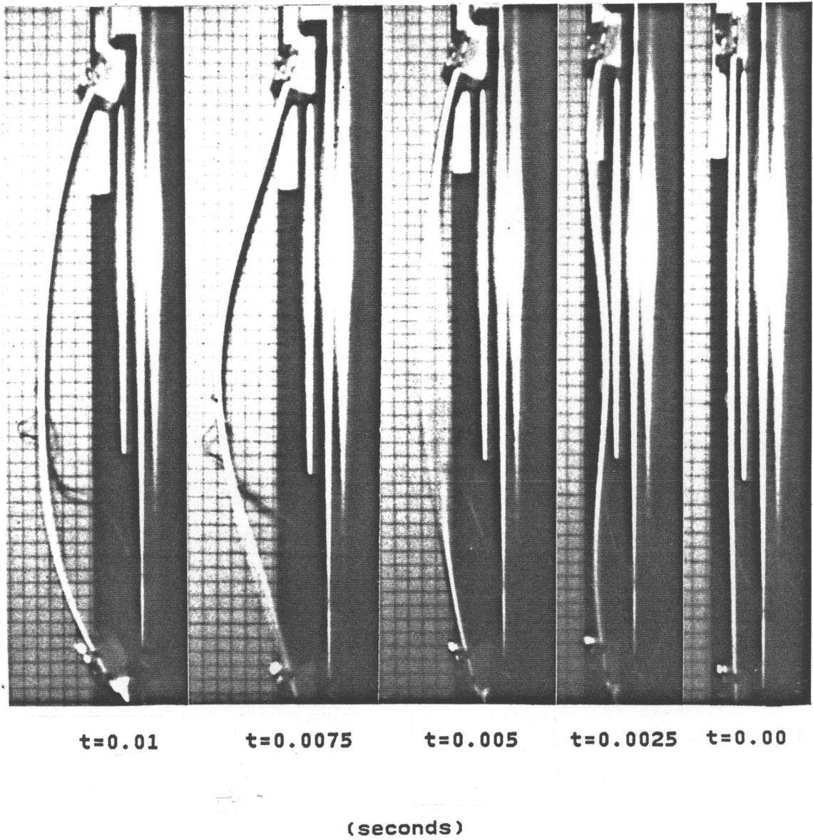
Figure 3.4 Third Mode Deformation Response
