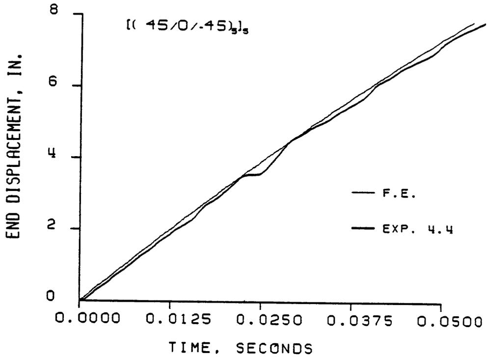
Figure 6.6 Dynamic Displacement vs. Time: Experimental and Finite Element Results for a [(45/0/-45)<sub>5</sub>]<sub>s</sub> Laminate
