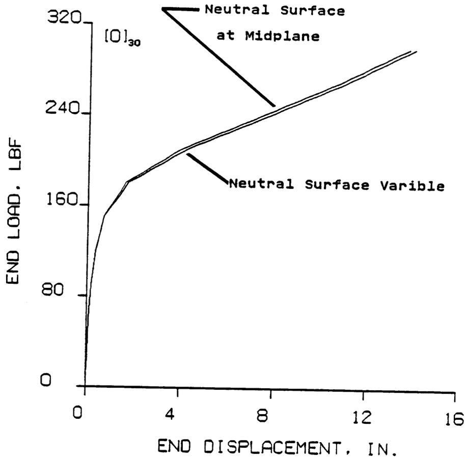
Figure H.2 Effect of Shift in Neutral Surface on the Load-Displacement Relation for the  $[0]_{30}$  Laminate
