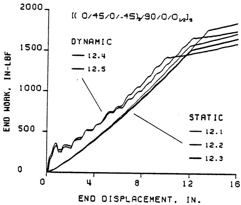
Figure 3.48 End Load Work vs. Displacement for the [(0/45/0/-45)<sub>3</sub>/90/0/0]<sub>1/2</sub><sub>s</sub> Laminates
