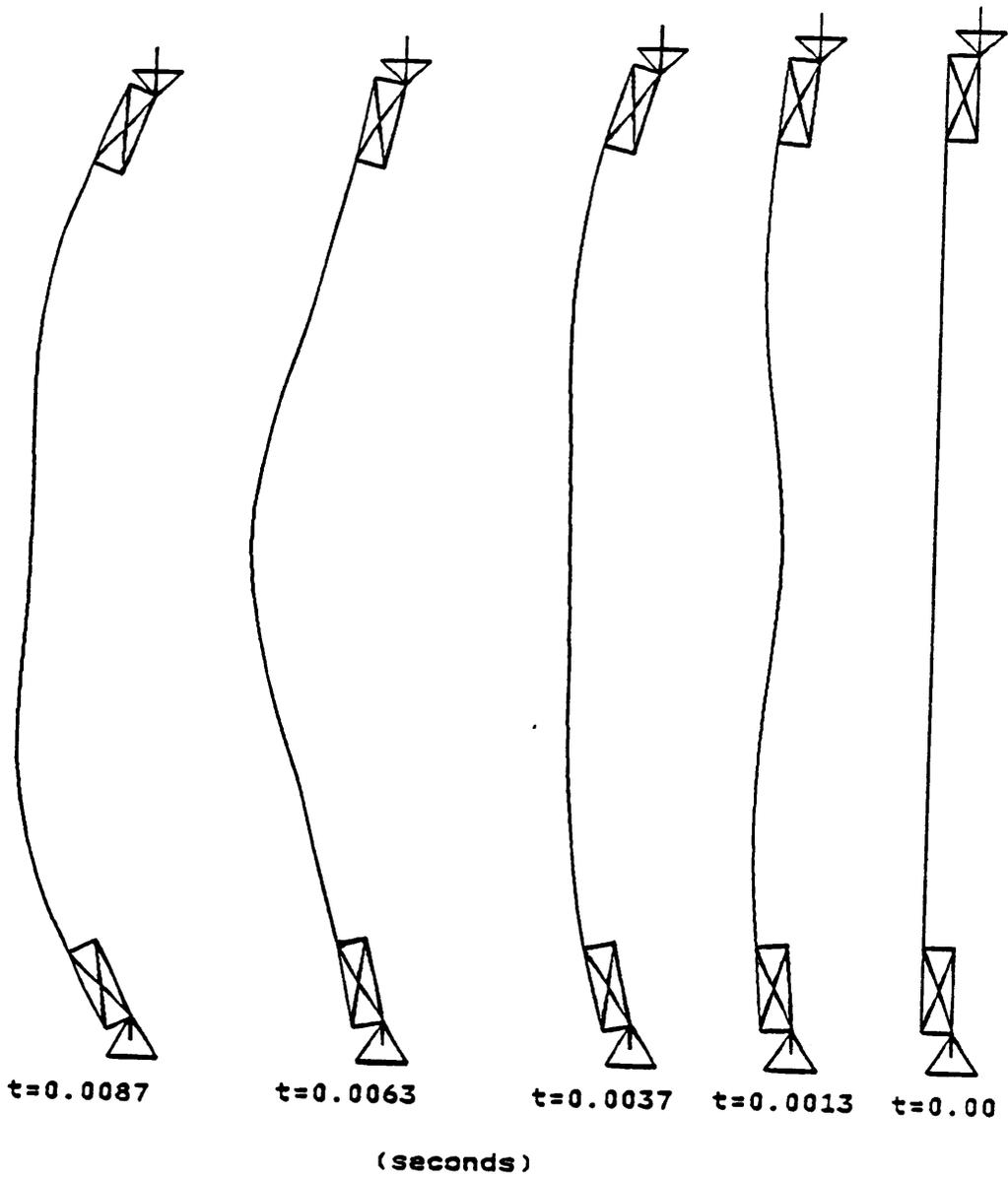
Figure 6.11 Spatial Shapes of a  $[(45/0/-45)_5]_S$  Laminate Under Dynamic Loading
