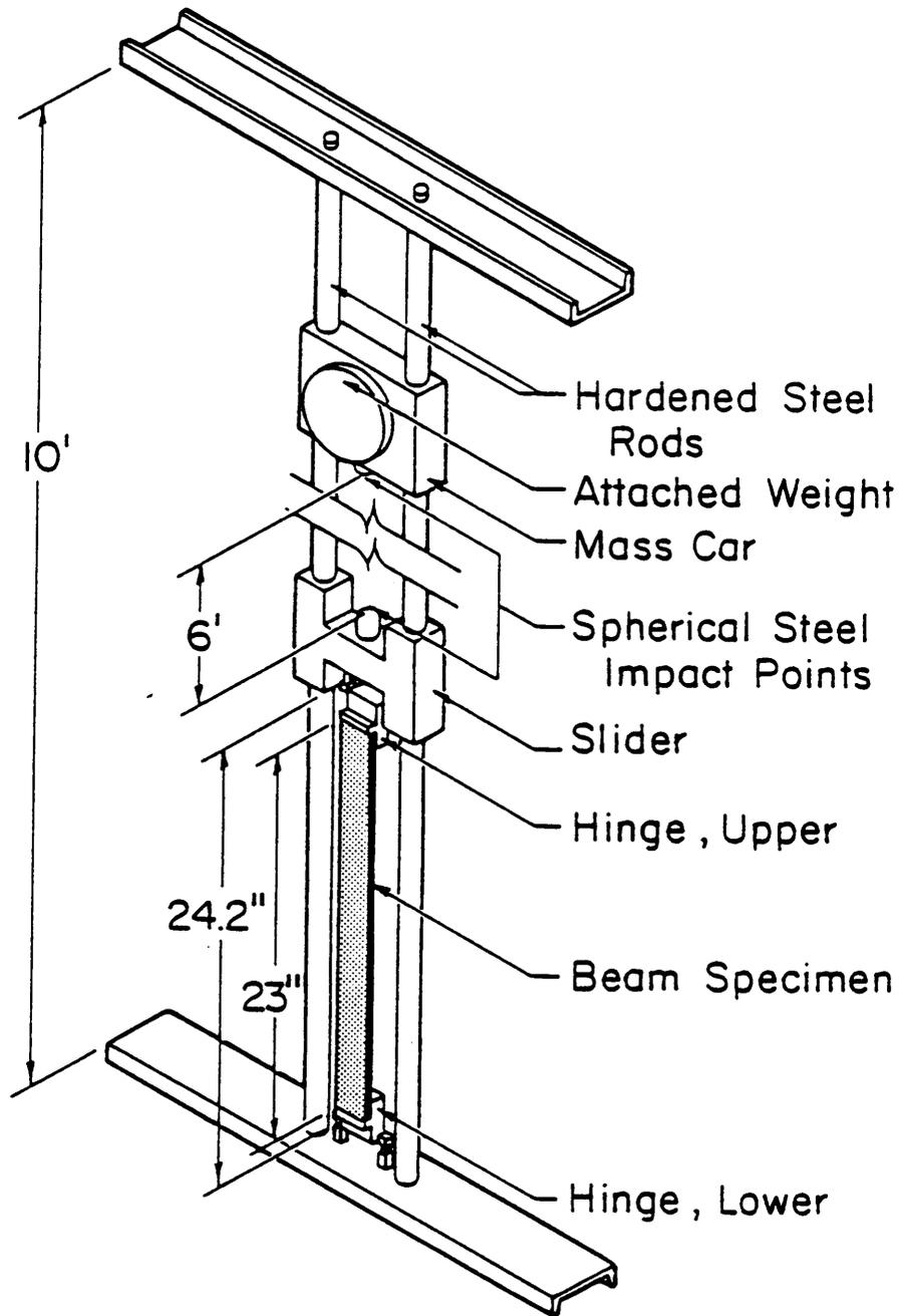
Figure 2.3 Schematic of Drop Tower
