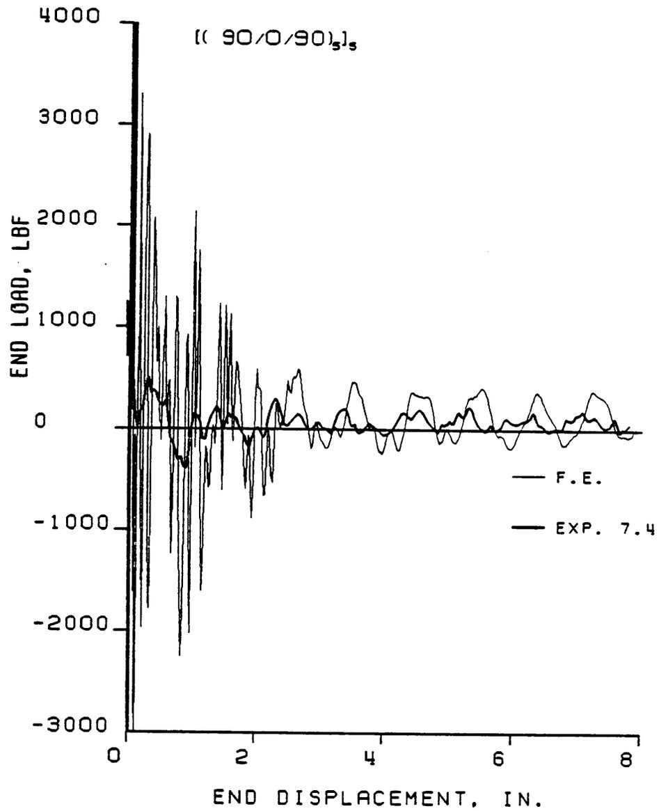
Figure 6.4 Dynamic Load vs. Displacement: Experimental and Finite Element Results for a [(90/0/90)<sub>5</sub>]<sub>s</sub> Laminate
