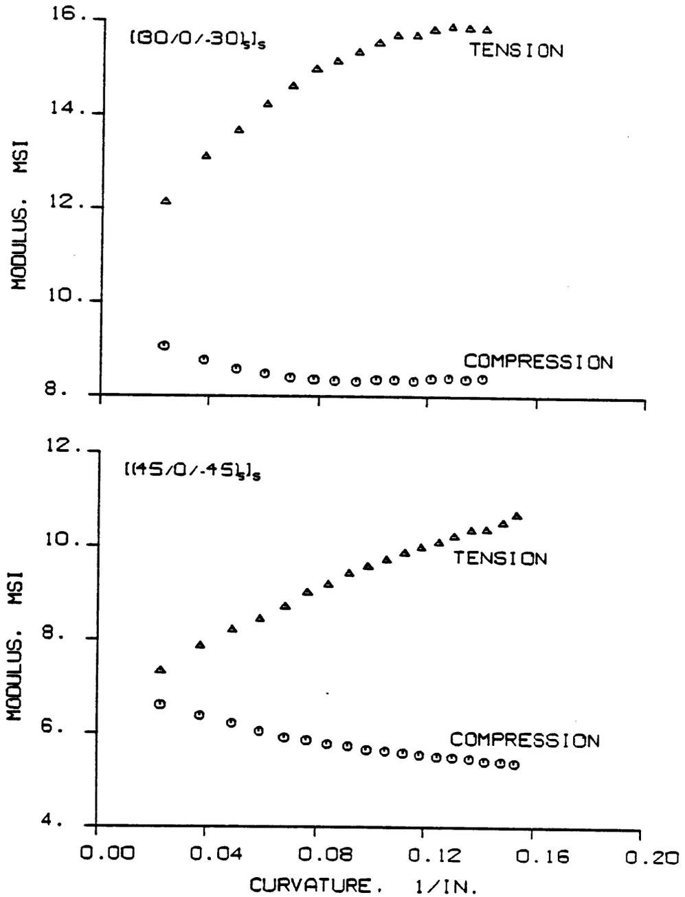
Figure 4.3 Moduli vs. Curvature for the  $[(30/0/-30)_5]_s$  and  $[(45/0/-45)_5]_s$  Laminates
