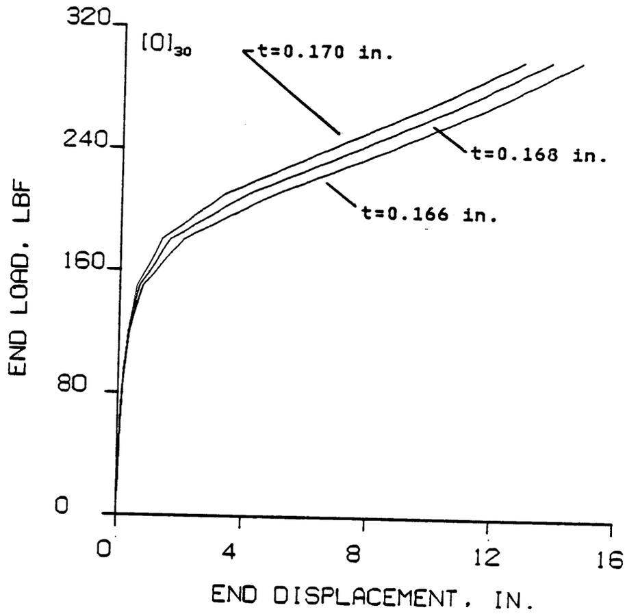
Figure A.1 Effect of Beam Thickness on Static Load-Displacement Relation
