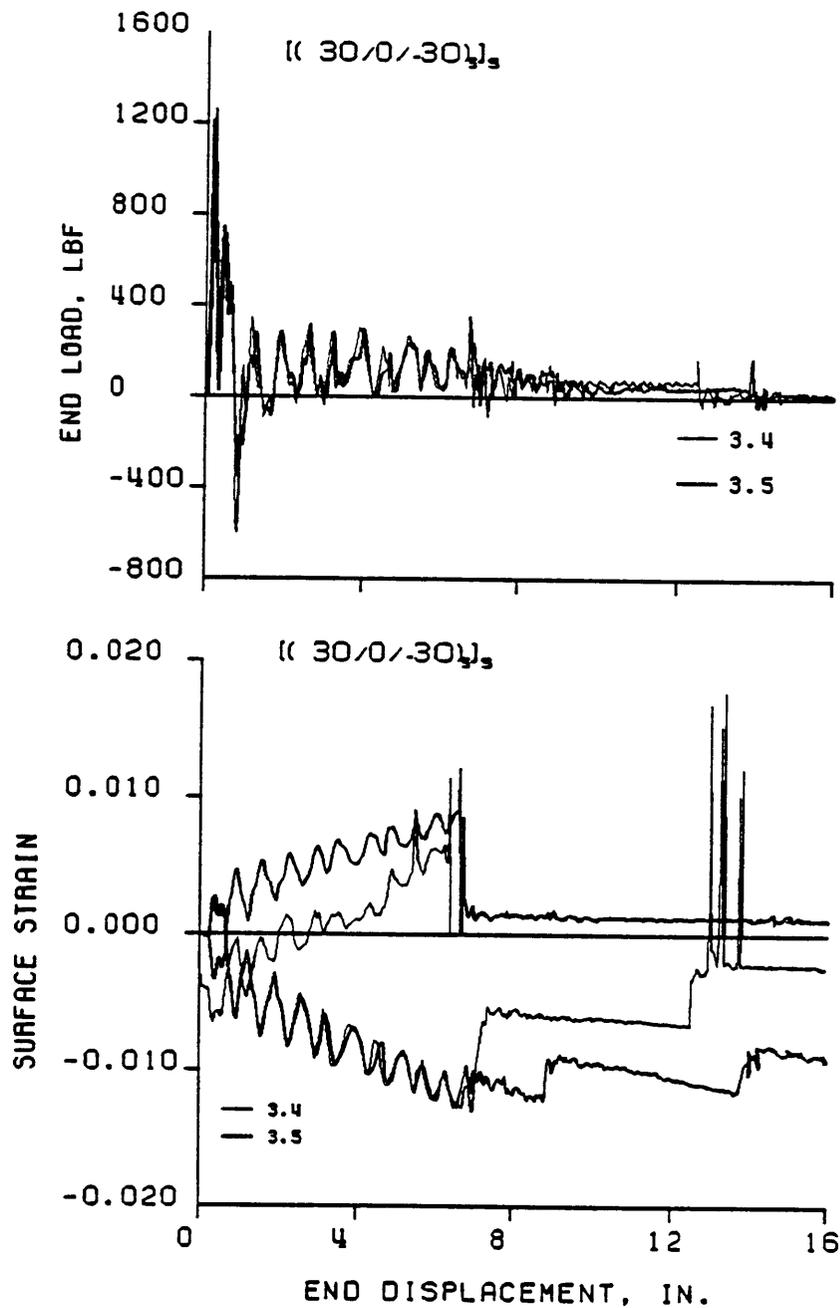
Figure 3.12 Dynamic Load and Strain vs. Displacement for the [(30/0/-30)<sub>5</sub>]<sub>s</sub> Laminates
