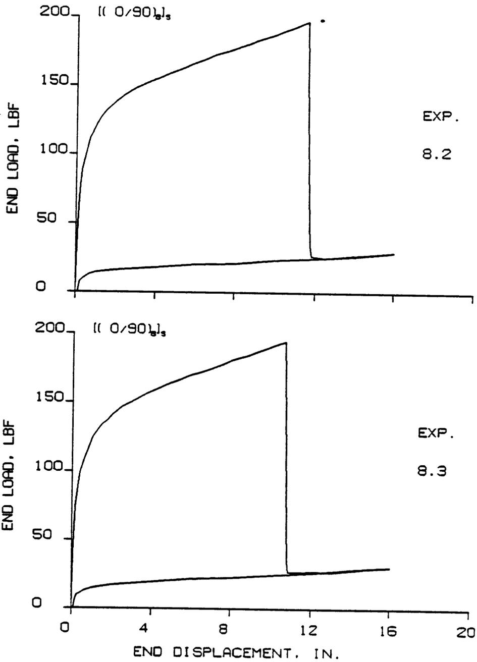
Figure 0.10 Static Load-Displacement Relation for Specimens 8.2 and 8.3
