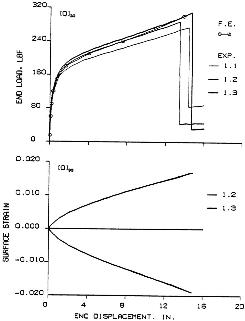
Figure 3.8 Static Load and Strain vs. Displacement for the  $[0]_{30}$  Laminates
