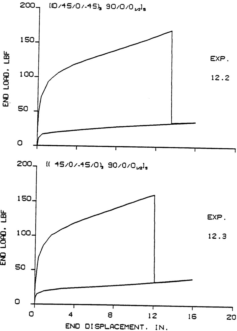
Figure 0.16 Static Load-Displacement Relation for Specimens 12.2 and 12.3
