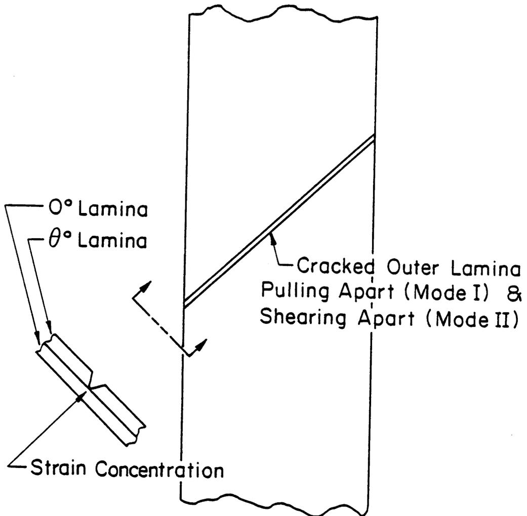
Figure 5.1 Strain Concentration Near Matrix Crack
