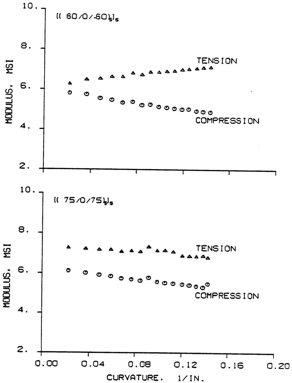
Figure 4.4 Moduli vs. Curvature for the  $[(60/0/-60)_5]_s$  and  $[(75/0/-75)_5]_s$  Laminates
