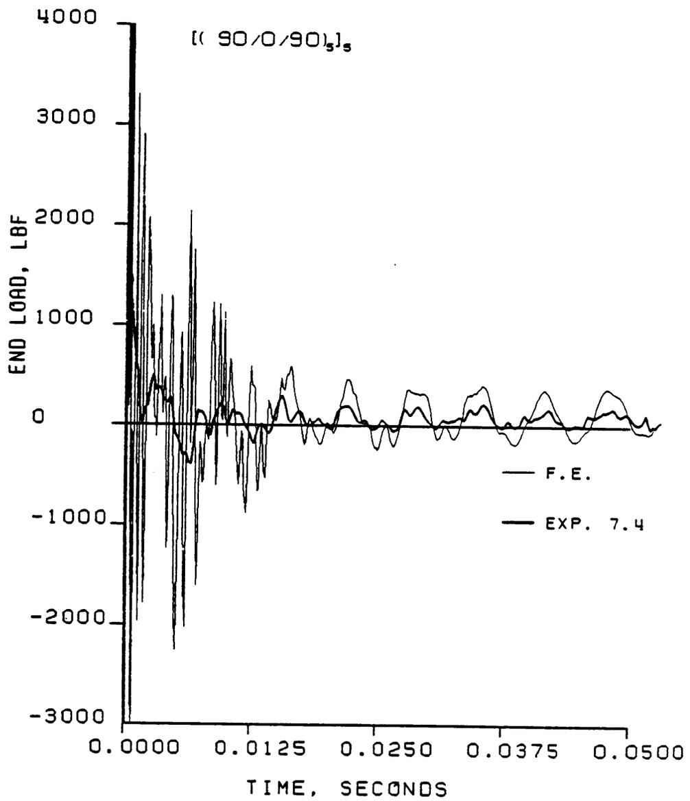
Figure 6.2 Dynamic Load vs. Time: Experimental and Finite Element Results for a  $[(90/0/90)_5]_S$  Laminate
