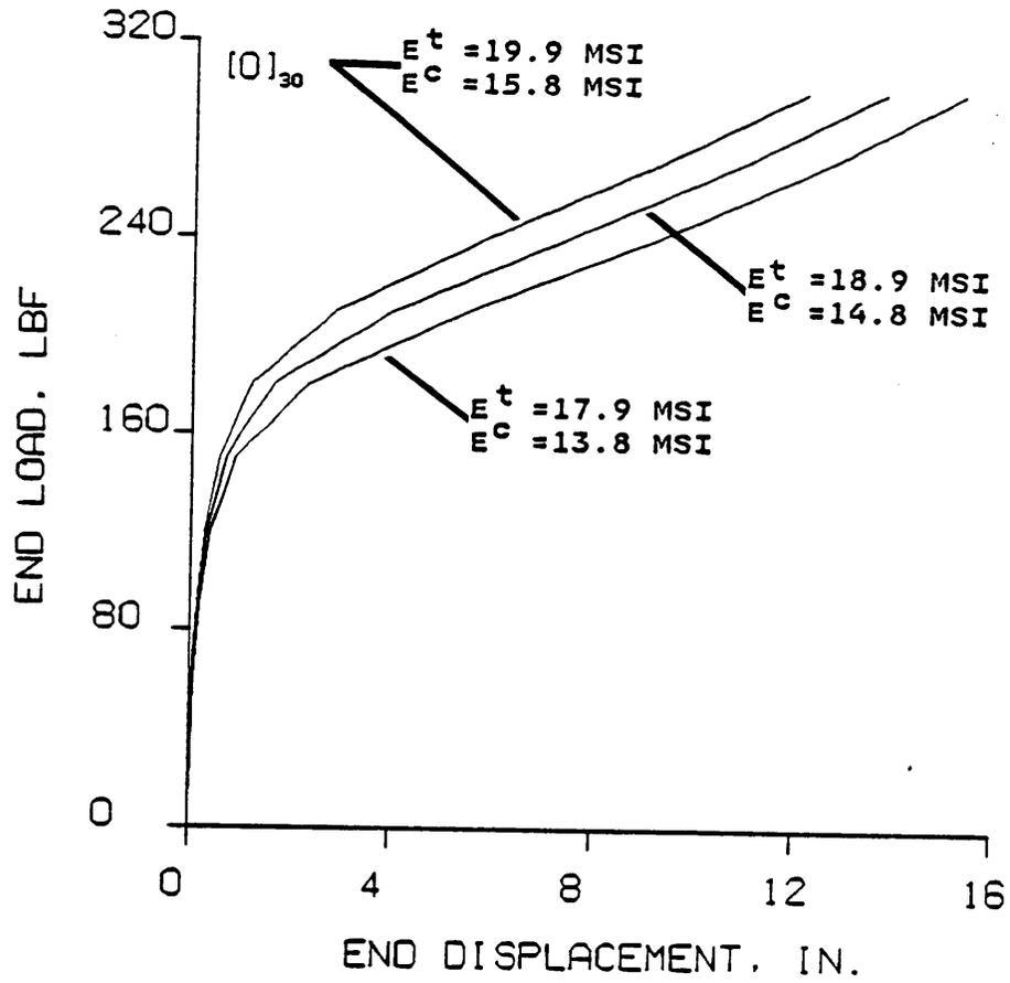
Figure I.1 Effect on the Uncertainty in the Moduli on the Load-Displacement Relation
