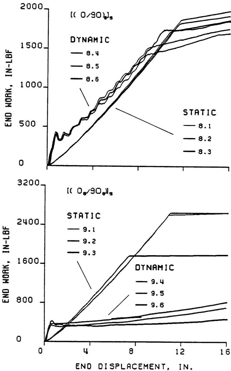
Figure 3.46 End Load Work vs. Displacement for the  $[(0/90)_8]_s$  and  $[(0_g/90_g)_8]_s$  Laminates
