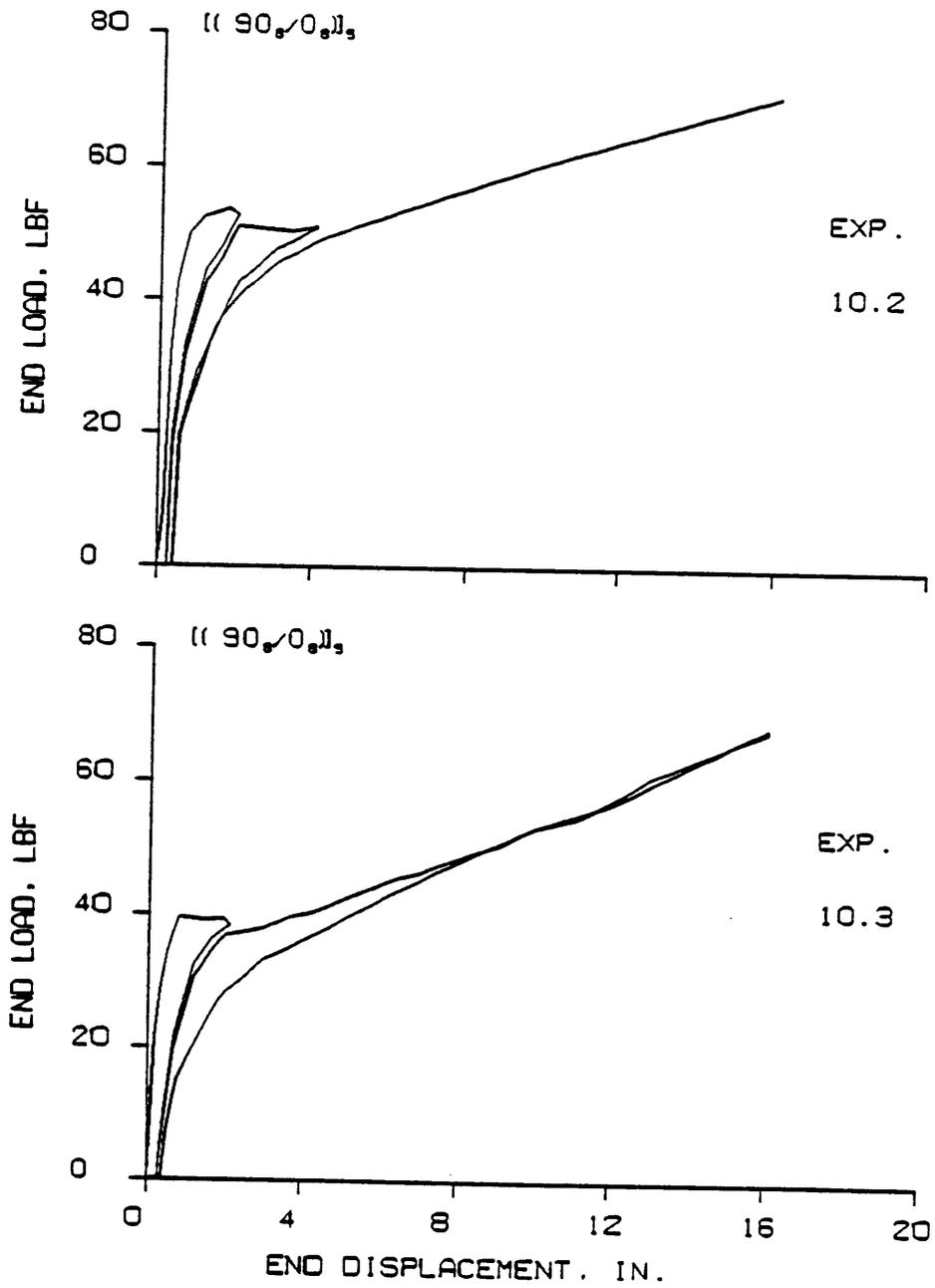
Figure 0.13 Static Load-Displacement Relation for Specimens 10.2 and 10.3
