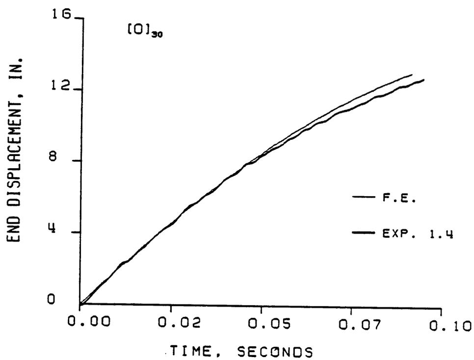
Figure 6.9 Dynamic Displacement vs. Time: Experimental and Finite Element Results for a  $[0]_{30}$  Laminate
