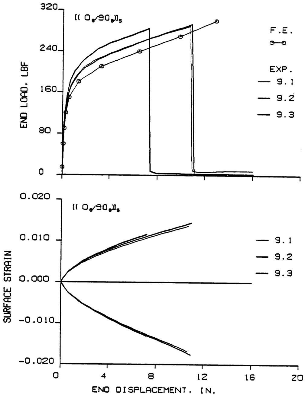
Figure 3.26 Static Load and Strain vs. Displacement for the  $(0_g/90_g)_5$  Laminates
