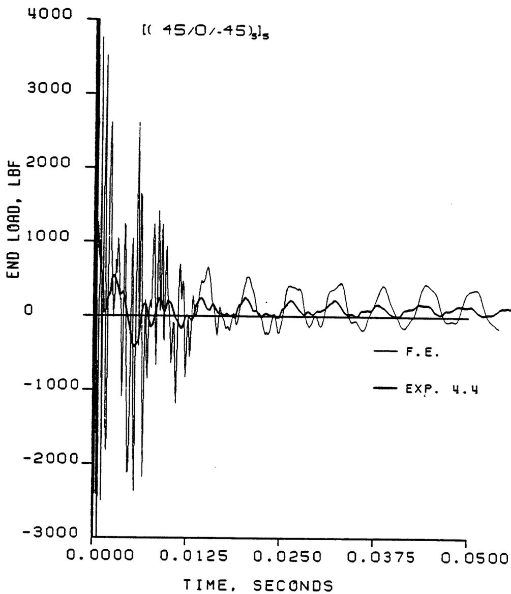
Figure 6.5 Dynamic Load vs. Time: Experimental and Finite Element Results for a [(45/0/-45)<sub>5</sub>]<sub>s</sub> Laminate
