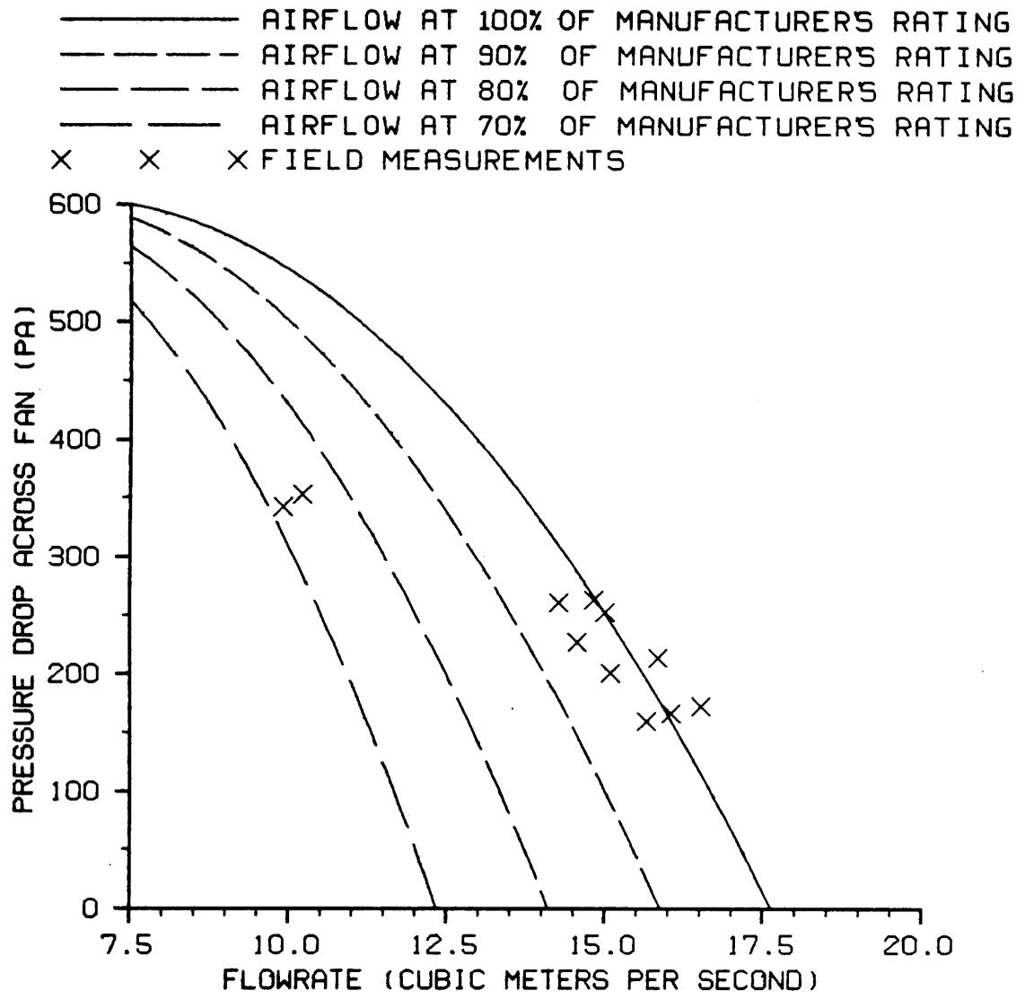
Figure 26. Pressure drop vs. flowrate for a six-trailer unit equipped with an 11.2-kW Aerovent fan (Lewiston, NC).
