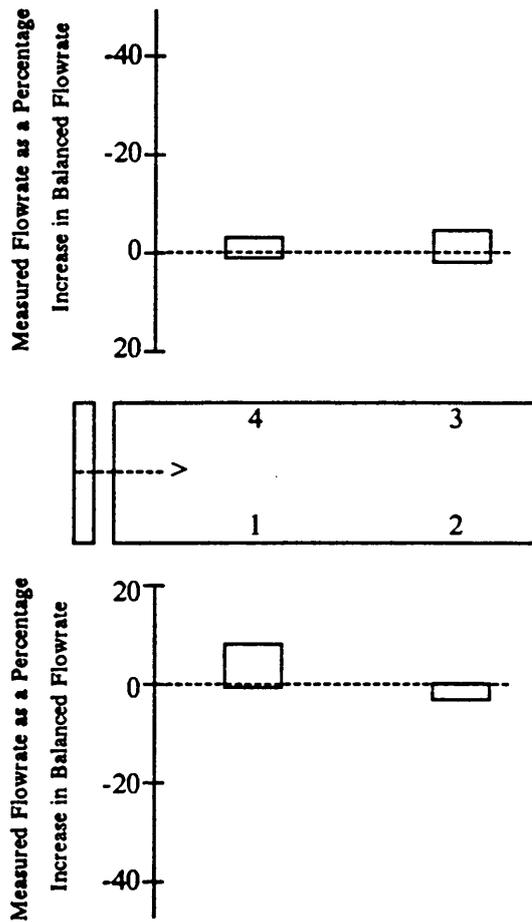
Figure 53. Deviation of measured from balanced flowrate, all combinations in a four-trailer unit, 5.60-kW Long fan, with baffle (Blacksburg, VA).
