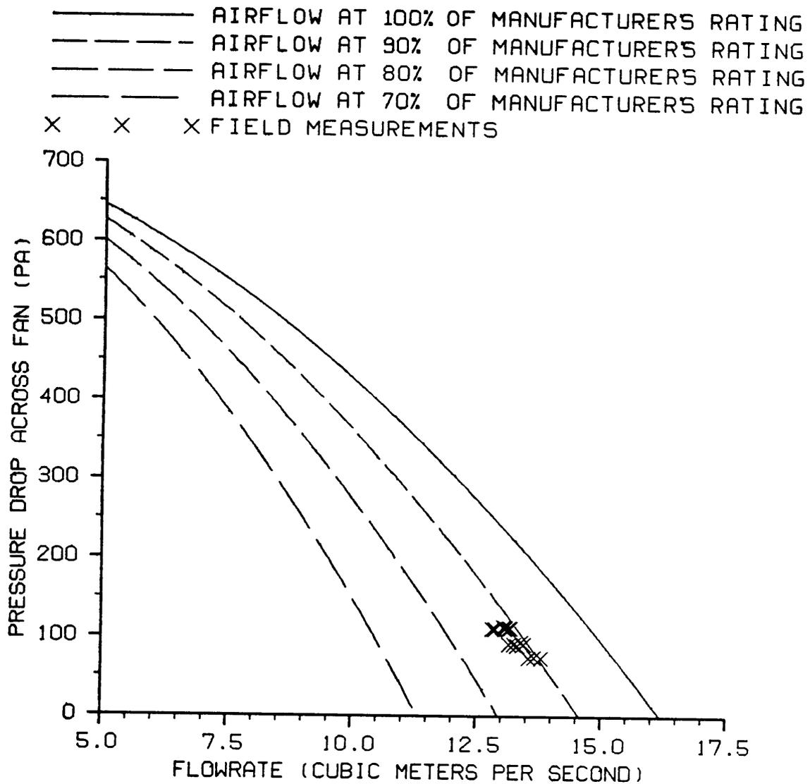
Figure 32. Pressure drop vs. flowrate for an eight-trailer unit equipped with a 7.46-kW Long fan, with baffle (Blacksburg, VA).
