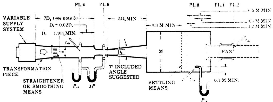
Figure 7. Inlet chamber setup - ducted nozzle on chamber (Reprinted from AMCA, 1985).
