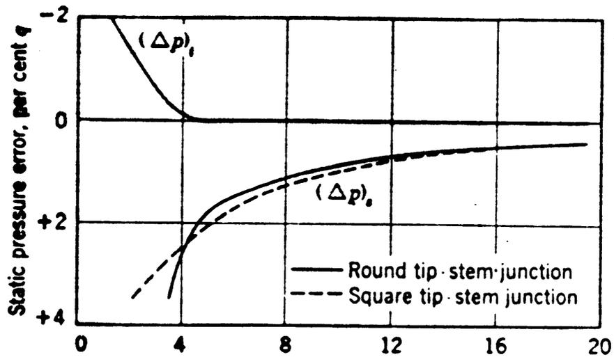
Figure 3. Static orifice distance from tip base or stem centerline, diameters (Reprinted from Pope and Harper, 1966).
