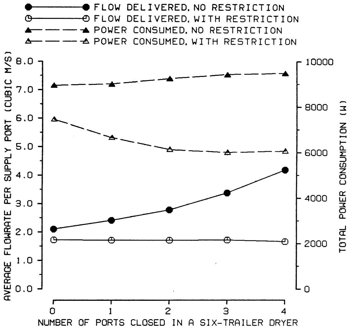
Figure 55. Flow reduction with inlet restrictions.
