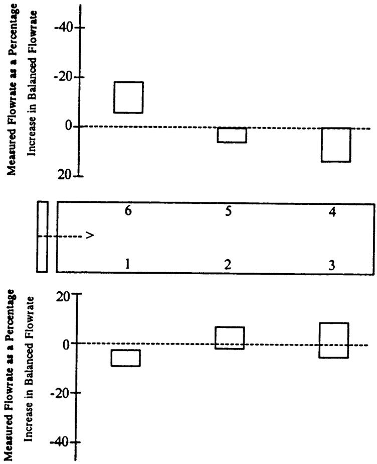
Figure 48. Deviation of measured from balanced flowrate, all combinations in a six-trailer unit, 7.46-kW Aerovent fan (Holland, VA).
