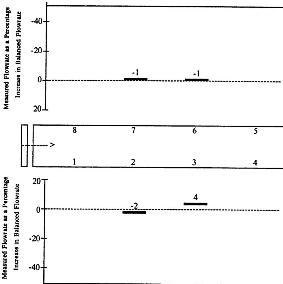
Figure 43. Deviation of measured from balanced flowrate with four ports open in an eight-trailer unit, 11.2-kW Aerovent fan (Lewiston, NC). Dashed lines indicate balanced flow. Solid lines indicate recommended flow which is 51% below balanced flow.
