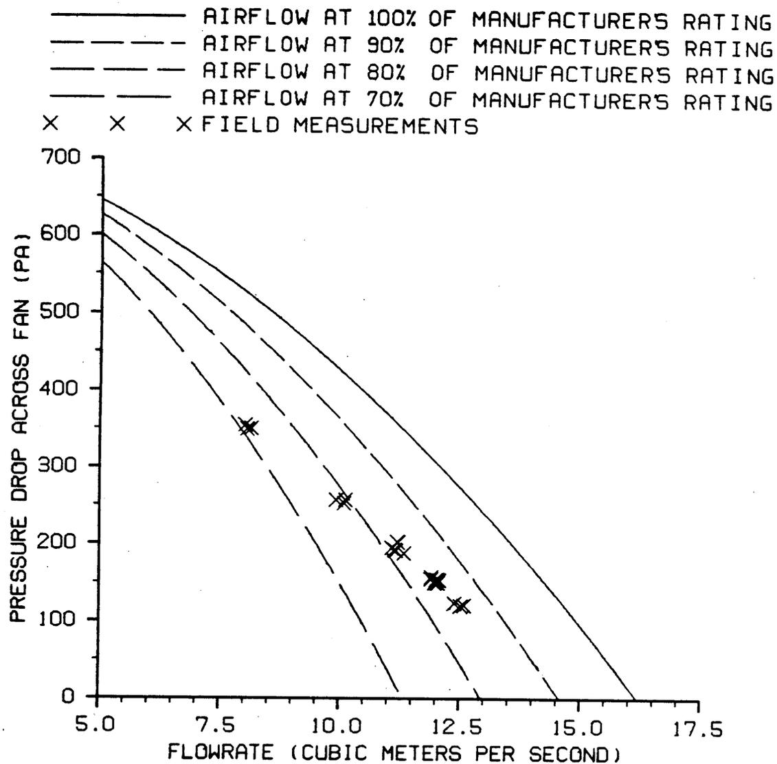
Figure 28. Pressure drop vs. flowrate for a six-trailer unit equipped with a 7.46-kW Long fan (Blacksburg, VA).
