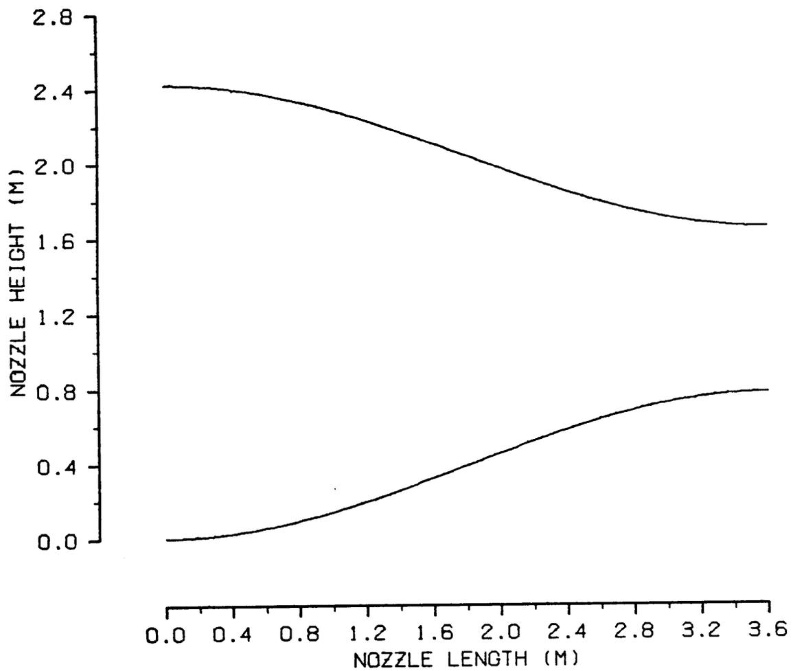
Figure 10. Profile of nozzle used for calibration of perforated plate.
