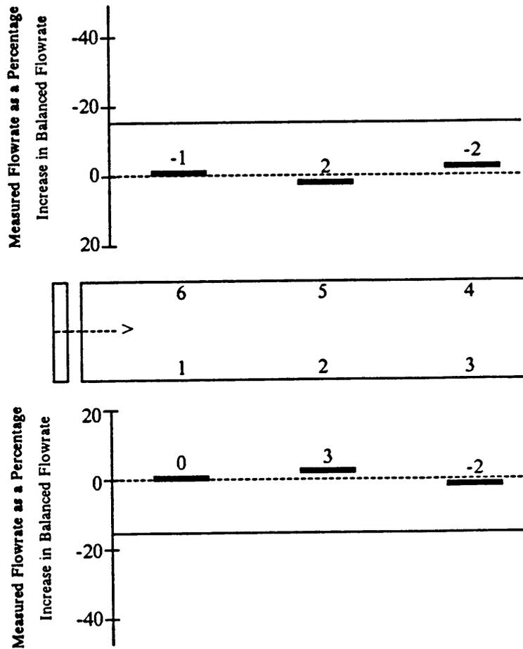
Figure 40. Deviation of measured from balanced flowrate with all ports open in a six-trailer unit, 7.46-kW Long fan, with baffle (Blacksburg, VA). Dashed lines indicate balanced flow. Solid lines indicate recommended flow which is 15% below balanced flow.
