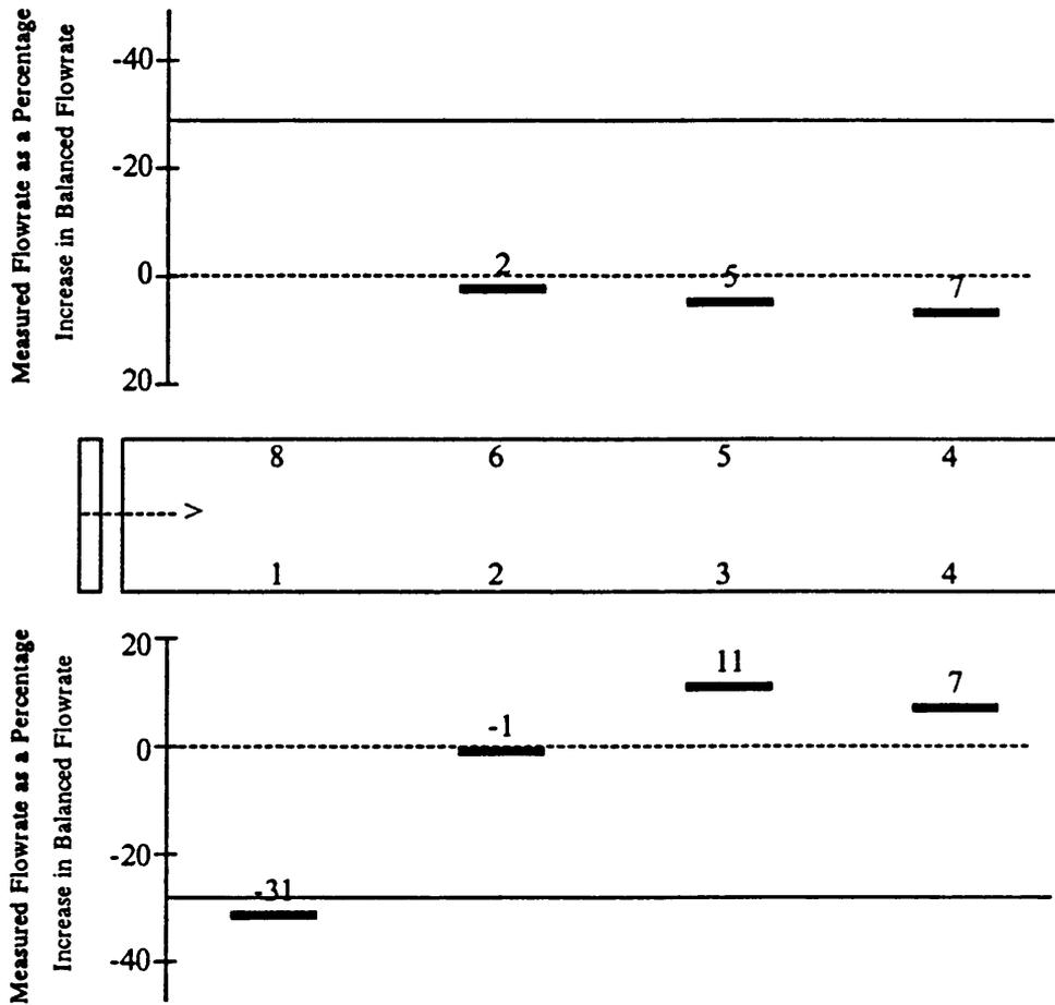
Figure 45. Deviation of measured from balanced flowrate with seven ports open in an eight-trailer unit, 11.2-kW Aerovent fan (Lewiston, NC). Dashed lines indicate balanced flow. Solid lines indicate recommended flow which is 28% below balanced flow.
