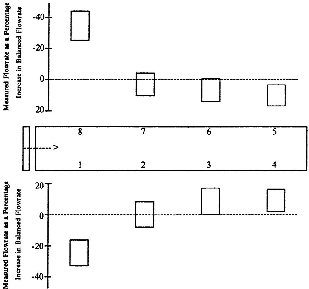
Figure 46. Deviation of measured from balanced flowrate, all combinations in an eight-trailer unit, 11.2-kW Aerovent fan (Lewiston, NC).
