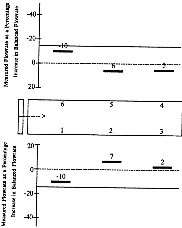
Figure 38. Deviation of measured from balanced flowrate with all ports open in a six-trailer unit, 7.46-kW Long fan (Blacksburg, VA). Dashed lines indicate balanced flow. Solid lines indicate recommended flow which is 16% below balanced flow.
