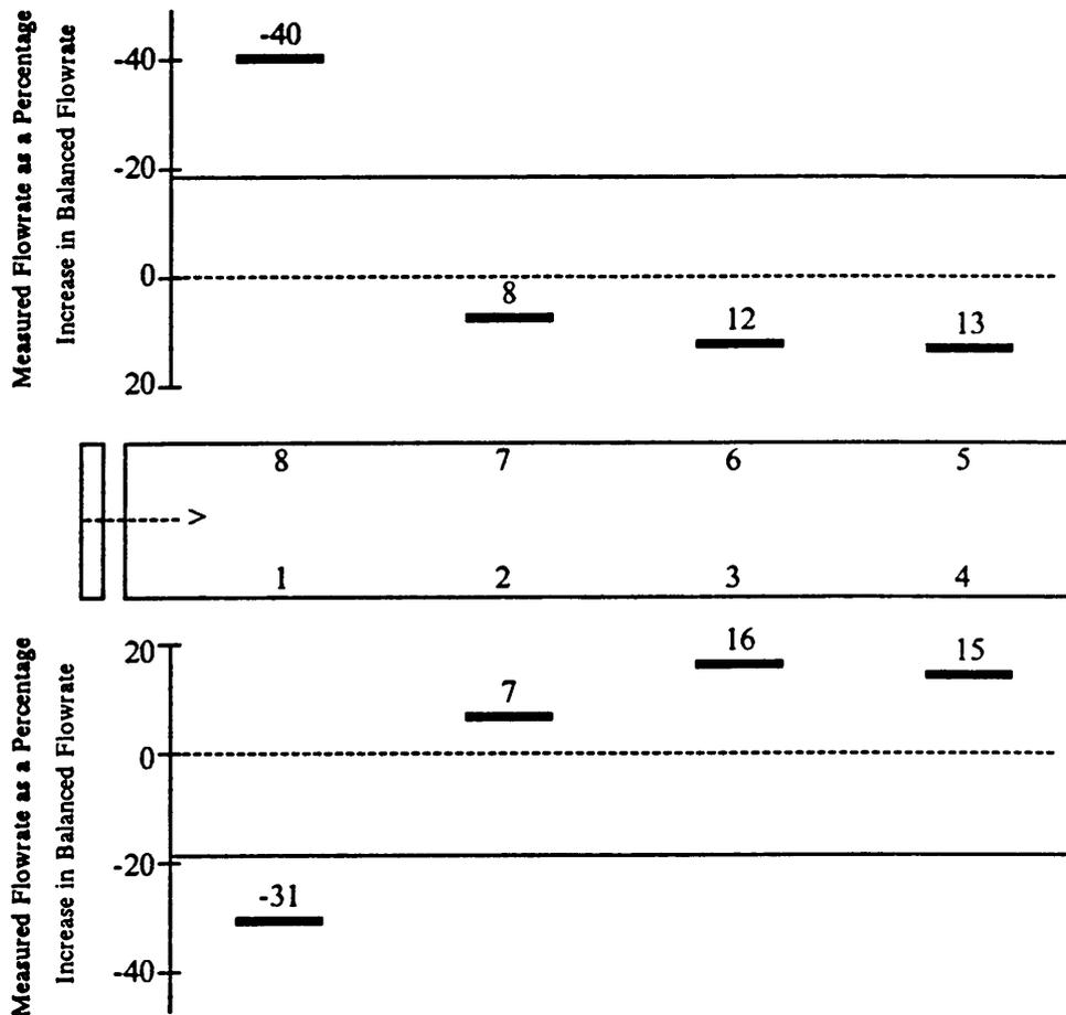
Figure 34. Deviation of measured from balanced flowrate with all ports open in an eight-trailer unit, 11.2-kW Aerovent fan (Lewiston, NC). Dashed lines indicate balanced flow. Solid lines indicate recommended flow which is 19% below balanced flow.
