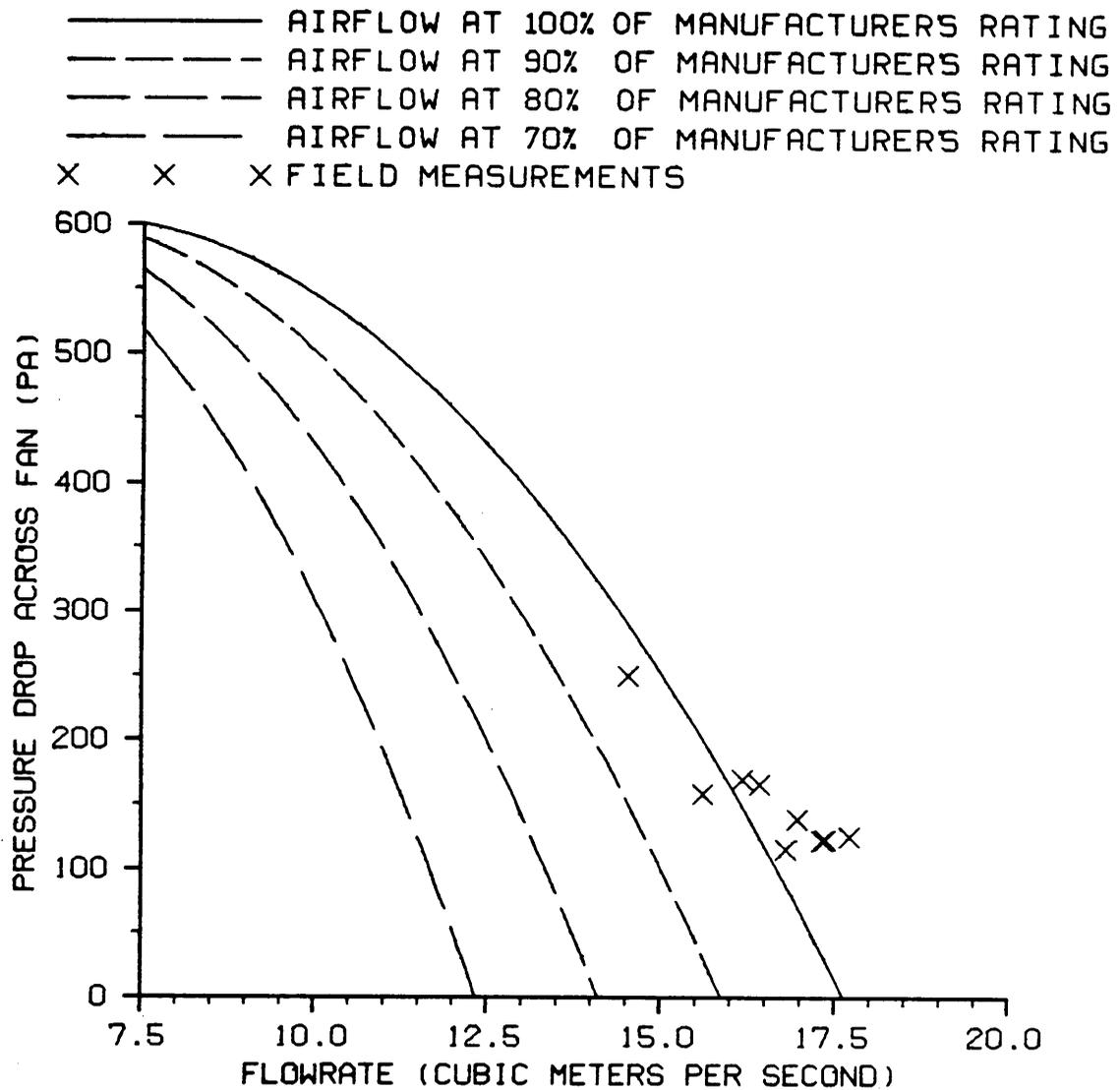
Figure 25. Pressure drop vs. flowrate for an eight-trailer unit equipped with an 11.2-kW Aerovent fan (Lewiston, NC).
