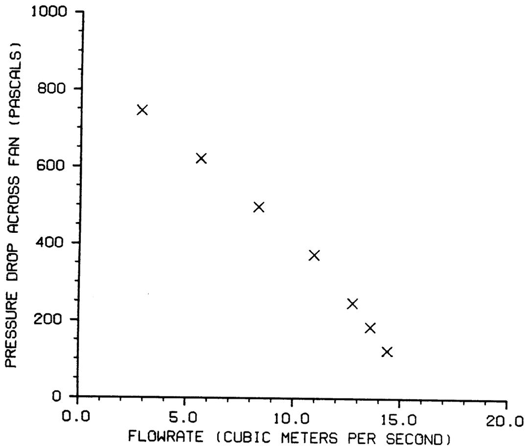
Figure 16. Manufacturer's fan rating curve for 7.46-kW Aerovent (Adapted from Aerovent performance data).
