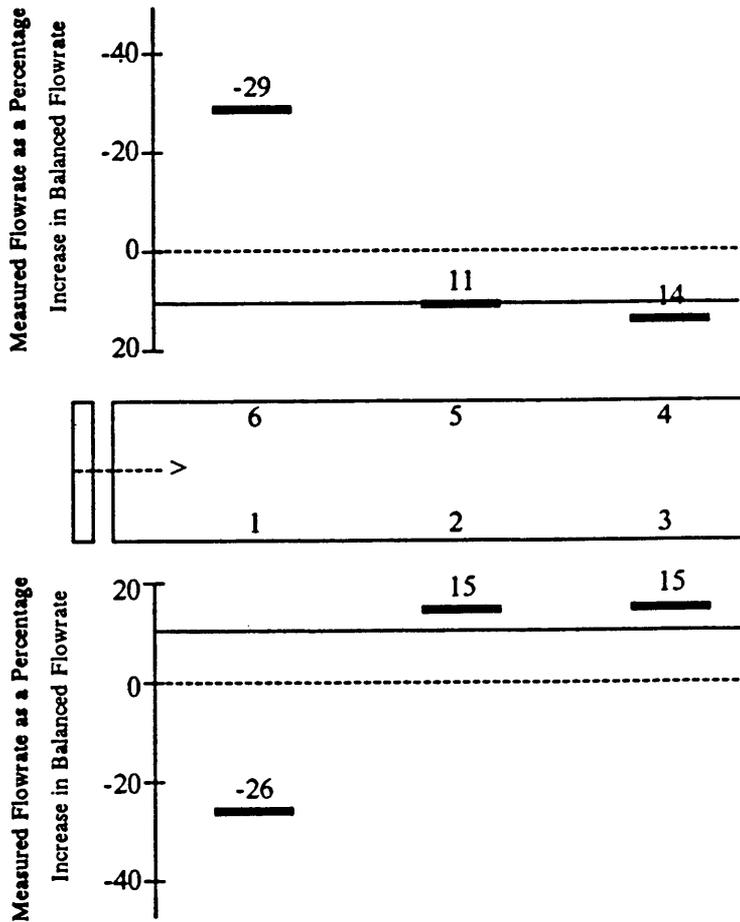
Figure 37. Deviation of measured from balanced flowrate with all ports open in a six-trailer unit, 5.60-kW Long fan (Blacksburg, VA). Dashed lines indicate balanced flow. Solid lines indicate recommended flow which is 11% above balanced flow.
