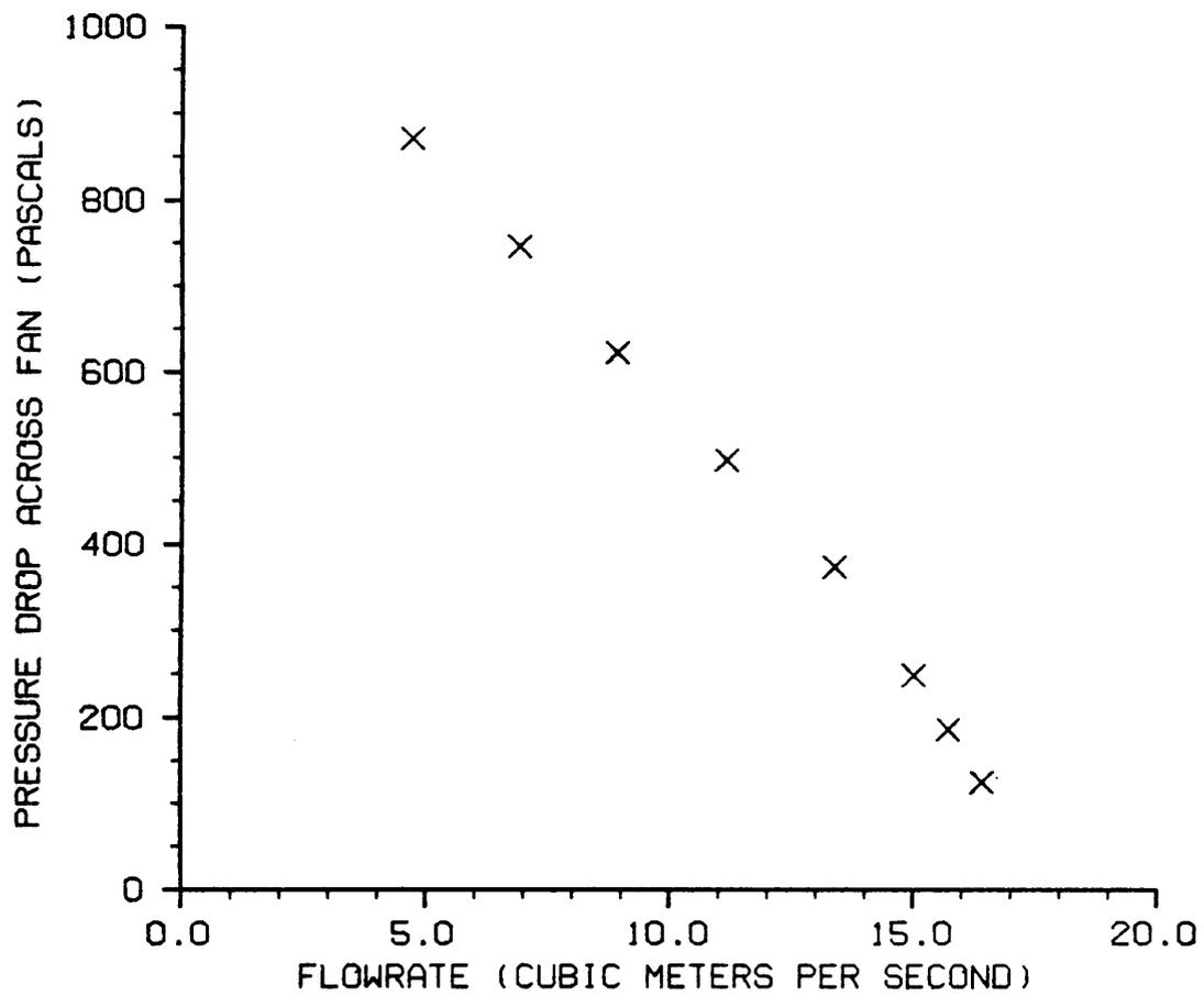
Figure 15. Manufacturer's fan rating curve for 11.2-kW Aerovent (Adapted from Aerovent performance data).
