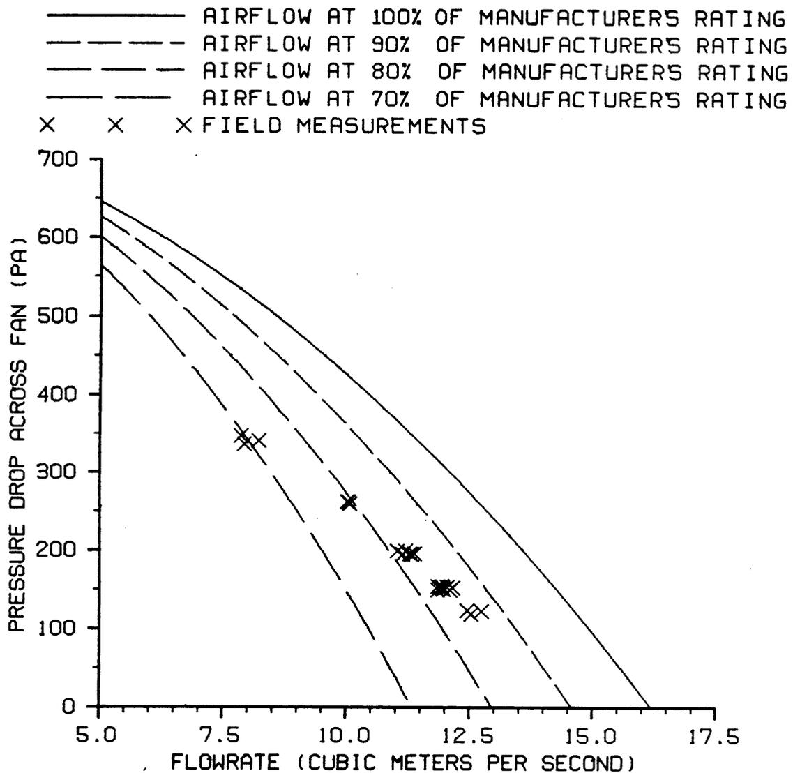
Figure 30. Pressure drop vs. flowrate for a six-trailer unit equipped with a 7.46-kW Long fan, with baffle (Blacksburg, VA).
