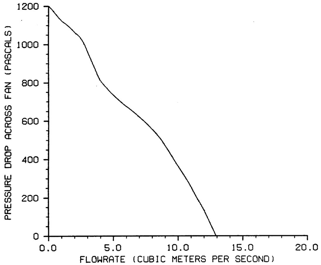
**Figure 17.** Manufacturer's fan rating curve for 5.60-kW Long (Adapted from Long performance data).
