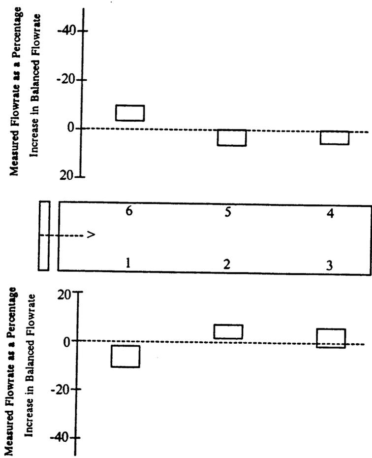
Figure 50. Deviation of measured from balanced flowrate, all combinations in a six-trailer unit, 7.46-kW Long fan (Blacksburg, VA).
