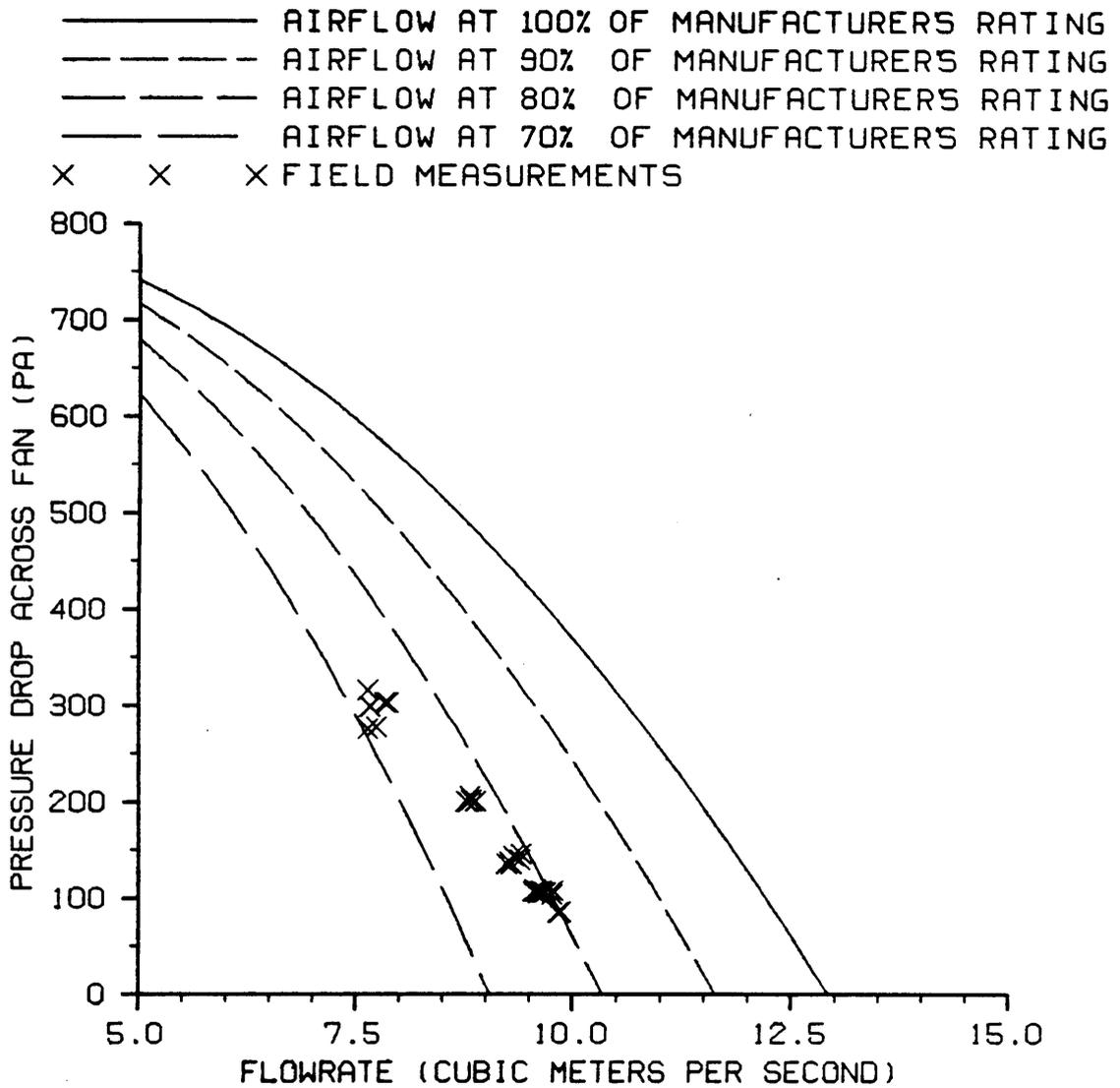
Figure 29. Pressure drop vs. flowrate for a six-trailer unit equipped with a 5.60-kW Long fan (Blacksburg, VA).
