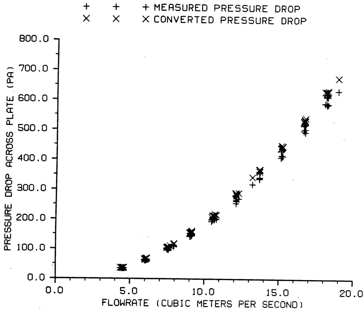
Figure 20. Measured flowrates, and measured and adjusted pressure drops on two separate days.
