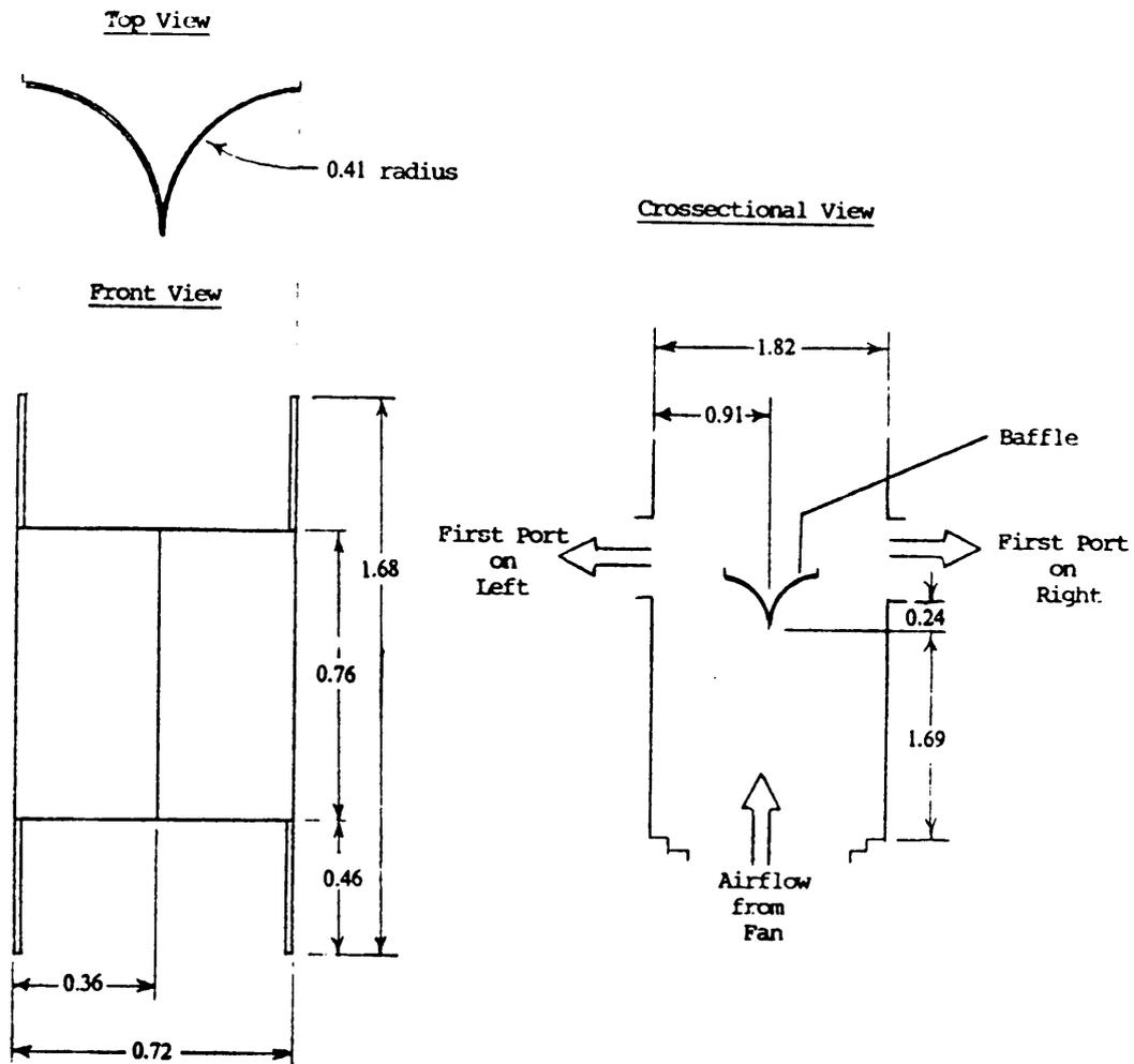
Figure 19. Baffle dimensions and position in dryer plenum (All dimensions in meters).
