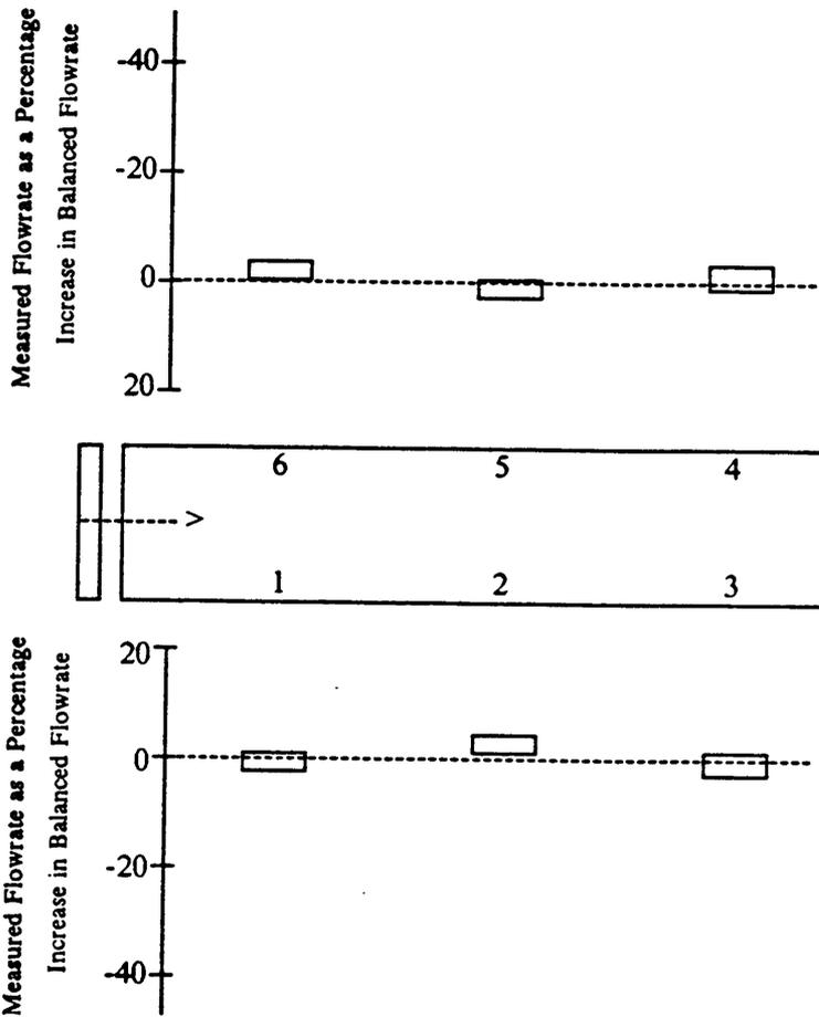
Figure 52. Deviation of measured from balanced flowrate, all combinations in a six-trailer unit, 7.46-kW Long fan, with baffle (Blacksburg, VA).
