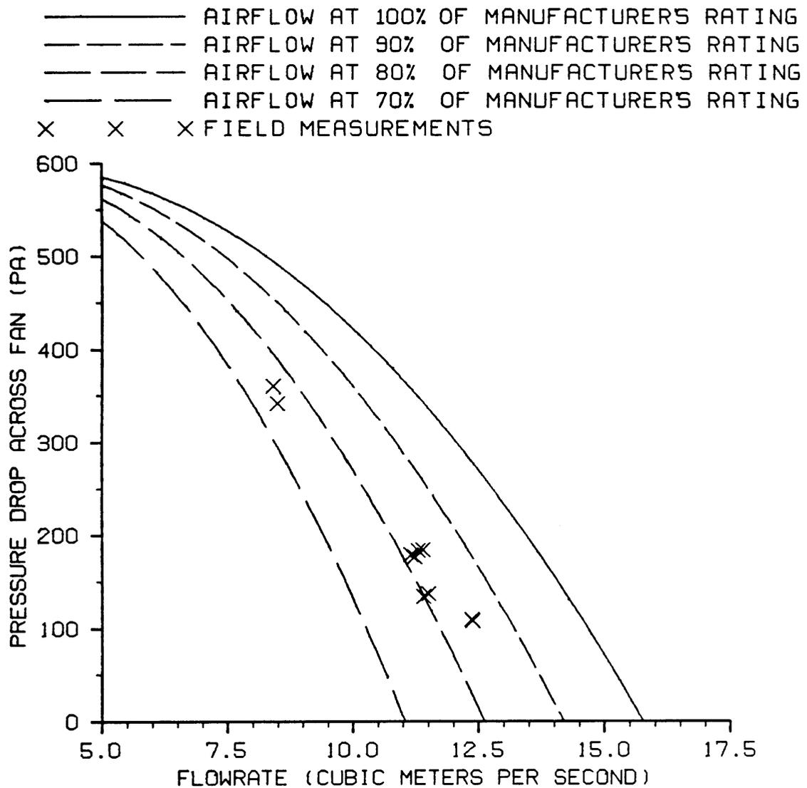
Figure 27. Pressure drop vs. flowrate for a six-trailer unit equipped with a 7.46-kW Aerovent fan (Holland, VA).
