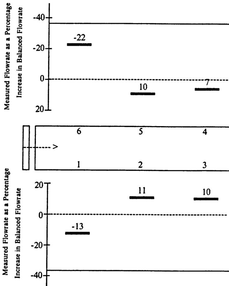
Figure 35. Deviation of measured from balanced flowrate with all ports open in a six-trailer unit, 11.2-kW Aerovent fan (Lewiston, NC). Dashed lines indicate balanced flow. Solid lines indicate recommended flow which is 37% below balanced flow.
