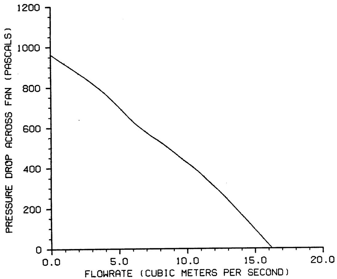
Figure 18. Manufacturer's fan rating curve for 7.46-kW Long (Adapted from Long performance data).
