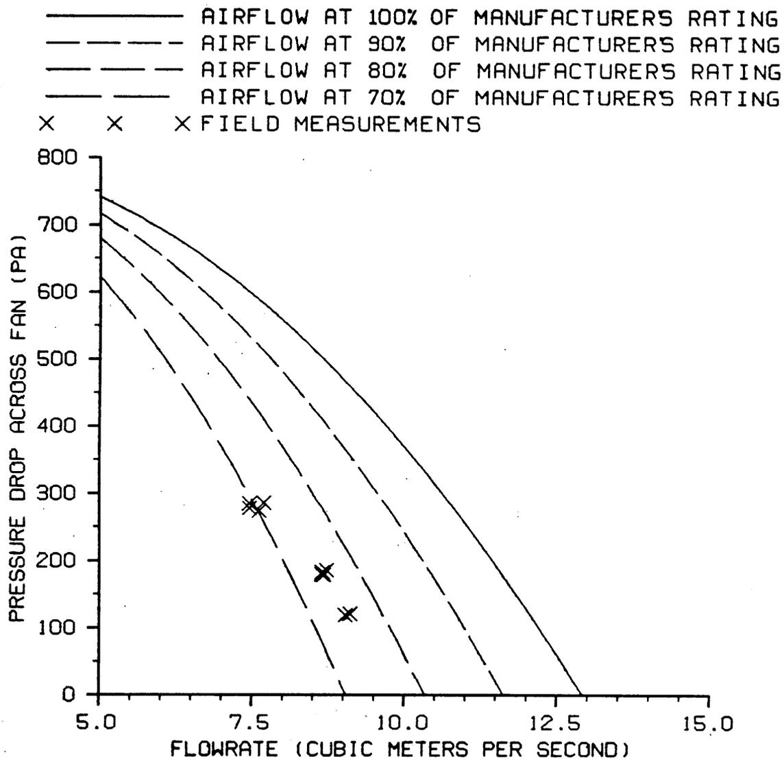
Figure 33. Pressure drop vs. flowrate for a four-trailer unit equipped with a 5.60-kW Long fan, with baffle (Blacksburg, VA).
