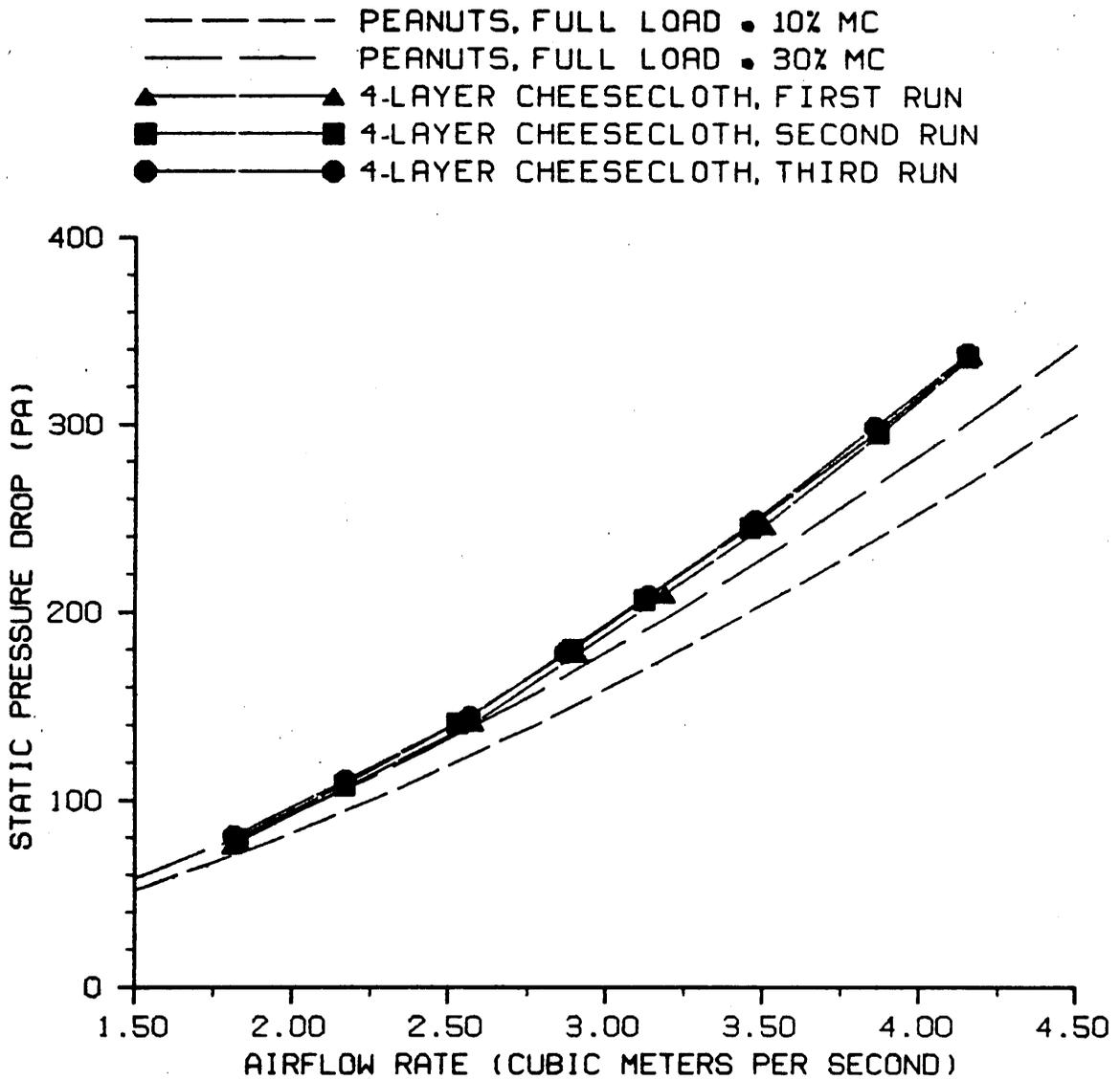
Figure 23. Pressure drop-flowrate for Resistance Plate No. 7, with resistance of a trailer filled with peanuts.
