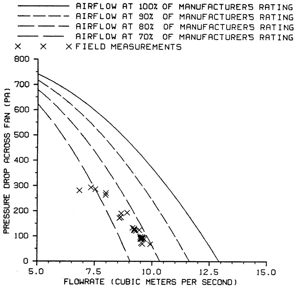
Figure 31. Pressure drop vs. flowrate for a six-trailer unit equipped with a 5.60-kW Long fan, with baffle (Blacksburg, VA).
