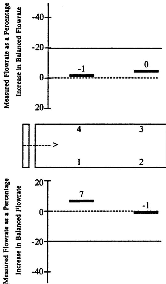
Figure 41. Deviation of measured from balanced flowrate with all ports open in a four-trailer unit, 5.60-kW Long fan, with baffle (Blacksburg, VA). Dashed lines indicate balanced flow. Solid lines indicate recommended flow which is 20% below balanced flow.
