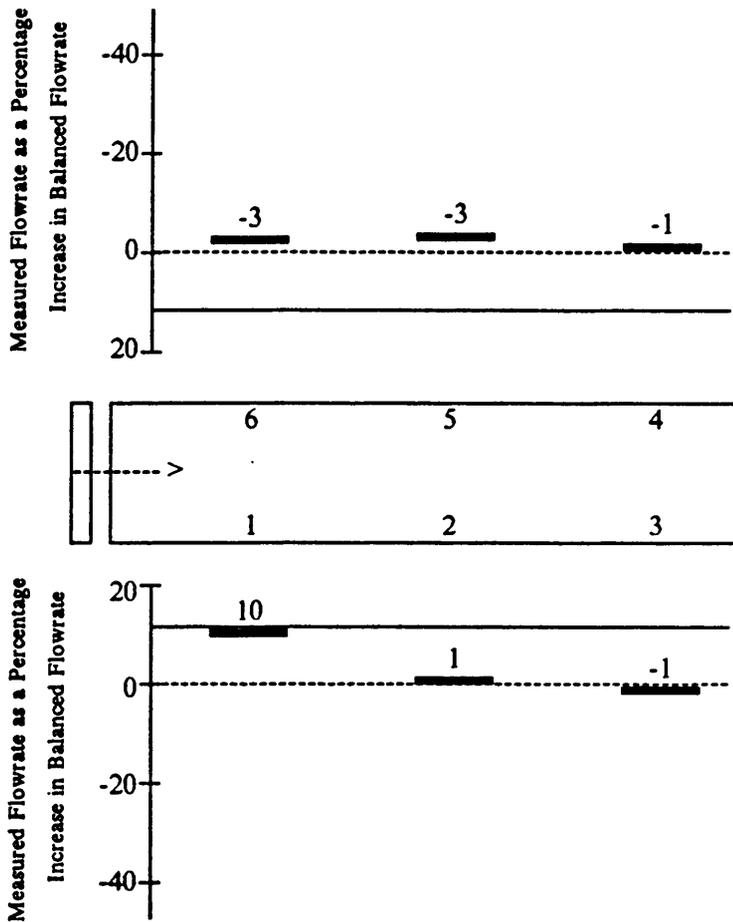
Figure 39. Deviation of measured from balanced flowrate with all ports open in a six-trailer unit, 5.60-kW Long fan, with baffle (Blacksbrug, VA). Dashed lines indicate balanced flow. Solid lines indicate recommended flow which is 12% above balanced flow.
