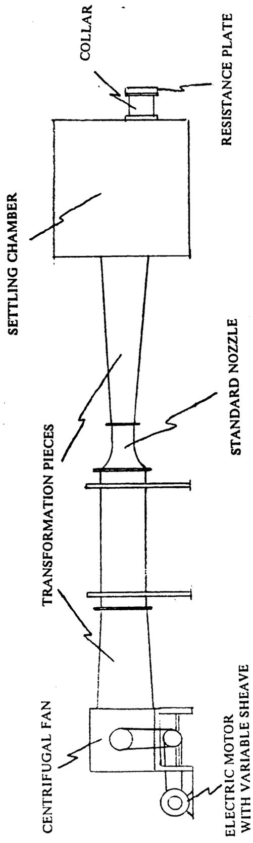
Figure 13. Experimental setup for calibration of resistance plates.
