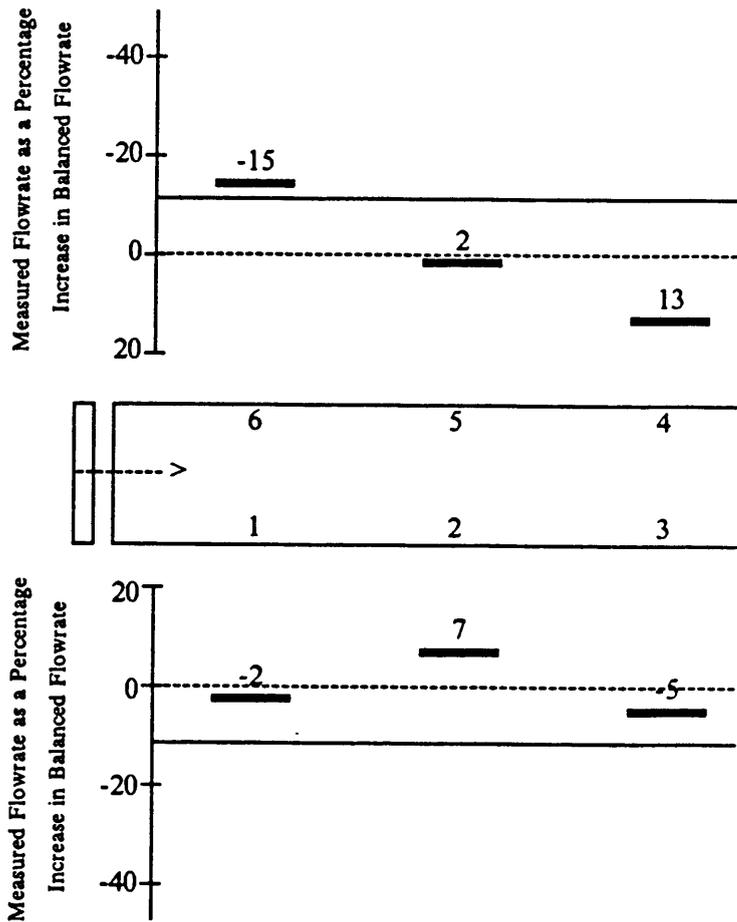
Figure 36. Deviation of measured from balanced flowrate with all ports open in a six-trailer unit, 7.46-kW Aerovent fan (Holland, VA). Dashed lines indicate balanced flow. Solid lines indicate recommended flow which is 11% below balanced flow.
