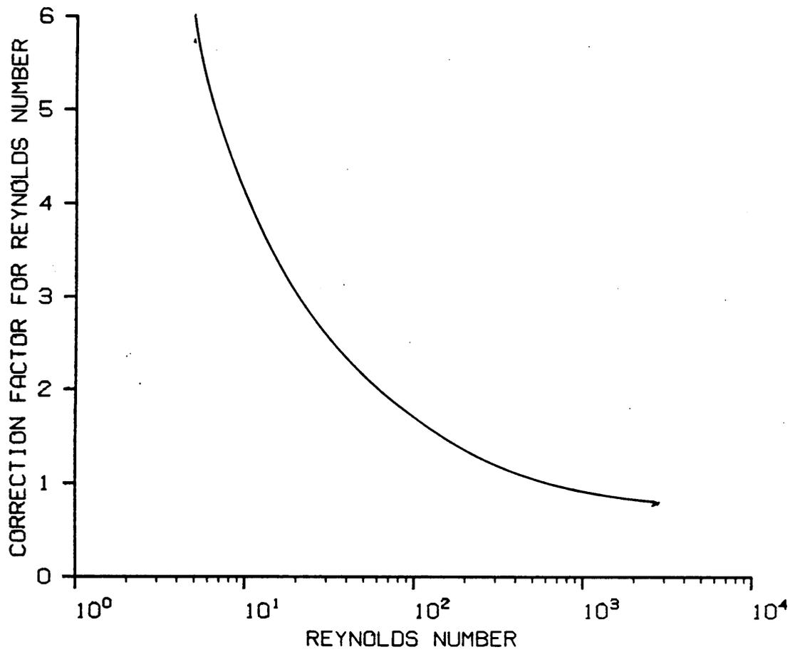
Figure 5. Pressure drop coefficient correction factor for  $Re > 2000$  (Adapted from Engineering Sciences Data Unit, 1972).
