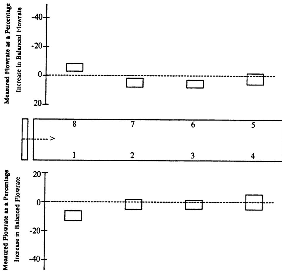
Figure 54. Deviation of measured from balanced flowrate, all combinations in an eight-trailer unit, 7.46-kW Long fan, with baffle (Blacksburg, VA).
