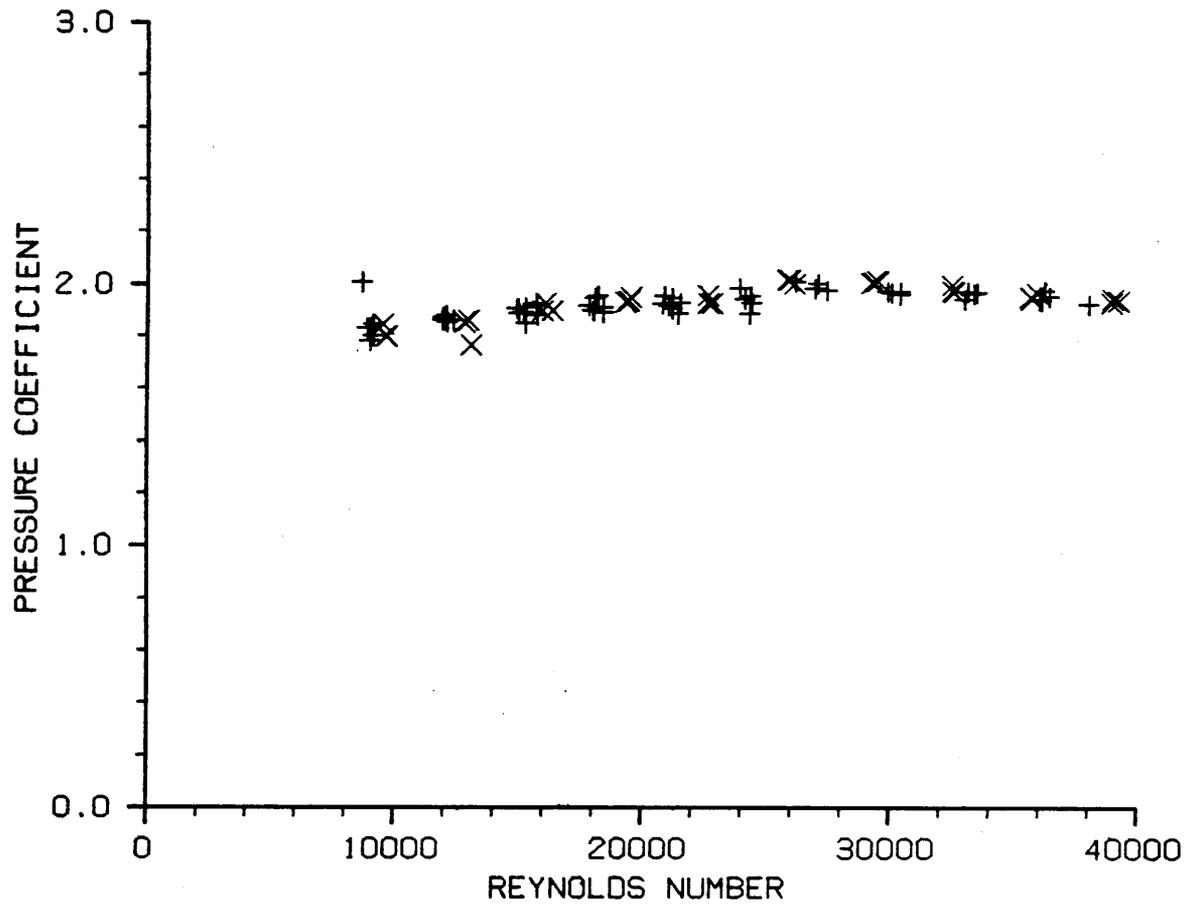
Figure 21. Pressure coefficient vs. Reynolds number for perforated plate.
