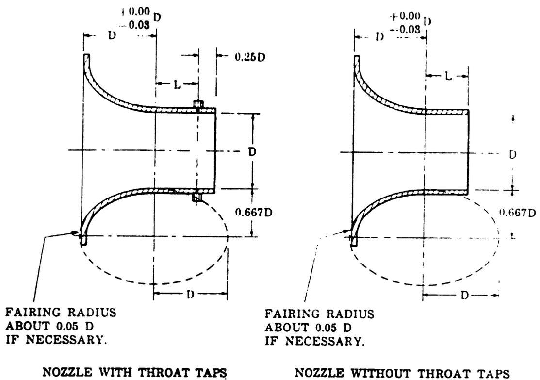
Figure 2. Standard nozzle (Reprinted from AMCA, 1985).
