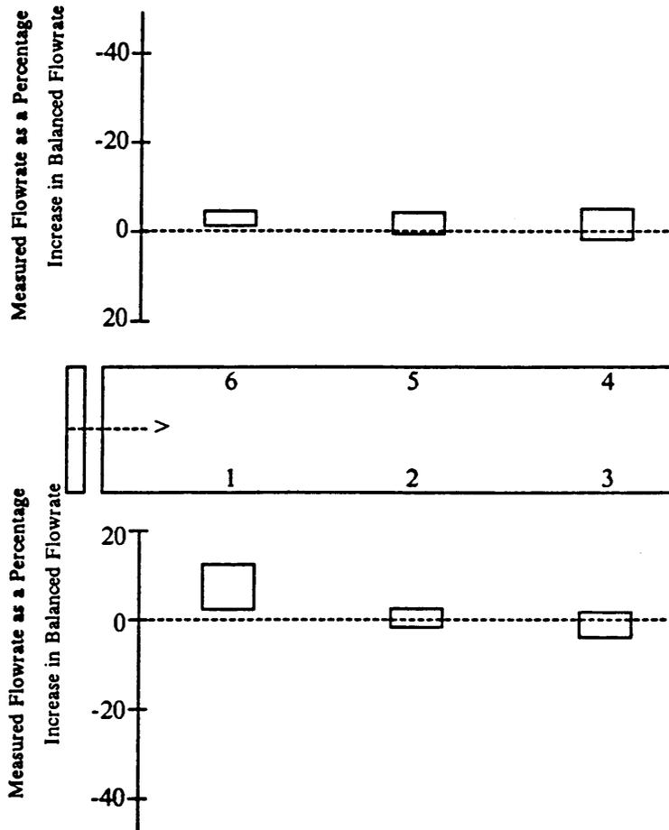
Figure 51. Deviation of measured from balanced flowrate, all combinations in a six-trailer unit, 5.60-kW Long fan, with baffle (Blacksburg, VA).
