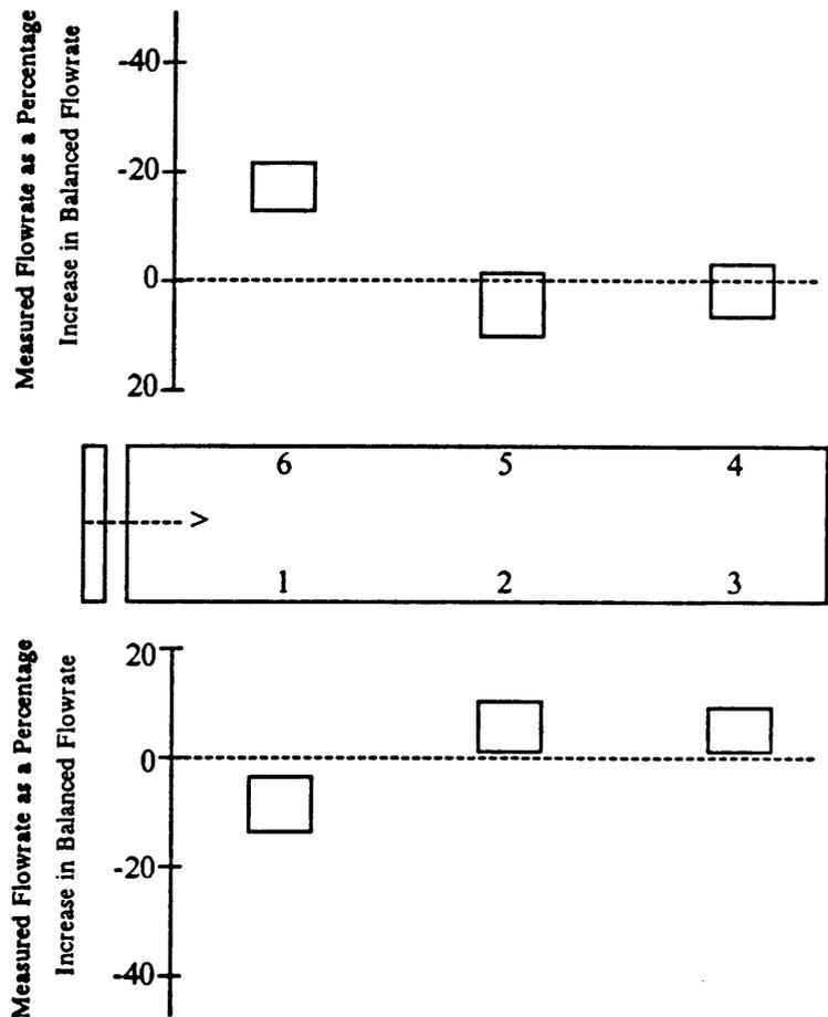
Figure 47. Deviation of measured from balanced flowrate, all combinations in a six-trailer unit, 11.2-kW Aerovent fan (Lewiston, NC).
