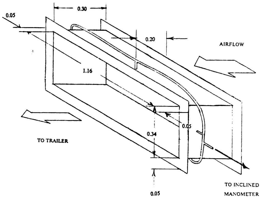
Figure 12. Rectangular collar with piezometer ring (All dimensions in meters).
