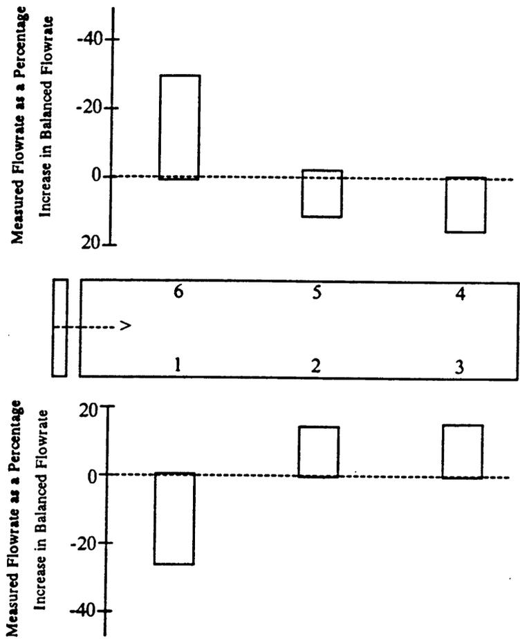
Figure 49. Deviation of measured from balanced flowrate, all combinations in a six-trailer unit, 5.60-kW Long fan (Blacksburg, VA).
