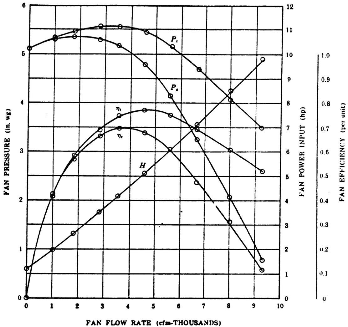
Figure 8. Typical fan performance curves (Reprinted from AMCA, 1985).
