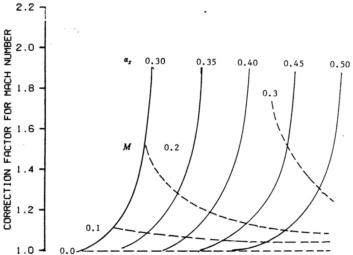
Figure 6. Pressure drop coefficient correction factor for  $M > 0$  (Adapted from Engineering Sciences Data Unit, 1972).
