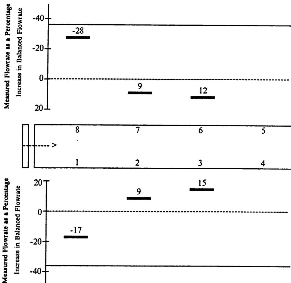
Figure 44. Deviation of measured from balanced flowrate with six ports open in an eight-trailer unit, 11.2-kW Aerovent fan (Lewiston, NC). Dashed lines indicate balanced flow. Solid lines indicate recommended flow which is 36% below balanced flow.
