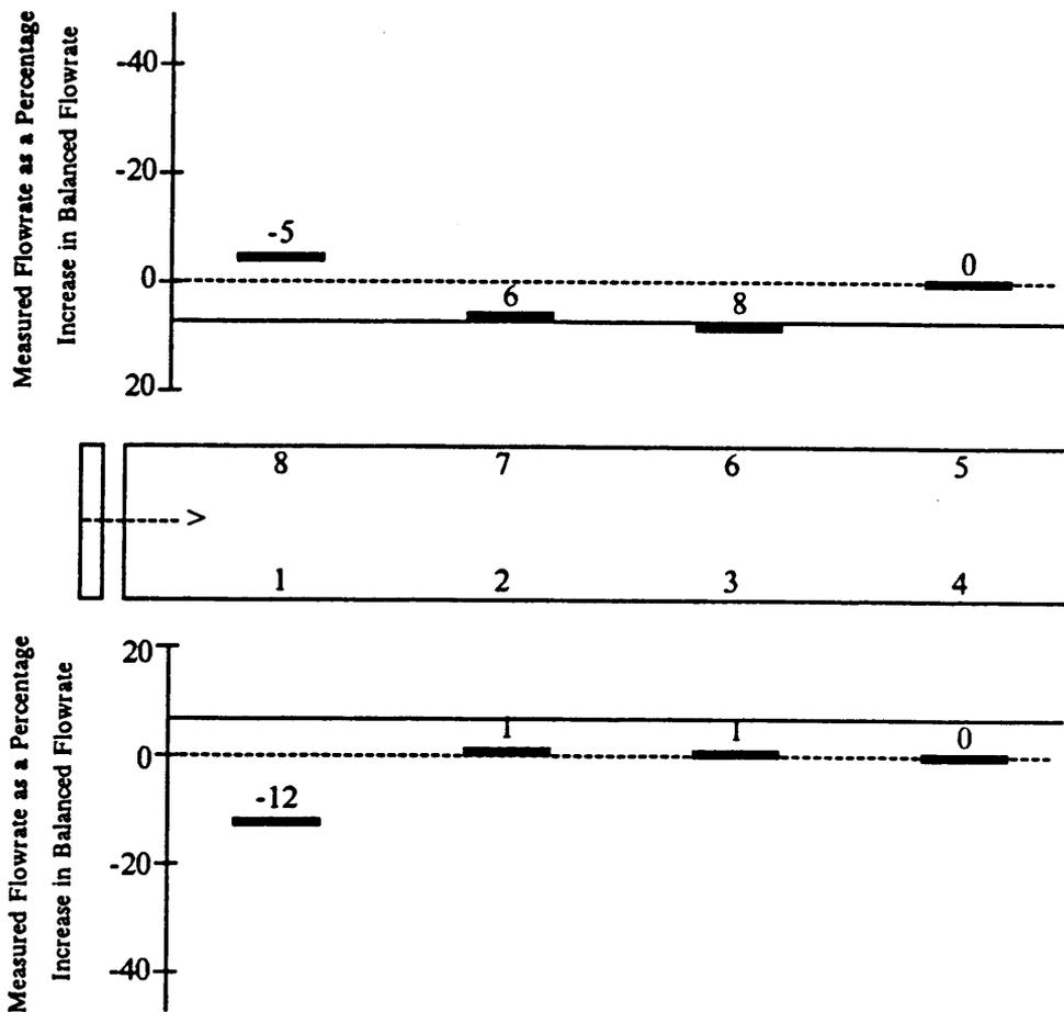
Figure 42. Deviation of measured from balanced flowrate with all ports open in an eight-trailer unit, 7.46-kW Long fan, with baffle (Blacksburg, VA). Dashed lines indicate balanced flow. Solid lines indicate recommended flow which is 7% above balanced flow.
