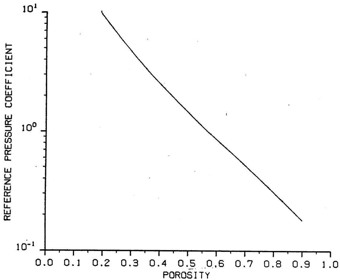
Figure 4. Reference pressure coefficient as a function of porosity (Adapted from Engineering Sciences Data Unit, 1972).
