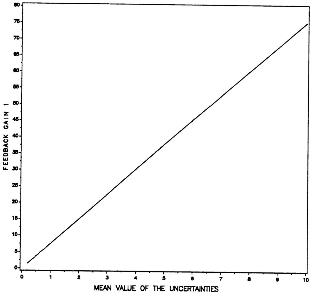
Fig. 4.6: Feedback Gain 1 for  $\overline{\Delta\gamma}/\gamma_m = 0.5$
