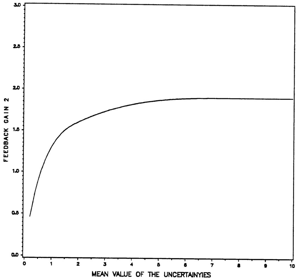
Fig. 4.7: Feedback Gain 2 for  $\overline{\Delta\gamma}/\gamma_m = 0.1$
