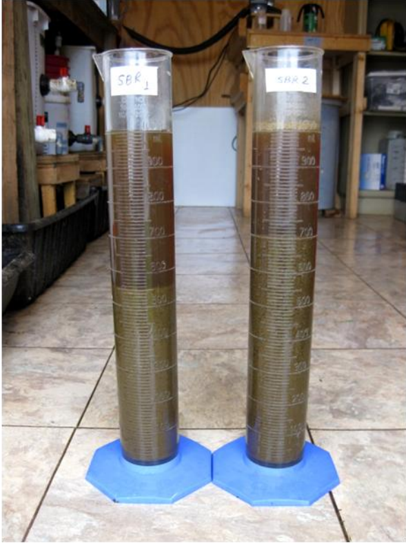
Figure 16. Sludge volume index test using 1 L graduated cylinder
