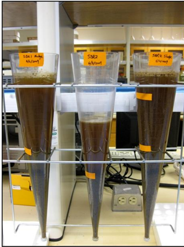
Figure 26. Gravity thickening tests using Imhoff cones
