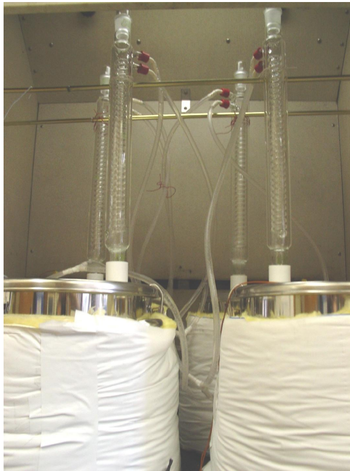
Figure 5: Vapor Condensers with cooling water tubes
