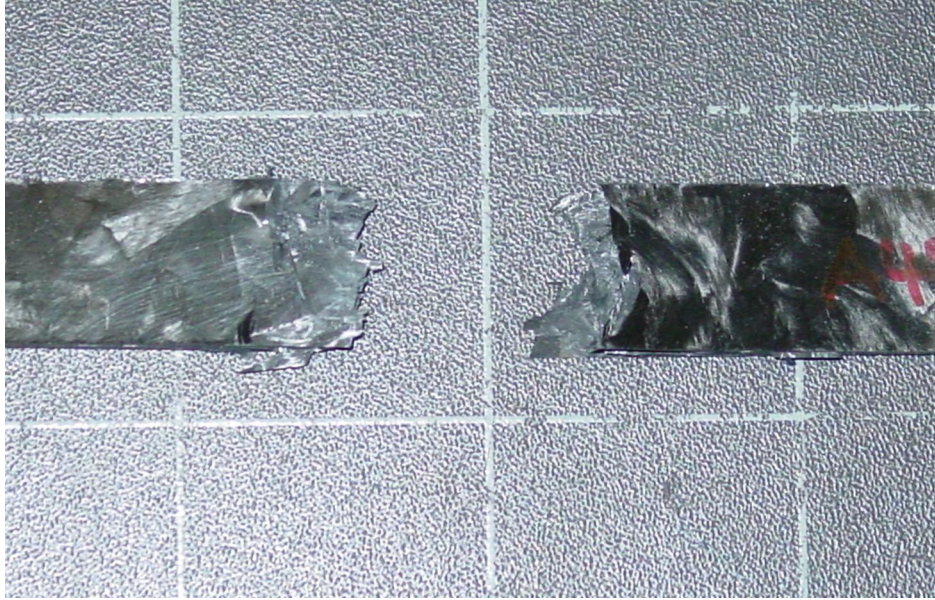
Figure 16: Typical tensile failure for Material A
