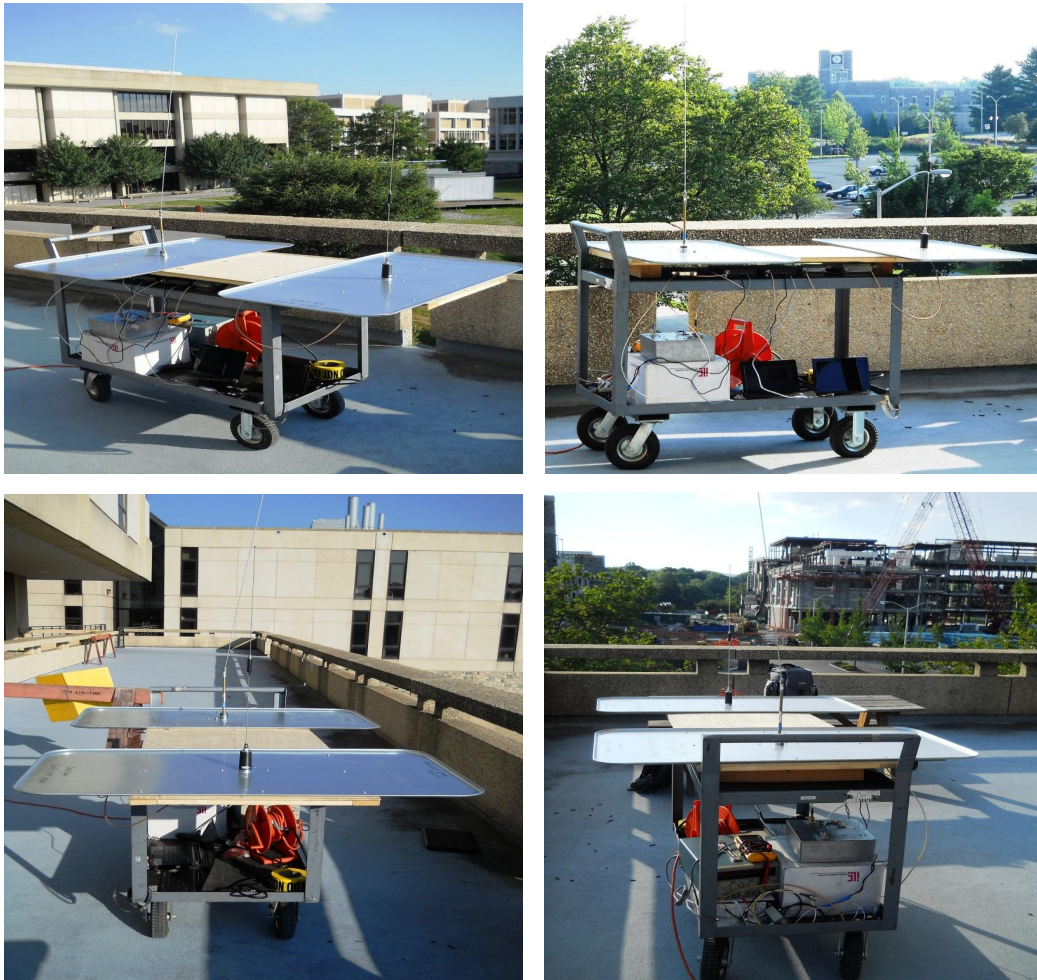
Figure 5.2: Location and test fixture. The reconfigurable antenna and the commercial antenna (in this case Laird Tech. Model C150/450C) appear to the left and right, respectively, in two figures. The automatic electronic tuner is the aluminium box located directly under the reconfigurable antenna. Views are top/left , approximately Southwest; top/right , approximately Northwest; bottom/left , approximately South; bottom/right , approximately North.
