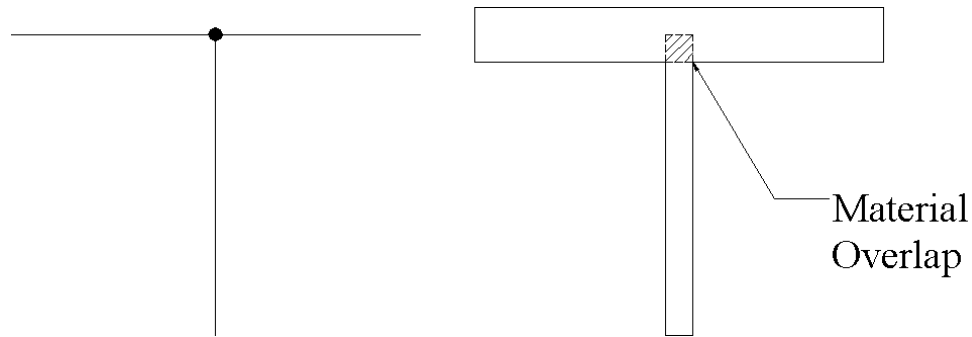
Figure 4.3-1: Material Overlap of Shell Elements
