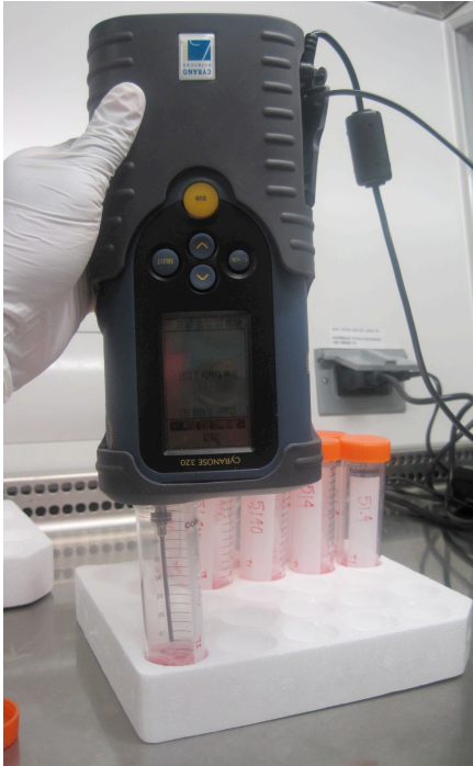
Figure 4.4 Insertion of snout into tube for sampling
