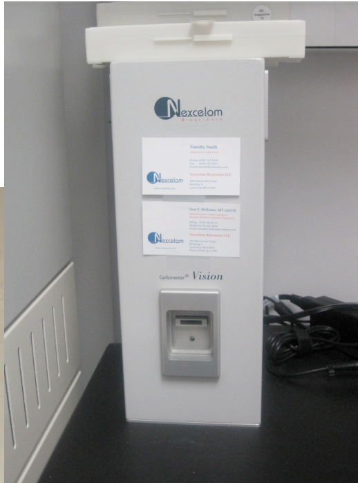
Figure 4.4 Disposable slide and Cellometer used for cell counting
