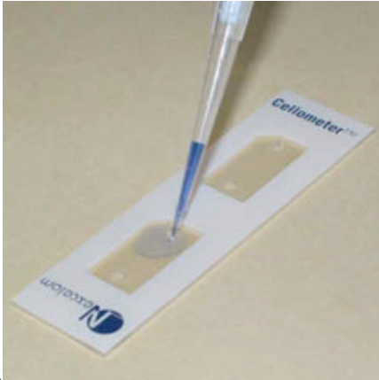
Figure 4.4 Disposable slide and Cellometer used for cell counting
