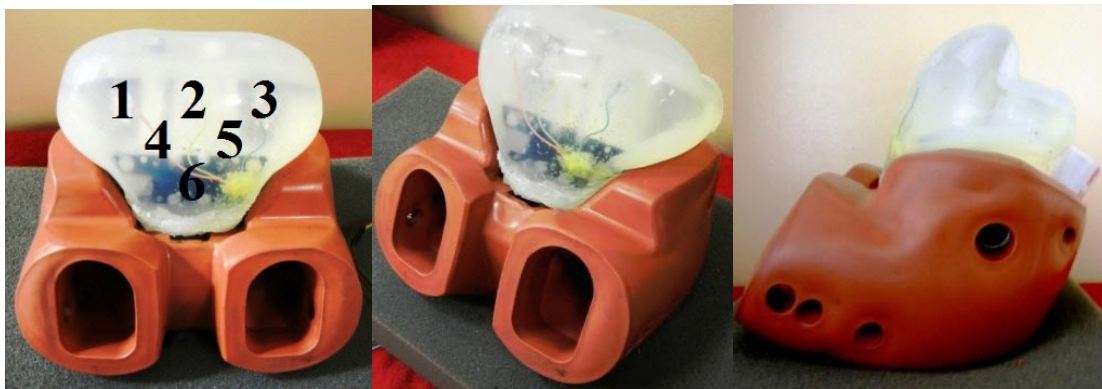
Figure 3.3: Instrumented biofidelic abdominal insert mounted on the HIII 6yo modified pelvis.
