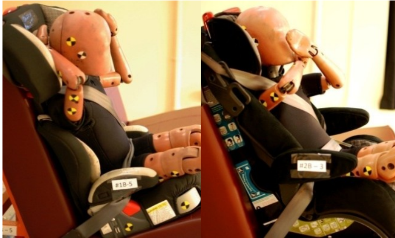
Figure A.5: SD1 (left) and SD2 (right) post-test belt placement for the modified dummy
