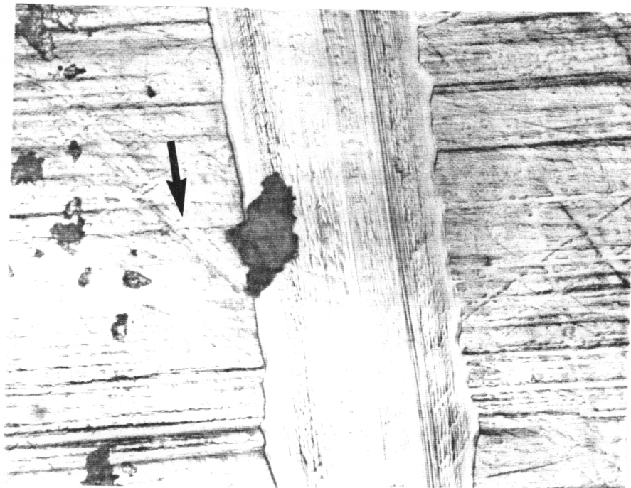
Figure 35. Optical micrographs of the wear track of the untreated 85/15 blend at 15N-5cm/s a) after 3000 cycles b) after 3600 cycles
