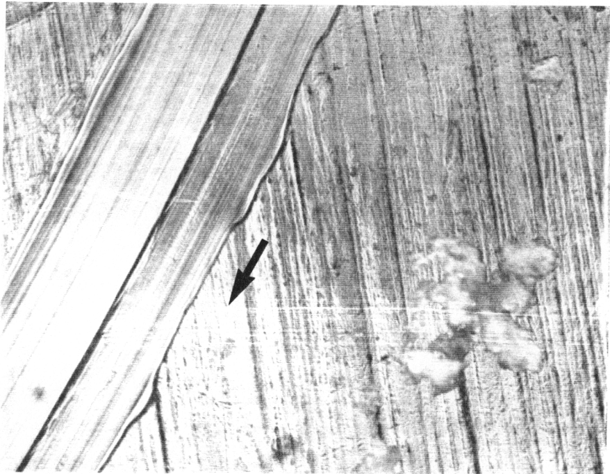
Figure 33. Optical micrographs of the wear track of the untreated 85/15 blend at 15N-5cm/s a) after 600 cycles b) after 1200 cycles
