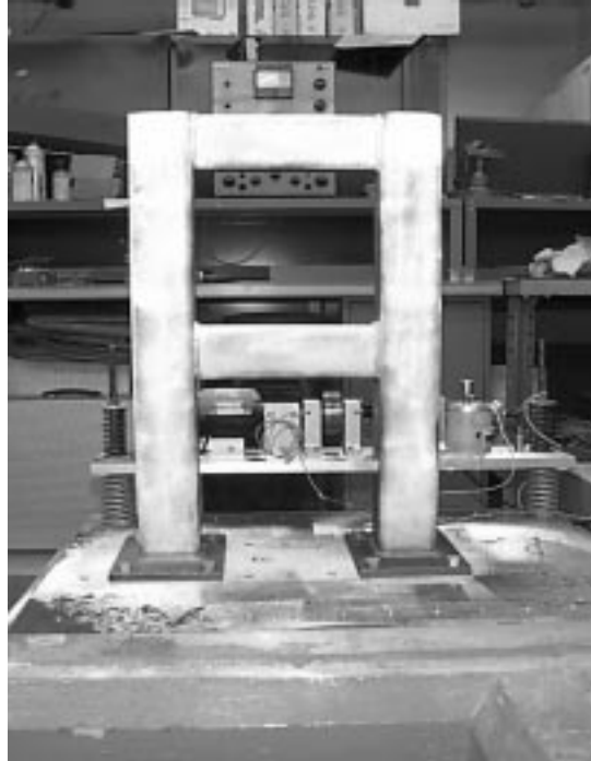
Figure 29. Test structure bolted to test stand
