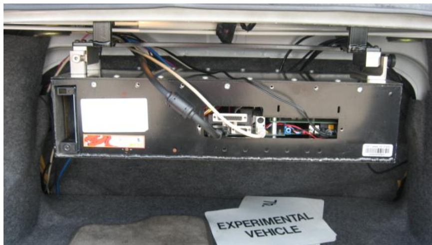
Figure 4. Data Acquisition System in the trunk of the participant vehicle.
