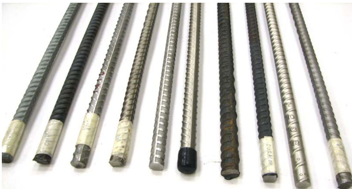
Figure 4. Different types of reinforcing bars that are being offered as being more corrosion resistant than traditional black steel reinforcing bars.
