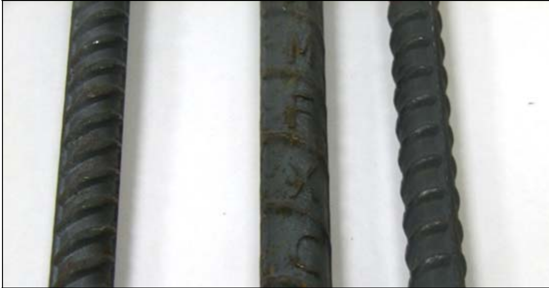
Figure 5. Similar looking bars, but bar on left is black steel and two bars on right are alloyed for improved corrosion resistance.
