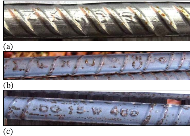
Figure 18. Mill identification marks on (a) stainless steel clad, (b) MMFX 2, and (c) Duracorr bars.
