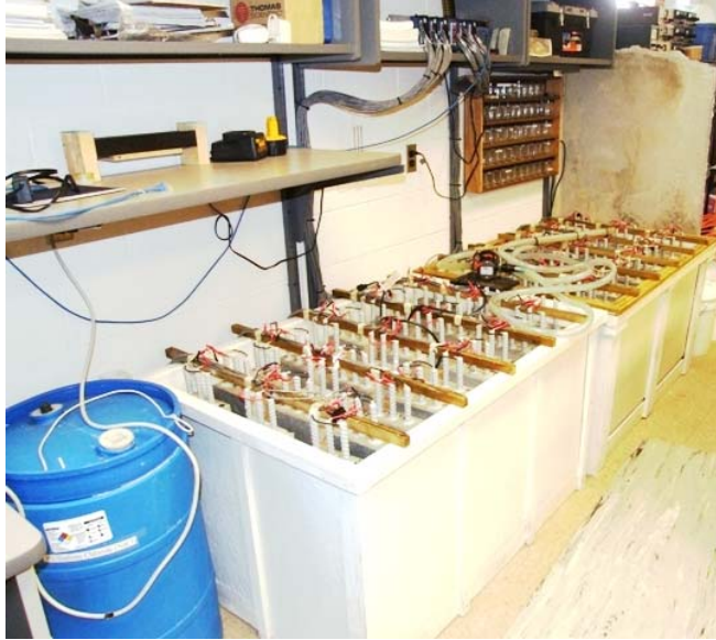
Figure I1. Tombstone test setup: 3% saltwater storage tank in lower left corner, with tombstone immersion tanks adjacent to saltwater storage tank and data acquisition system above tombstone tanks (top of picture).
