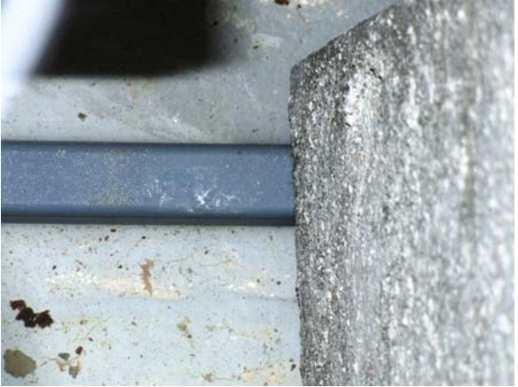
Figure I2. Close-up of 1" plastic square tube that functions as a sample booster
