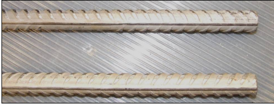
Figure 7. Two types of stainless steel reinforcement: one bar is a duplex and the other is an austenitic stainless steel.
