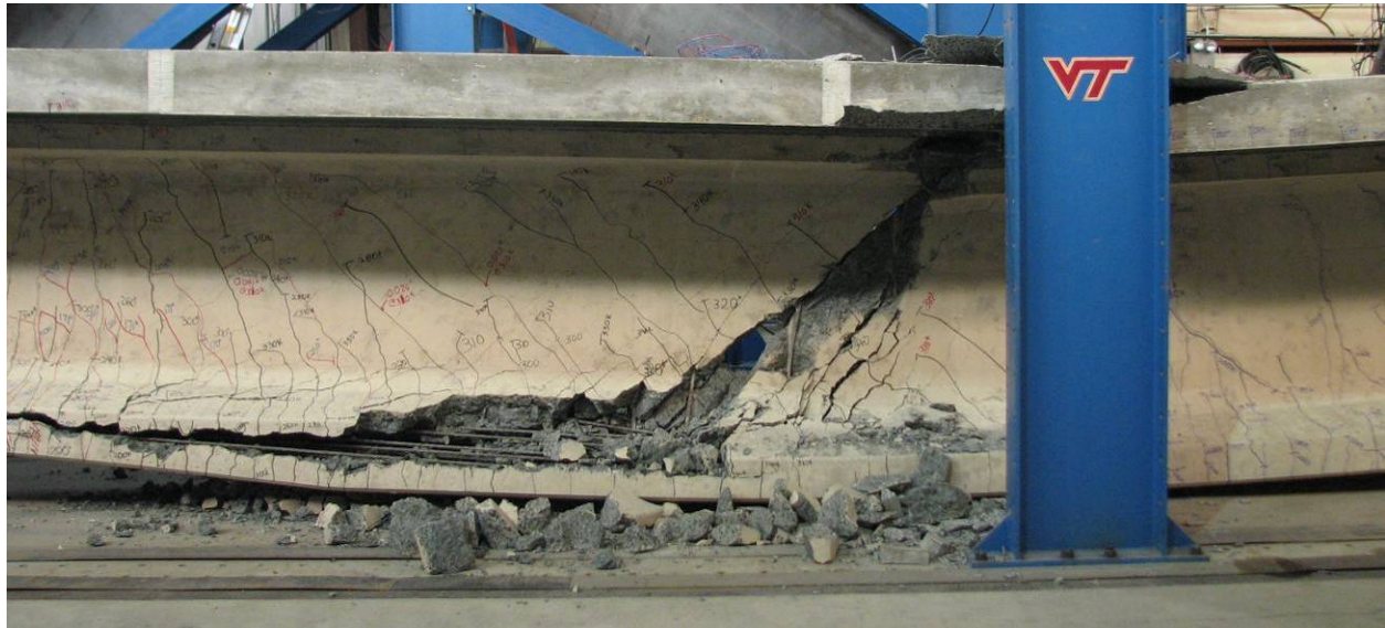
Figure 55. Ultimate failure of the PCBT-53
