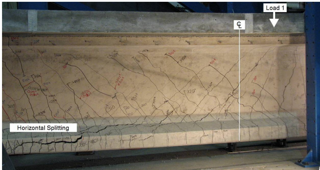
Figure 51. Horizontal bottom flange splitting failure
