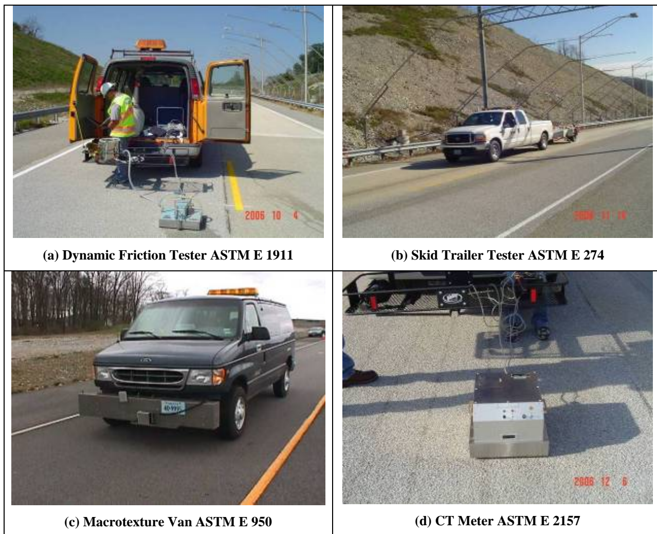
Figure 8. Friction and Macrotexture Measuring Devices Used
