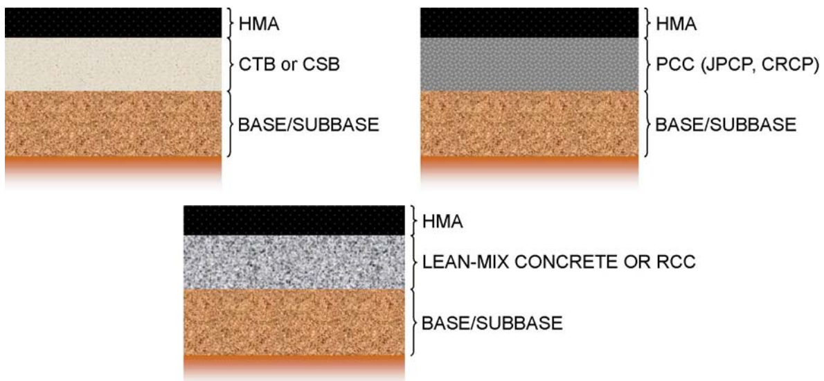
Figure 1. Typical Cross-sections of Composite Pavements
