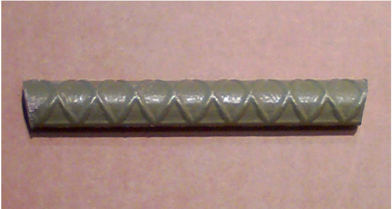
Figure A1. Glossy Green Rebar – 1
