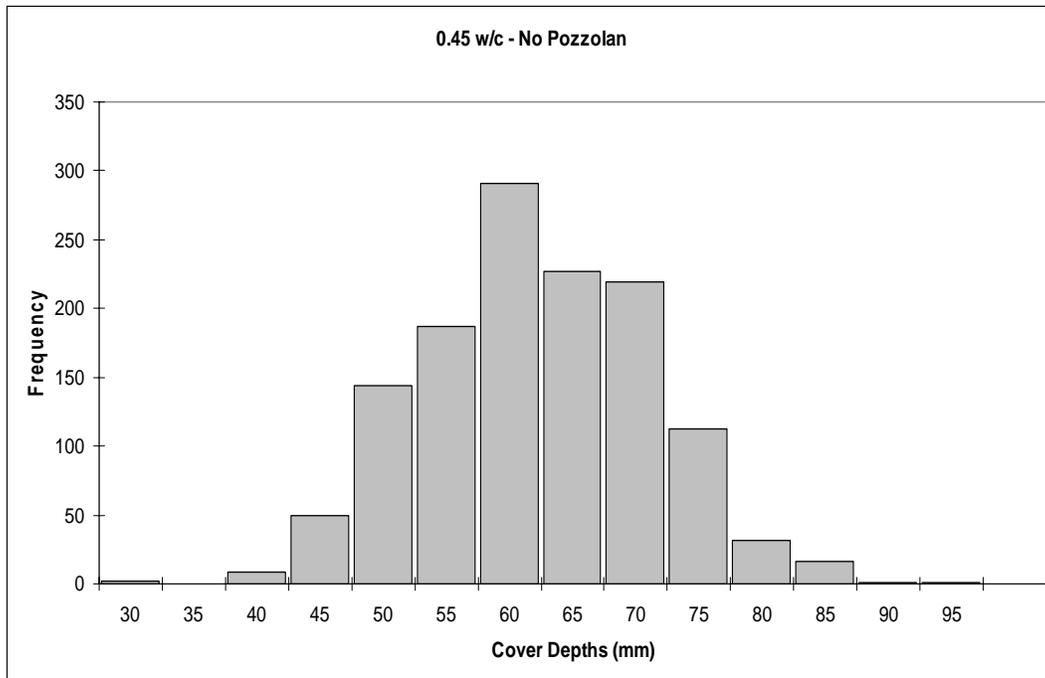
**Figure 15. Cover Depth Measurements – 0.45 w/c**
