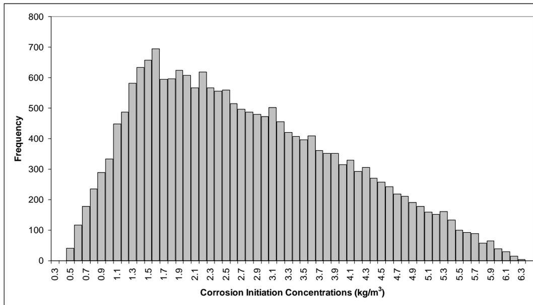
**Figure 9. Corrosion Initiation Concentrations (Bare Steel - Randomly Generated)**
