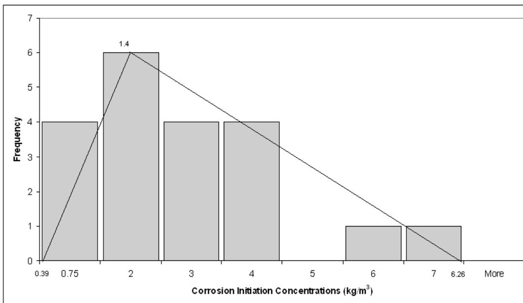
Figure 8. Corrosion Initiation Concentrations – Bare Steel
