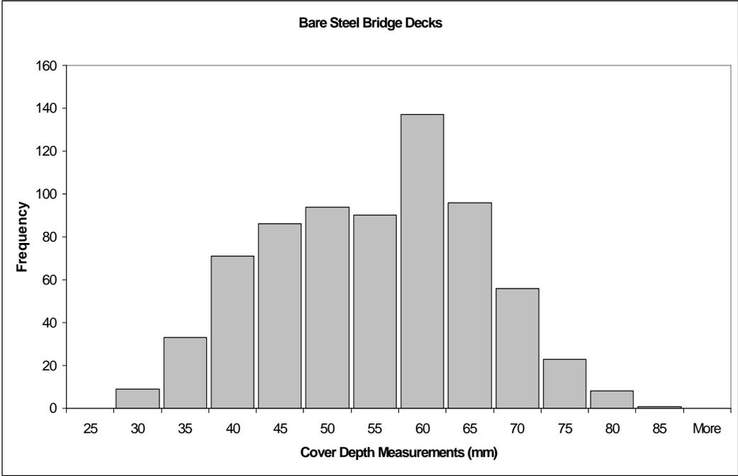
**Figure 13. Cover Depth Measurements –  $0.47 w/c$**
