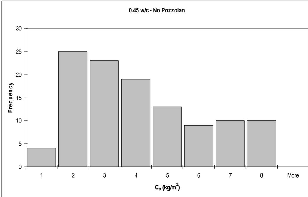
**Figure 14. Surface Chloride Concentrations – 0.45 w/c**
