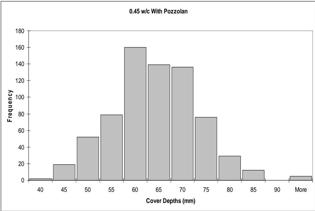
**Figure 18. Cover Depth Measurements – 0.45 w/c**
