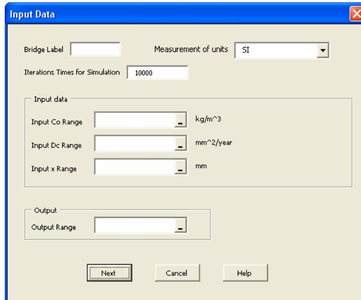
**Figure 4. BCA Chloride Threshold Input Form**
