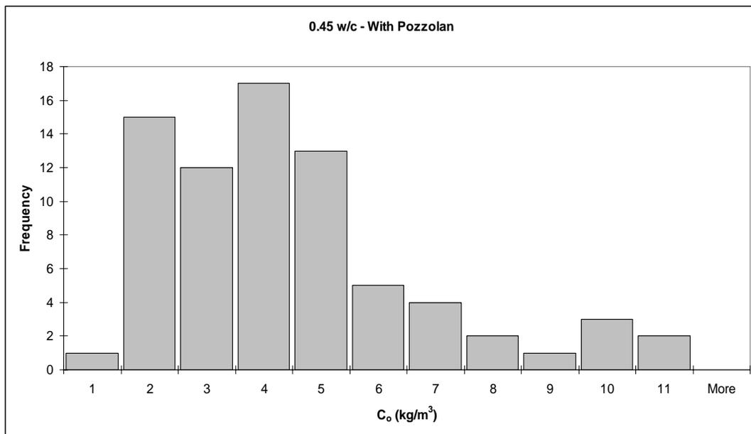
**Figure 17. Surface Chloride Concentrations – 0.45 w/cm**
