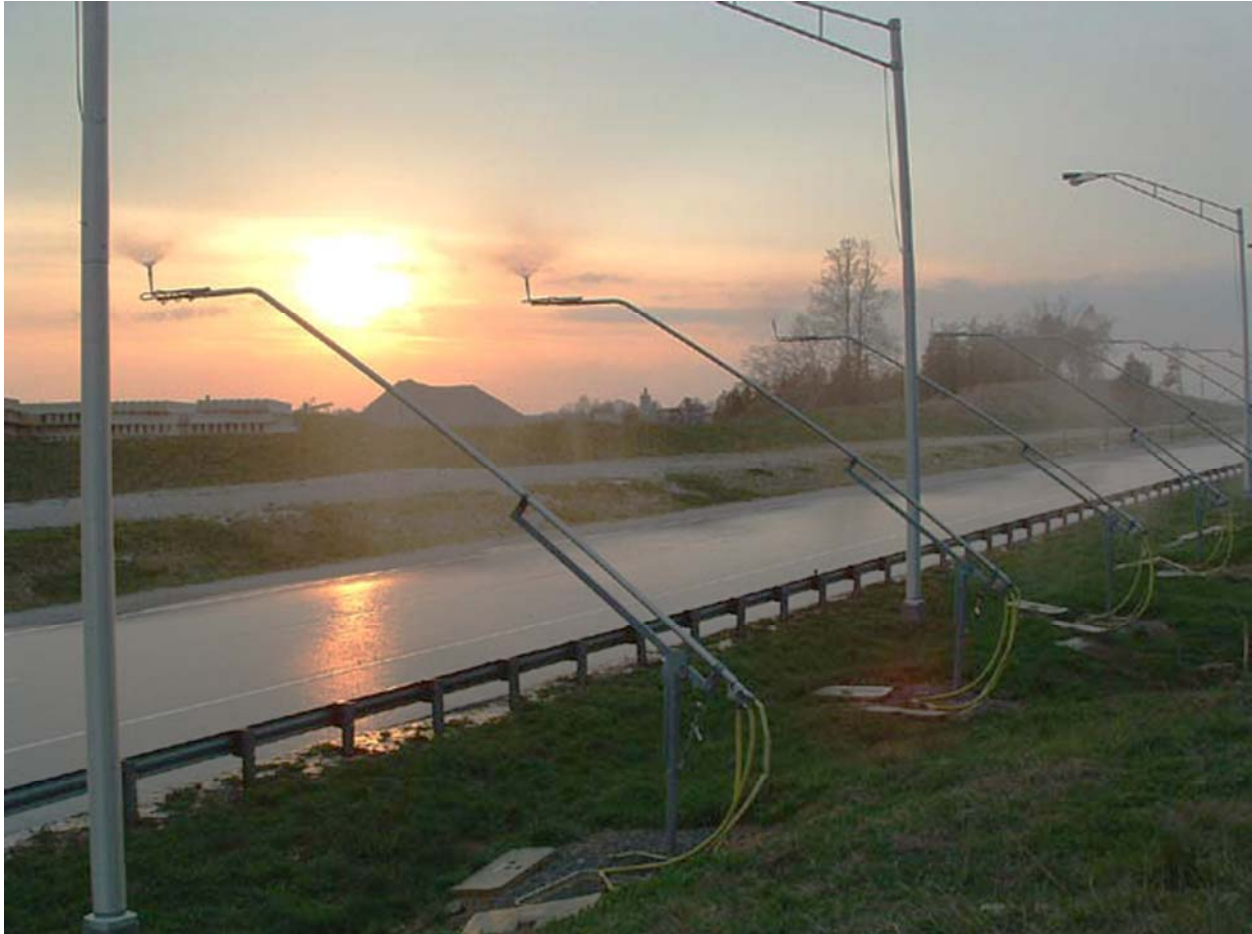
Figure 4. Smart Road All-Weather Testing System
