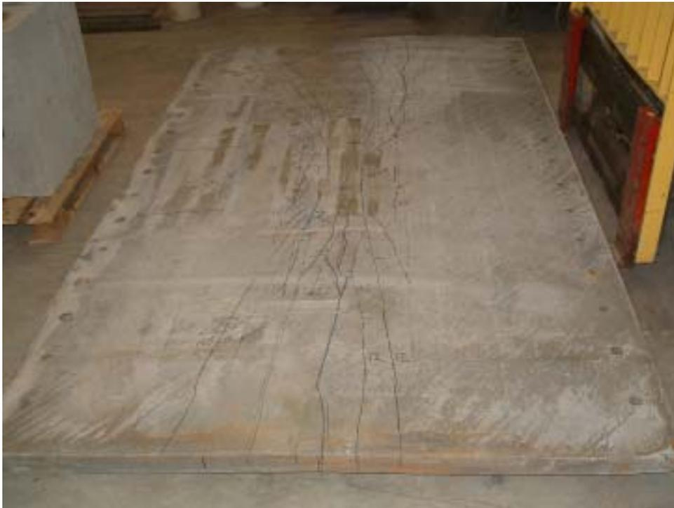
**Figure 27. Typical Cracking Pattern on Bottom Surface of Large Plate Specimens.**
