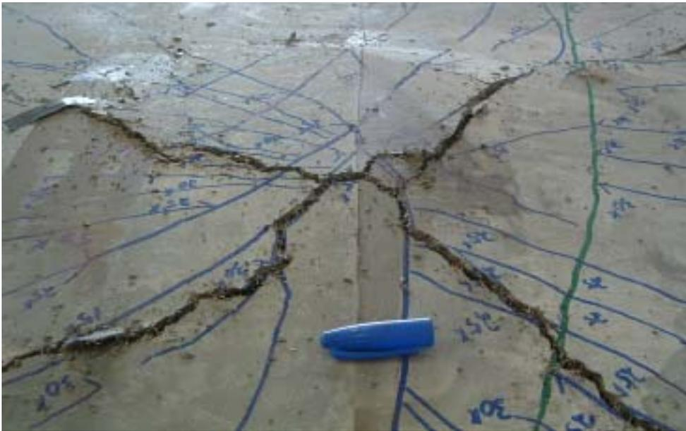
**Figure 25. Crack Patterns on Tension Faces of Specimens with Flexural Failures**
