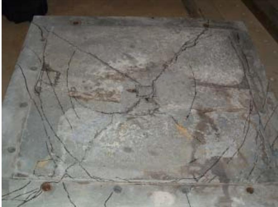
**Figure 26. Cracking Pattern on Loaded Face of Specimens with Flexural Failures**
