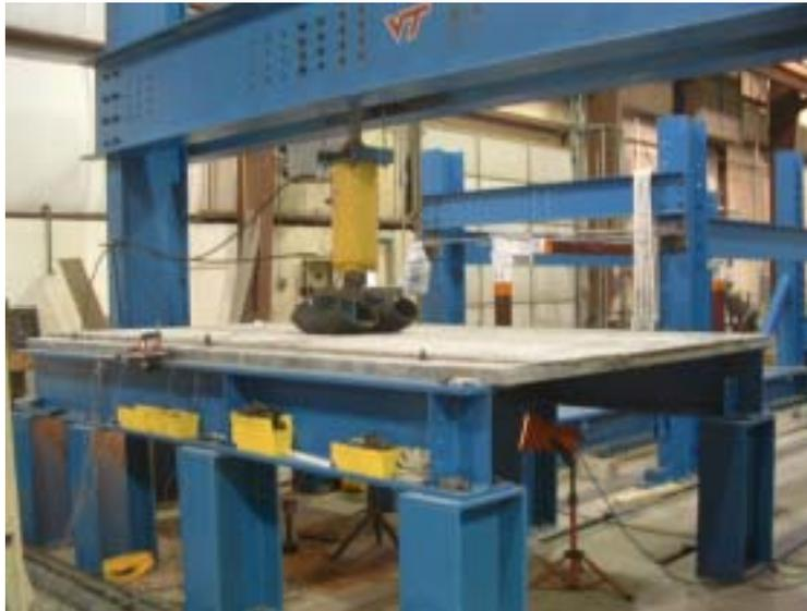
**Figure 21. Tire Patch Used to Load Large Slabs.**
