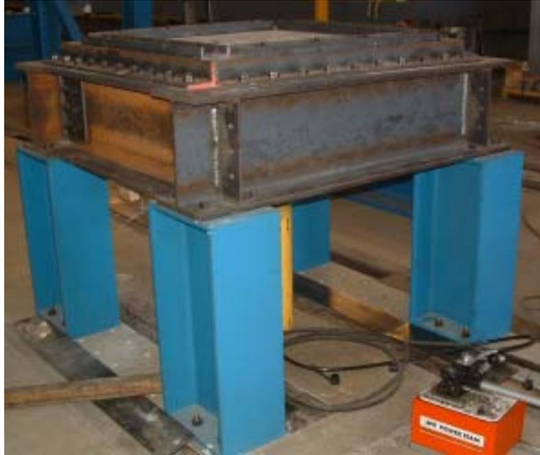
Figure 15. Frame for Small Slab Tests
