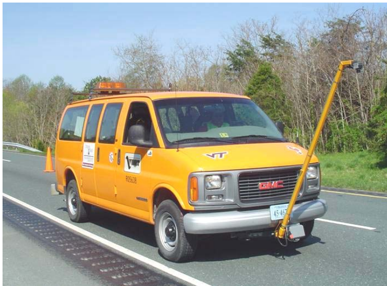
Figure 2. Deployment of the digital camera used for the video survey
