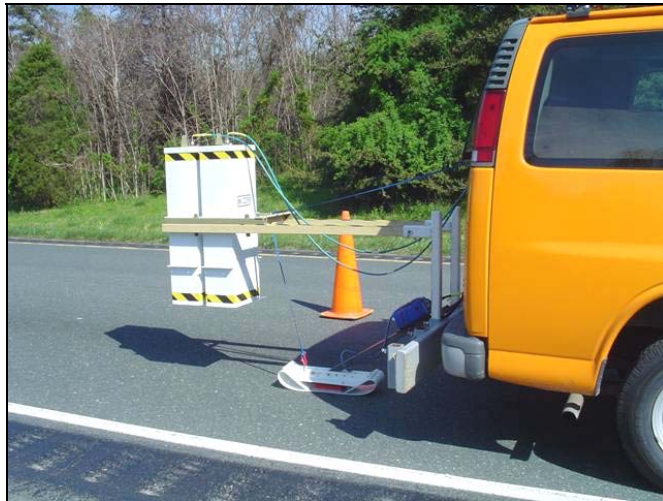
Figure 1. Van used for GPR data collection
