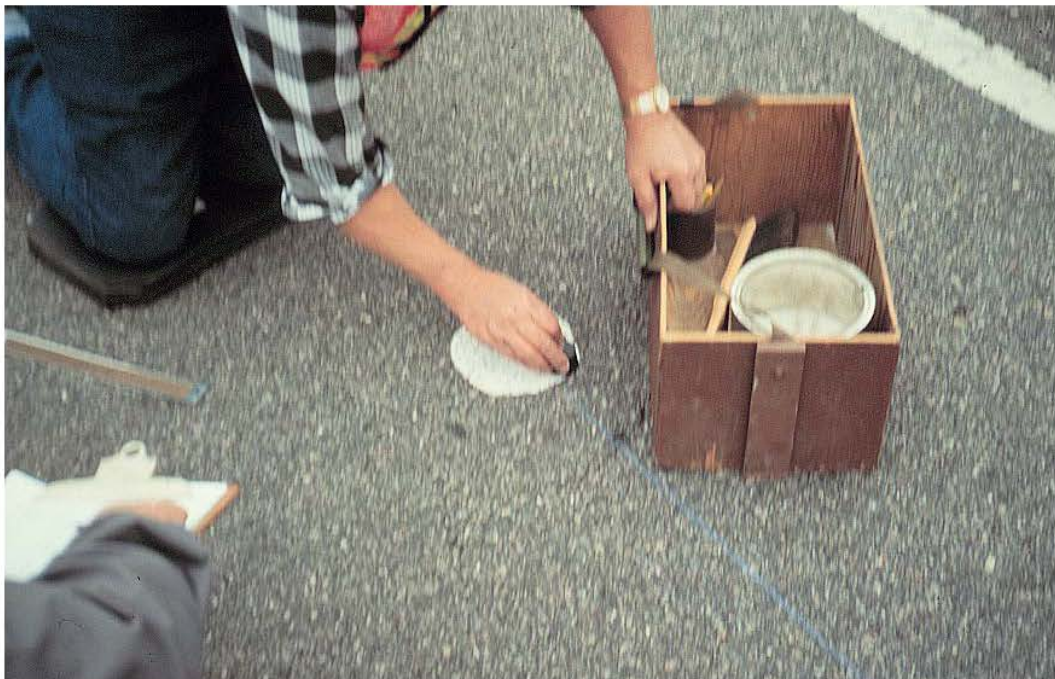
Figure 1. Volumetric Method (Sand Patch Test) (ASTM E965)
