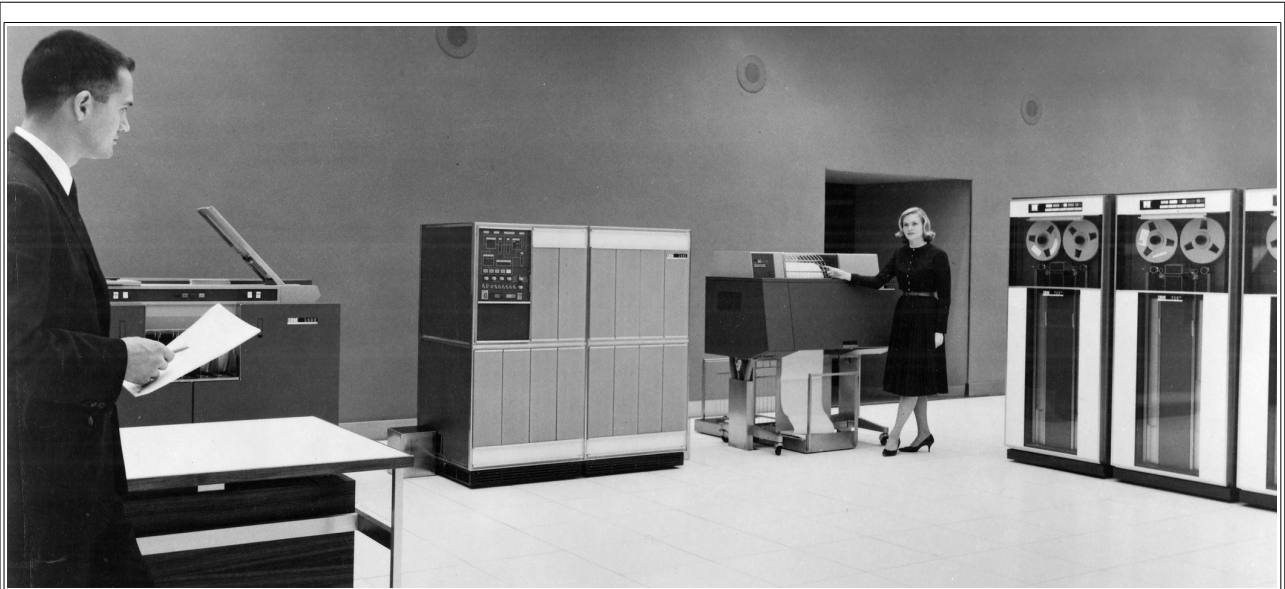
Figure 7: The IBM 1401 System (Optical Character Reader not shown here). From left to right, the punch card reader/writer, mainframe, printer, and magnetic tape units. The IBM 1401 Demo Lab and Restoration Project Computer History Museum, "IBM 1401 Archive Pics," Internet: http://ibm-1401.info/IBM1401_ArchivePics.html , Date Accessed: 2014. Used under fair use, 2014.
