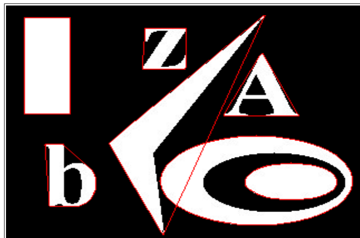
Figure 15: Red outlines represent convex hulls of the white regions. Aforge.NET, "Blobs Processing," Internet: http://www.aforgenet.com/framework/features/blobs_processing.html , Date Accessed: 2013. Used under fair use, 2014.
