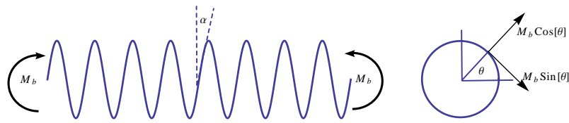
FIGURE 5.2: Pure bending of a spring in its axial plane
