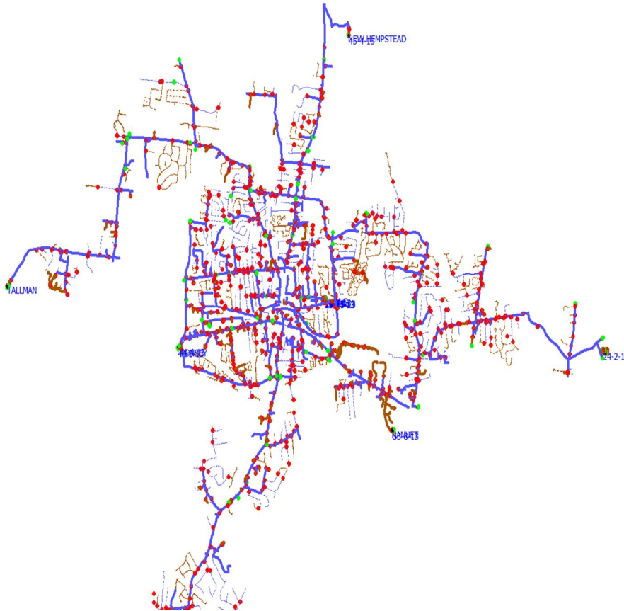
Figure 3-1. Eleven feeder system used in study
