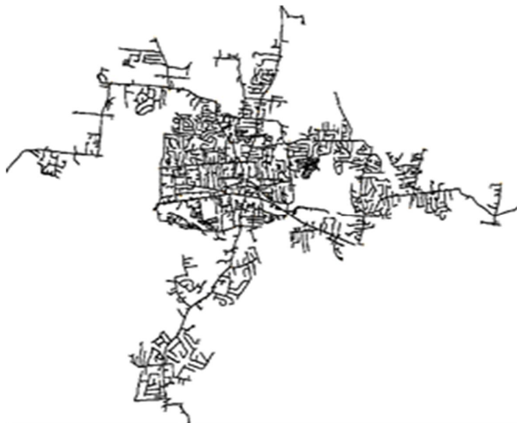
Figure 4-1. Seven substations, fourteen feeder model
