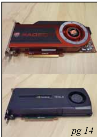
Pictured to the left are NVIDIA and AMD brand GPU accelerator cards. These cards would normally be installed in each compute node of the small cluster testbed featured on the cover.
