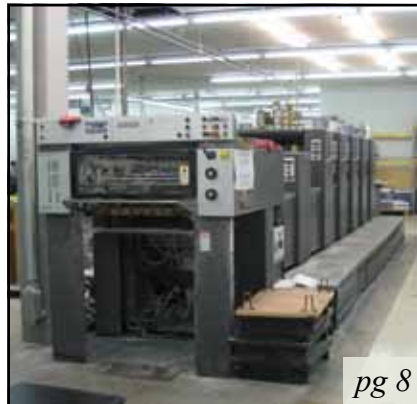
The Heidelberg Speedmaster 74 five-color press, which has a tower dedicated to each of the CMYK (cyan, magenta, yellow, and black) colors and an extra tower for a spot color when necessary.
