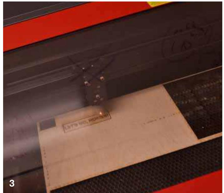
1. An example of the well-defined cuts that the laser cutter in the workshop is able to perform on plastic. This device can be used to cut, engrave, and print on materials other than simple paper.
