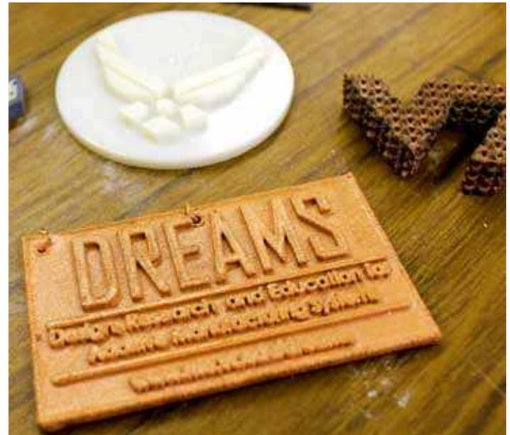
Here are a few of the artifacts created in the DREAMS Lab. Notice how unique and complex the internal and external geometries are. Without additive manufacturing technologies, it would be very difficult to form these products.
