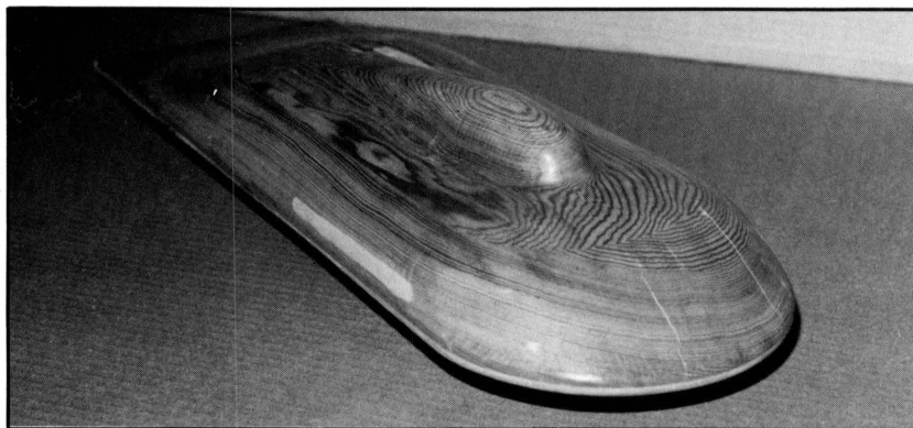
A wooden mock-up of the VT Solaray, designed by volunteer mechanical and electrical engineering students.
