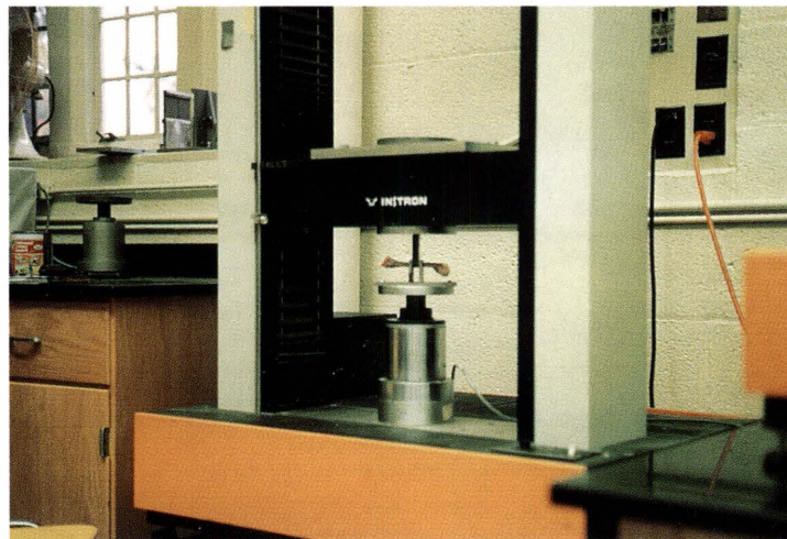
The chicken bones were tested for shear strength by an Instron testing machine. (Photos this page courtesy of Dr. James Wilson.)
