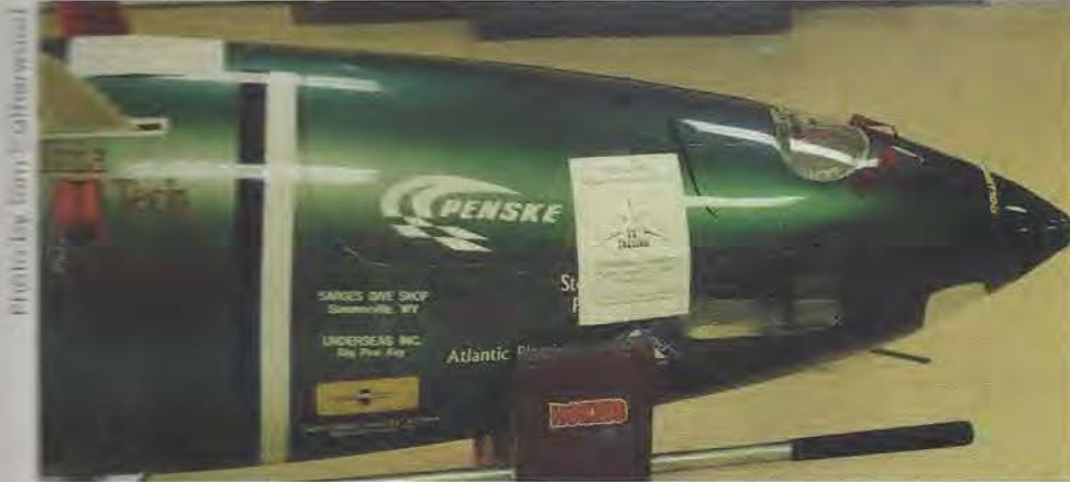
The streamlined sub's pointed snout draws design cues from the Great White Shark
