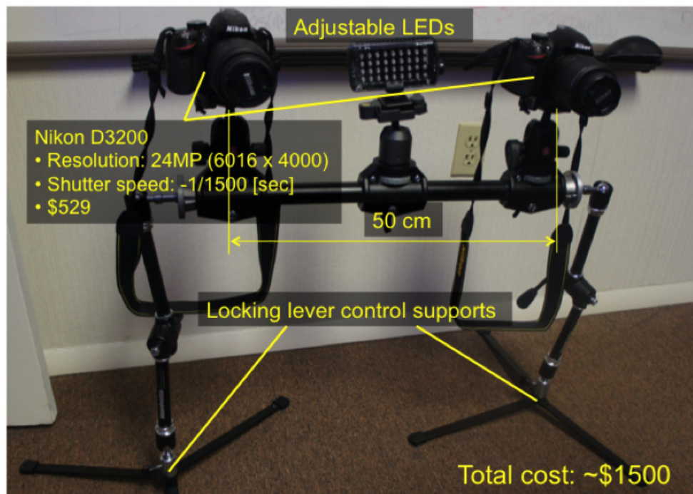
Figure 7.4: Hardware system for parallel DCT full-field measurement
