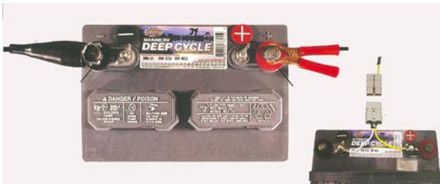
**Battery with special terminals with charger connections (left) and the connection for the light system (lower right).**
