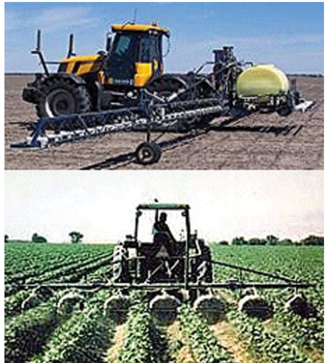
Figure 10. Sensor-based WeedSeeker for herbicide control www.ntechindustries.com/rowcrop.html .
