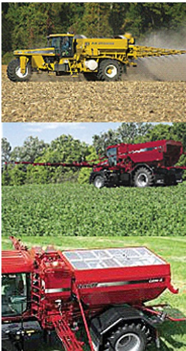
Figure 14. Pneumatic spreaders for applying dry chemicals (lime, nutrients), and the hop conveyor can be driven for VRA.
