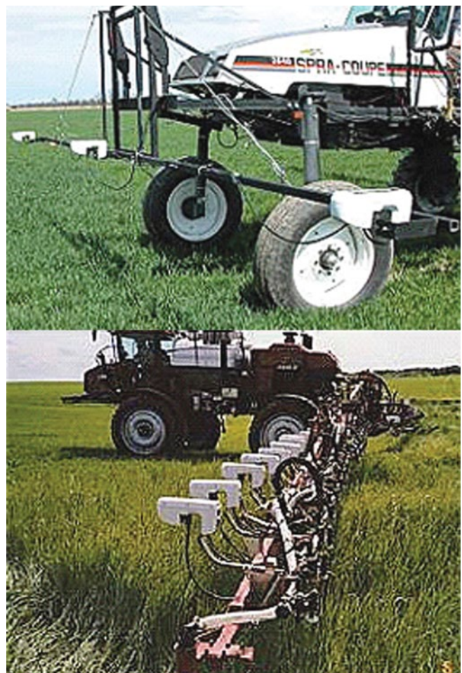
Figure 16. Optical sensor measuring Normalized Difference Vegetation Index (NDVI; GreenSeeker) and adjusting VRA nitrogen on wheat.
