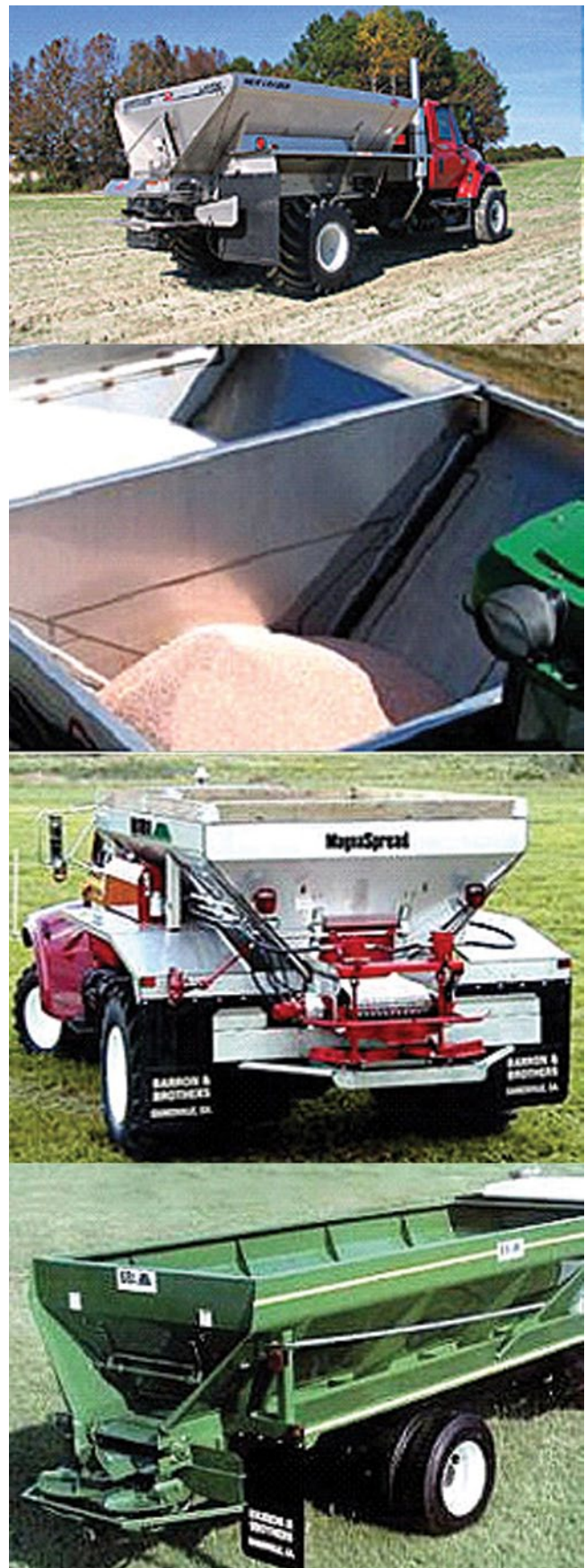
Figure 13. Spreaders for applying dry chemicals (lime, nutrients), and the hop conveyor can be driven for VRA.
