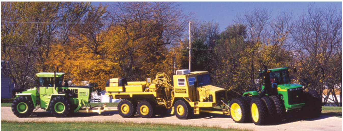
Figure 2. The lead tractor is being tested on the track during drawbar-performance tests. The two vehicles in tow are load units.
