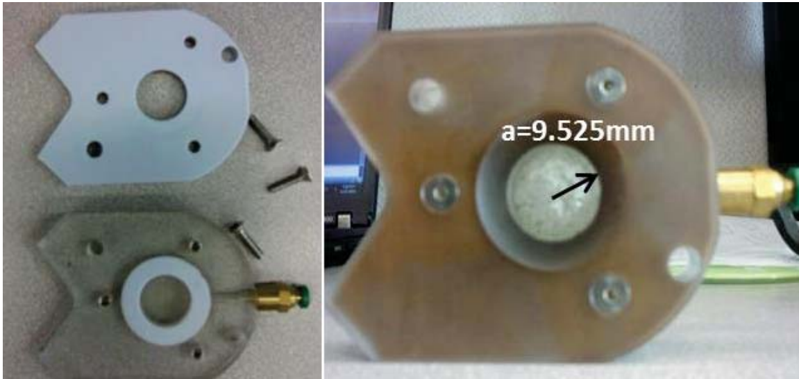
Figure 4.1. Fixture used for biaxial strength measurements, shown at left disassembled, and at right assembled with a pressurized blister.
