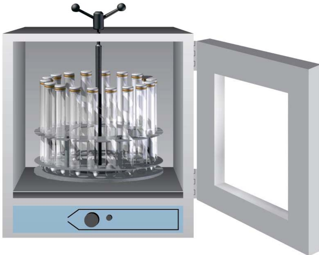
Figure 2.6. Schematic of in-house long term creep fixture.
