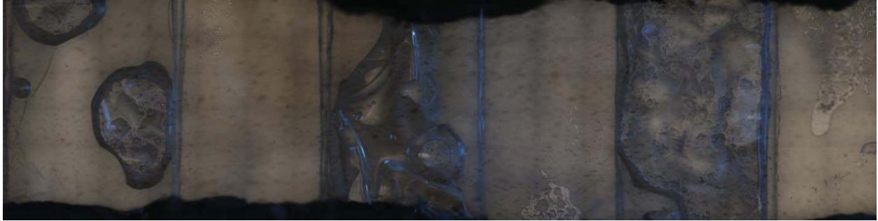
Figure 5.21. Images of membrane constrained in glass bipolar plate after 5 days immersed in DI water across multiple lands and channels.
