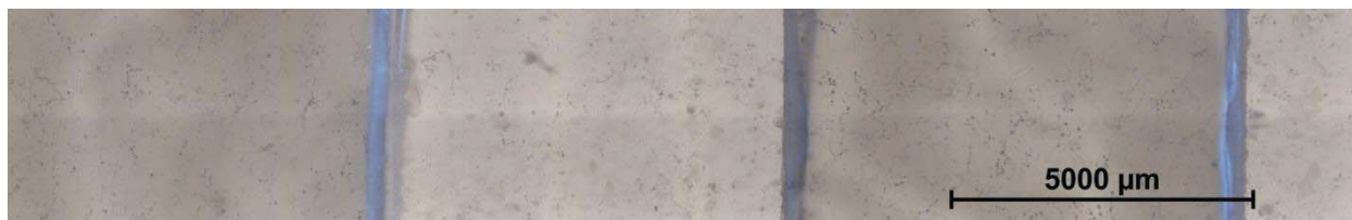
Figure 5.19. Large image scan of membrane in glass bipolar plate fixture after assembly, prior to immersion.
