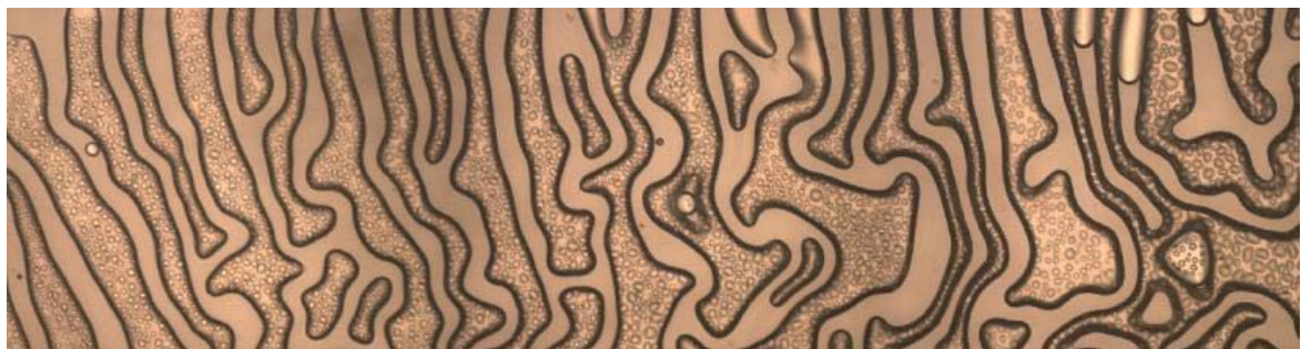
Figure 5.17. Buckling pattern of 3.17 mm wide PFCB/PVDF-HFP constrained primarily uniaxially between two glass slides held with binder clips after immersion in liquid water.
