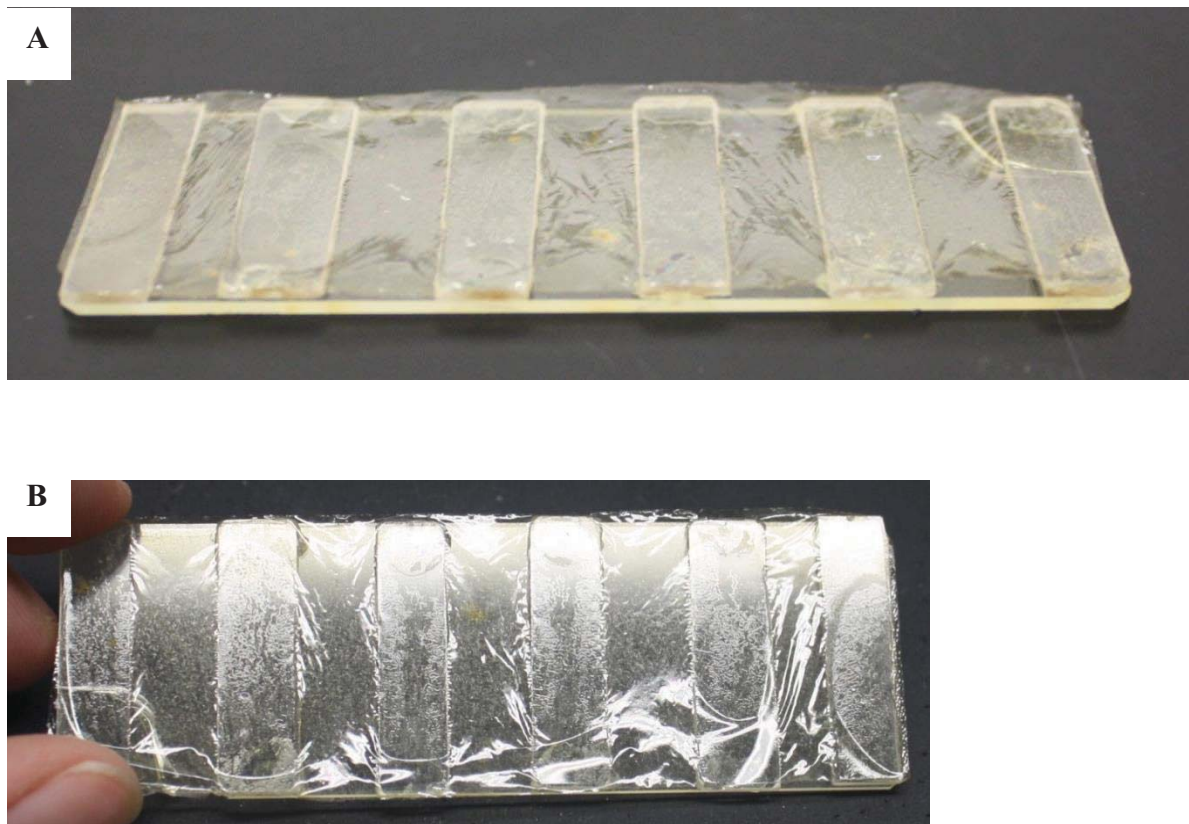
Figure 5.23. Images of membrane after disassembly of glass bipolar plate fixture using the Canon DSLR camera to highlight the wrinkles formed due to tensioning of the membrane during dry-out.
