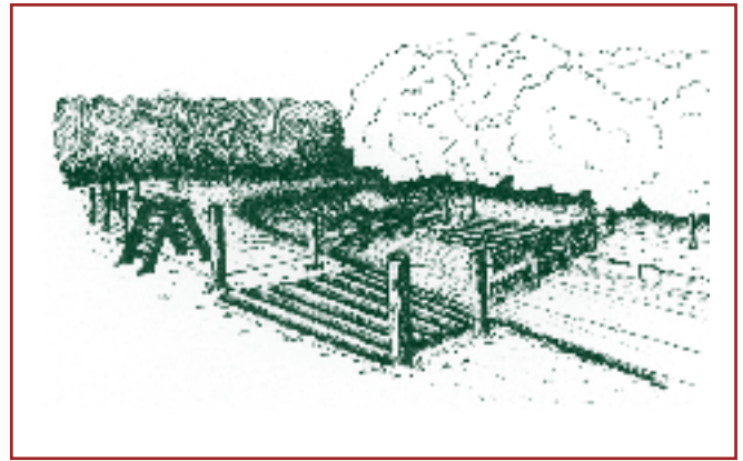
Fence livestock watering and crossing sites to restrict up-stream or downstream animal movements. Carefully select sites with a firm bottom and gentle slopes.
