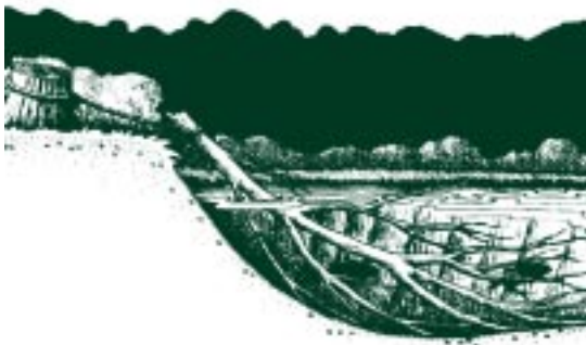
Example of a submerged tree top to provide cover.
