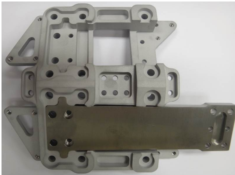
Figure 5-1: Configurable compliant spring interface for the shin with and without a compliant beam
