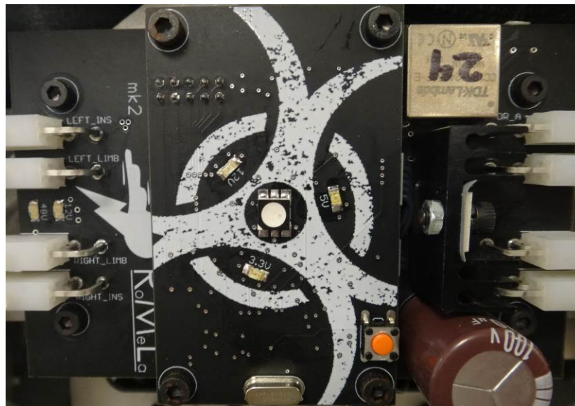
Figure A-9: Power distribution board on the upper body
