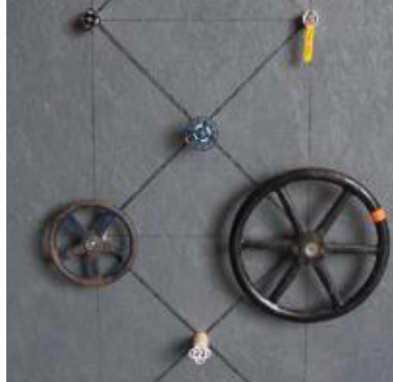
Figure 3-6: Example valves including large wheels, 90° turn levers, and hand knobs. Image used with permission from DARPA, http://www.darpa.mil/NewsEvents/Usage.aspx , 2013.
