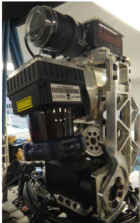
Figure 6-6: THOR head with spinning LIDAR and camera
