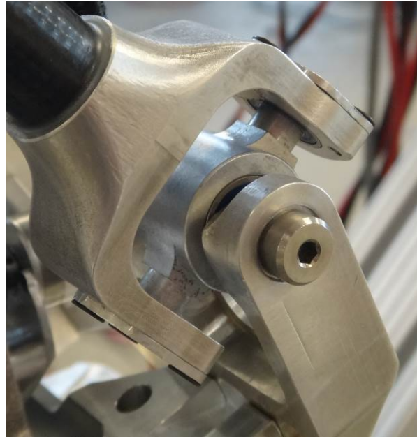
Figure 4-9: Universal joint attaching to the foot
