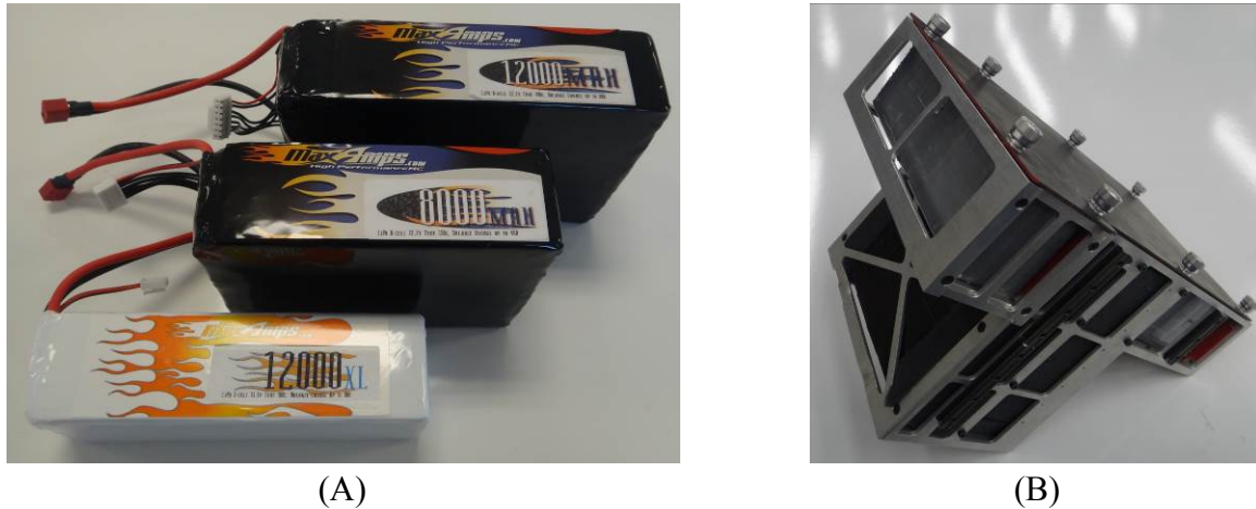
Figure 6-4: Images of the (A) lithium polymer batteries used for THOR and (B) the power core
