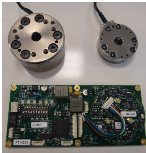
Figure A-3: From the top left: the Mini-58 transducer, the Mini-45 transducer, and the sensor interface board
