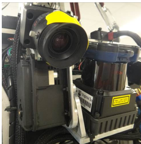
Figure 6-3: Ground mapping sensors on the chest
