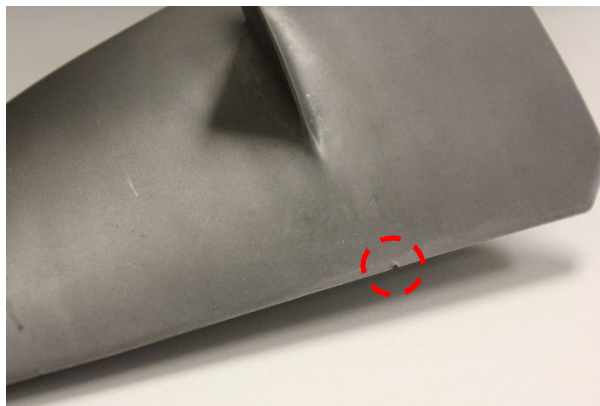
Figure 8. Small notch in a Garrett F109 fan blade caused by impact with foreign object
