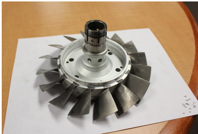
Figure 19. PT6A-28 first stage compressor rotor as received from overhaul shop, Airforce Turbine Service
