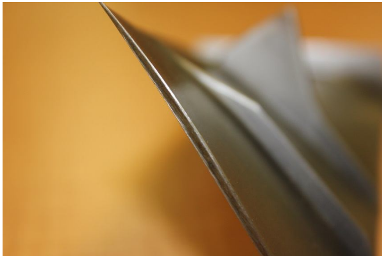
Figure 14. Image of actual used blade tip from the Virginia Tech Turbomachinery and Propulsion Research Laboratory JT15D. Note the bright pressure and suction edges and dark center of the blade tip
