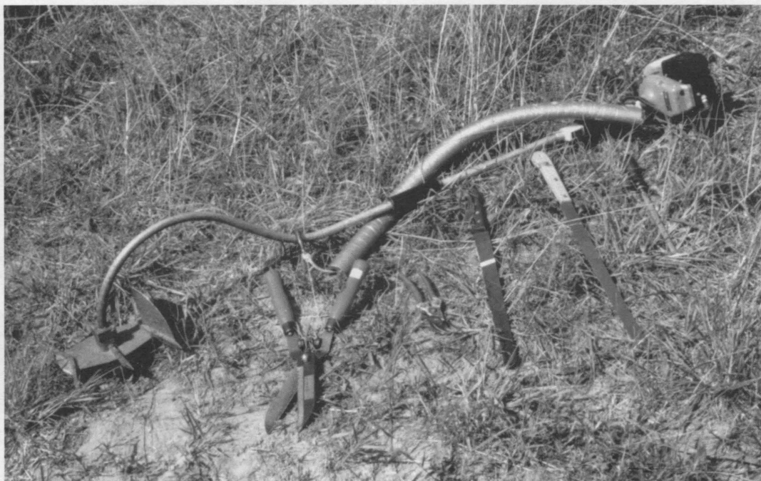
Figure 6. Shearing tools -- (top) hand-held motorized shearer; (bottom, left to right) hedge clipper, hand pruner, two shearing knives, and a sharpening steel.
