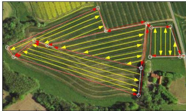
Figure 3: Computer generated solution to field path planning(Sørensen, Bak, and Jørgensen 2004)
