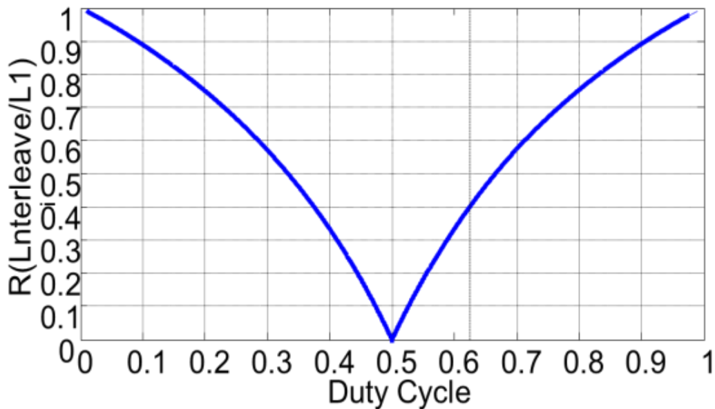
Figure 3-4 Current ripple reduction ratio of two phase interleaving topology
