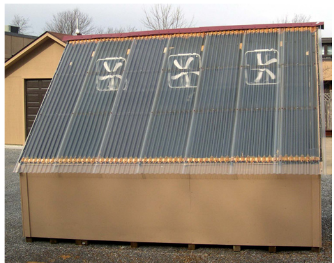
Figure 5. Front view of kiln showing fan placement.
