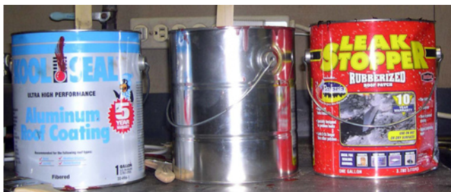
Figure 3. Coatings that can be used to seal the inside of the kiln and to coat the ends of sample boards. From left to right: Aluminum roof coating, a commercial kiln coating, and rubberized roofing sealer.
