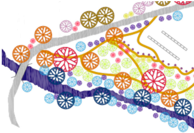
Figure 1. A clip of a riparian food forest design that uses mature crown widths drawn to scale to determine tree spacing.
