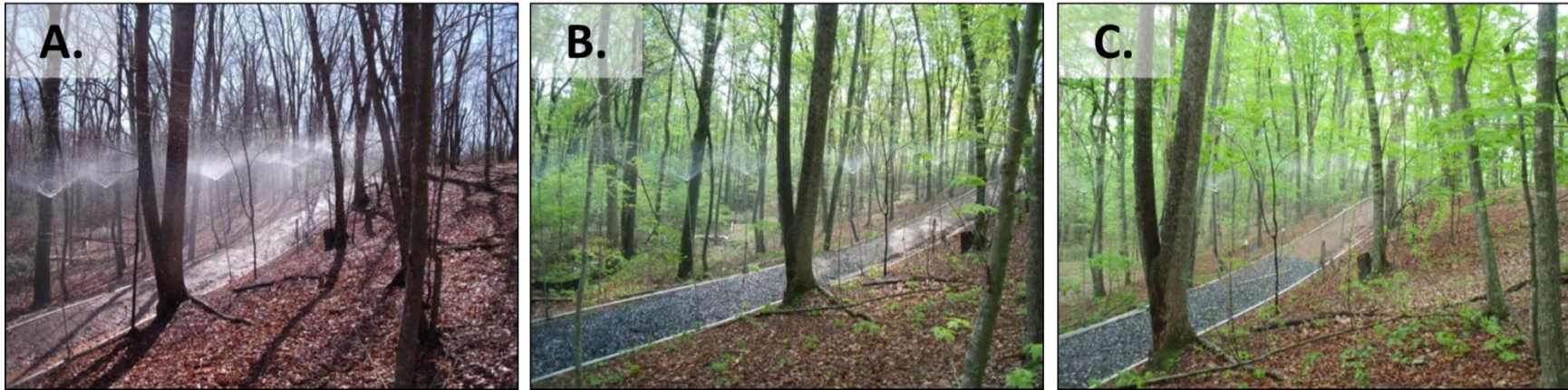
Figure 5.3. Photographs depicting rainfall simulation experiments for the succession of gravel surfacing treatments at Site 5: A.) No Gravel; B.) Low Gravel; C.) High Gravel. Surface cover for the rainfall simulation experiments at Site 5 was 14, 47, and 63%, respectively, for the No Gravel, Low Gravel, and High Gravel treatments.
