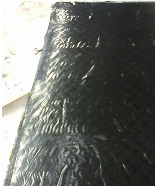
Figure 21: Wet layup resulted in resin remaining on the surface of the panel, potentially reducing the overall strength.
