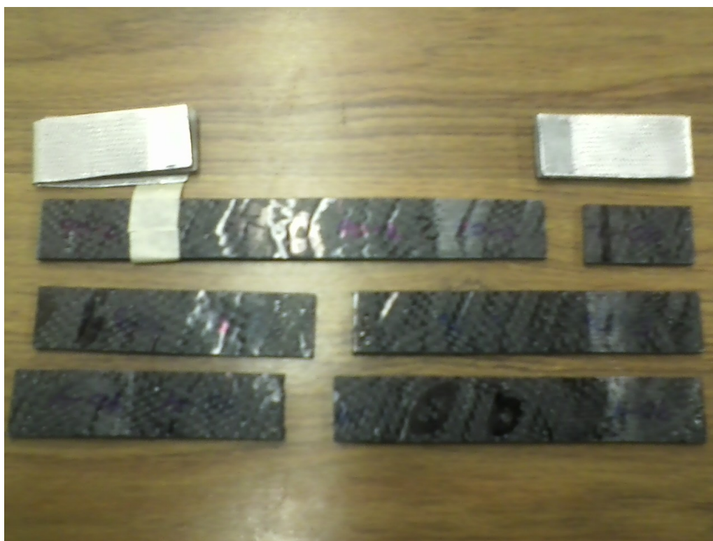
Figure 23: Ninety-degree specimens post failure: break is lateral as expected
