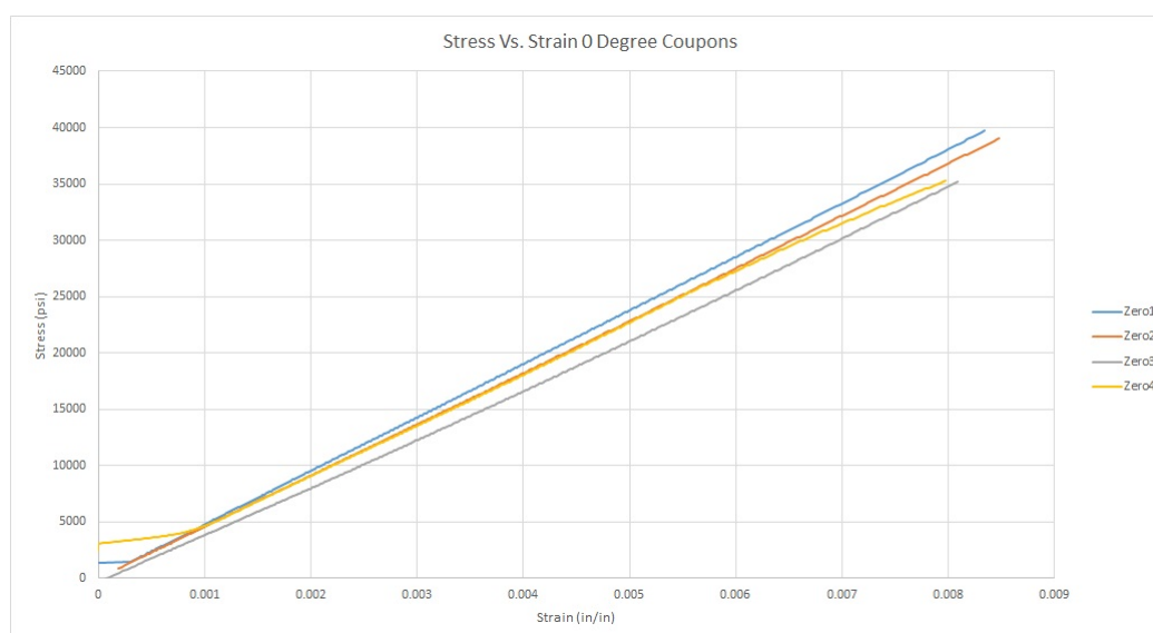
Figure 25: A nominal stress vs. nominal strain graph as measured by the strain gages for the zero-degree test coupons.
