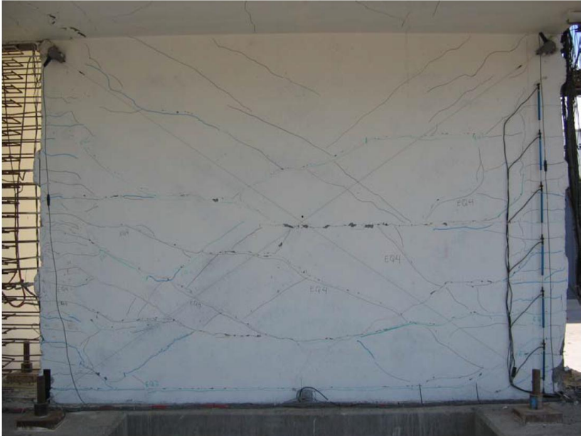
Figure 5.23: Crack Pattern on 1 st level of Seven-story Reinforced Concrete Specimen after Final Loading. Panagiotou, M., Restrepo, J., and Conte, J. (2007), “Shake Table Test of a 7-story Full Scale Reinforced Concrete Structural Wall Building Slice Phase I: Rectangular Wall Section” Report No. SSRP-07-07, San Diego, CA. Used under fair use, 2014.
