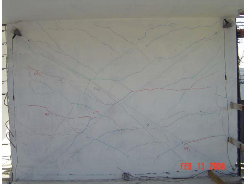
Figure 5.24: Crack Pattern on 2nd level of Seven-story Reinforced Concrete Specimen after Final Loading. Panagiotou, M., Restrepo, J., and Conte, J. (2007), “Shake Table Test of a 7-story Full Scale Reinforced Concrete Structural Wall Building Slice Phase I: Rectangular Wall Section” Report No. SSRP-07-07, San Diego, CA. Used under fair use, 2014.
