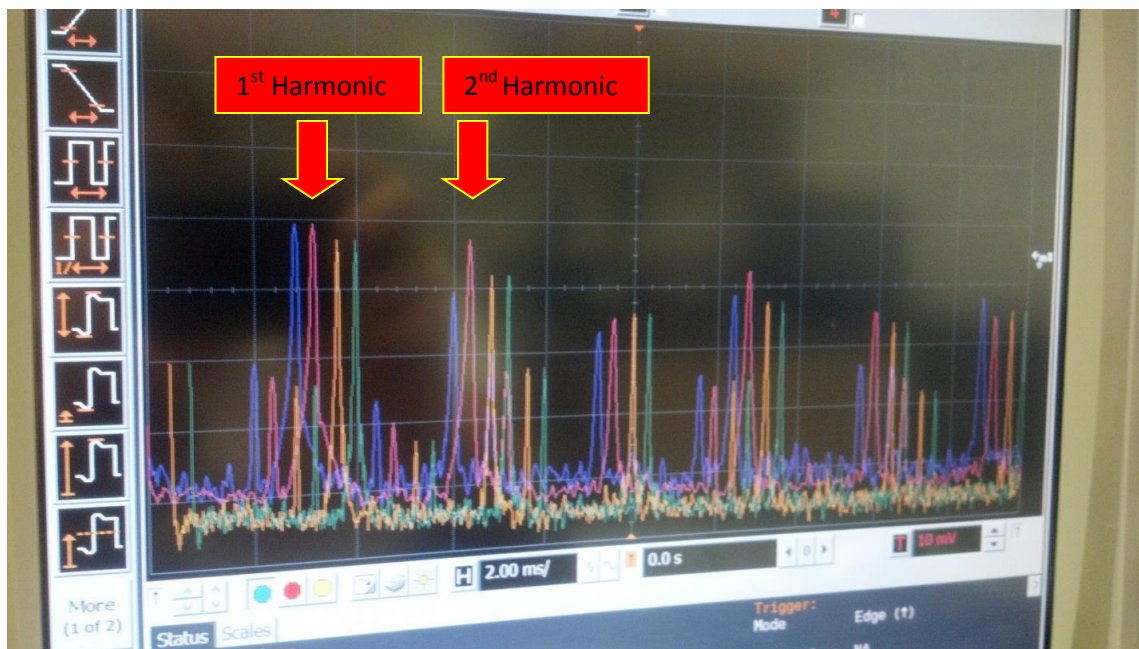
Figure 2-6 Second harmonic detection, red is 0% C 2 H 2 , orange and green are 10% C 2 H 2 , blue is 20% C 2 H 2
