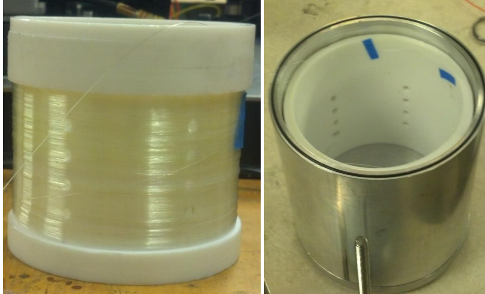
Figure 3-3 (a) Teflon mandrel wrapped with 200 meters fiber before etching. (b) Mandrel inserted into probe housing after etching
