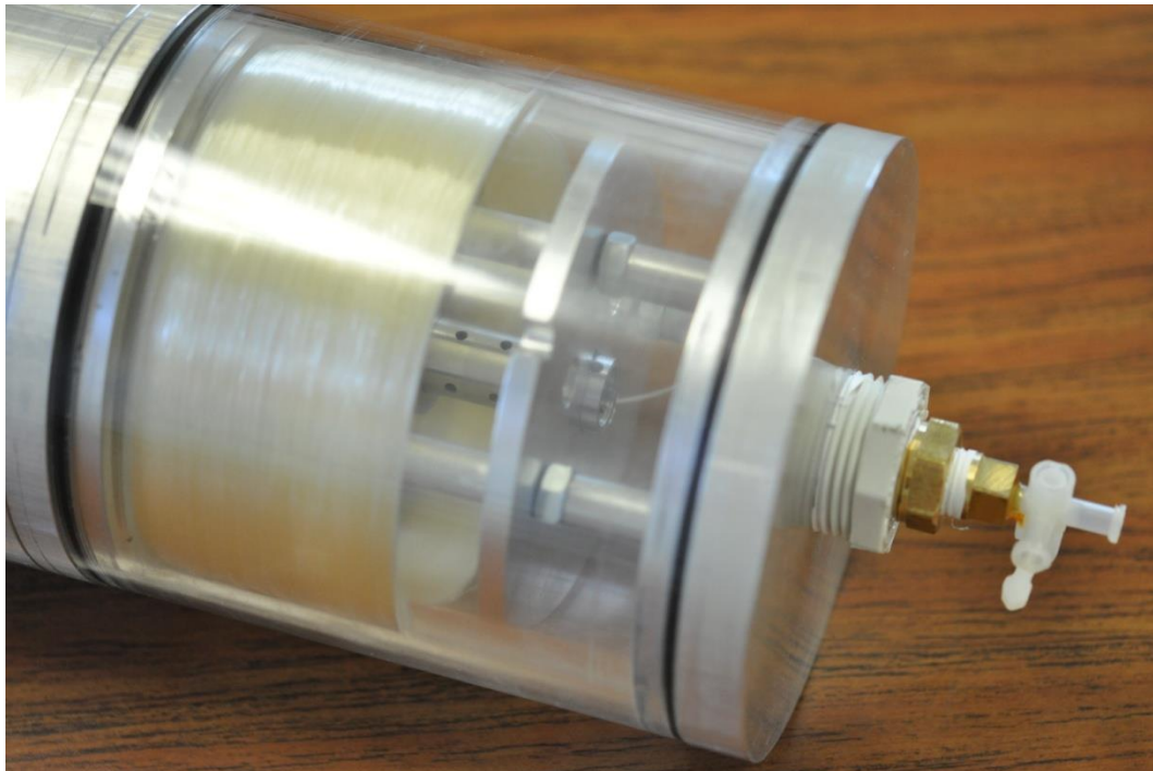
Sensor prototype displaying acetylene sensor probe centered between plates
