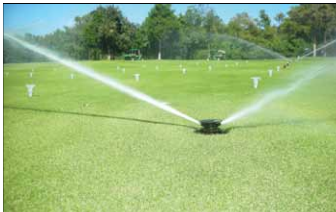
Figure 3-12. Catch can test layout in fairway. Source: EC Design Group, LTD.
