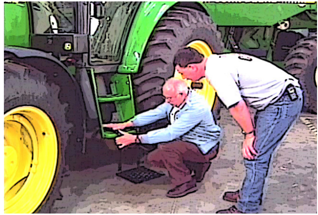
Figure 6. Steps added to improve reach while accessing the work space.
